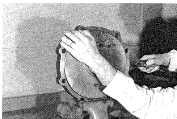
STEP 10. Place piston housing in vise. Start piston from housing by applying compressed air to piston housing pressure port.
