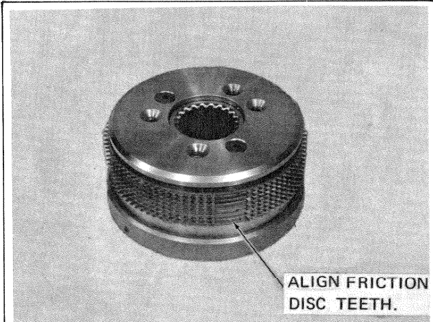
STEP 13. Align friction discs as shown.
