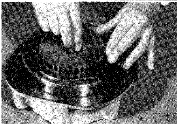
STEP 12. Align the inside teeth of the separator discs and install the hub.
