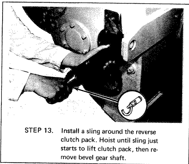
Figure 5-7. Removal And Disassembly Of Bevel Gear Shaft Assembly (Sheet 3 of 3)
