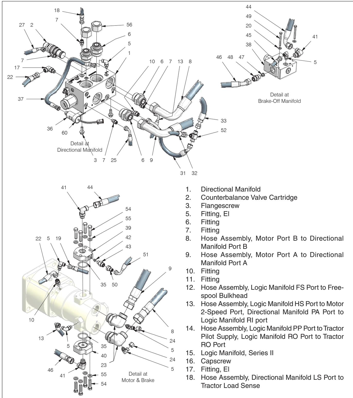
Figure 4-14 Hydraulic System Components, High-Performance\_1
