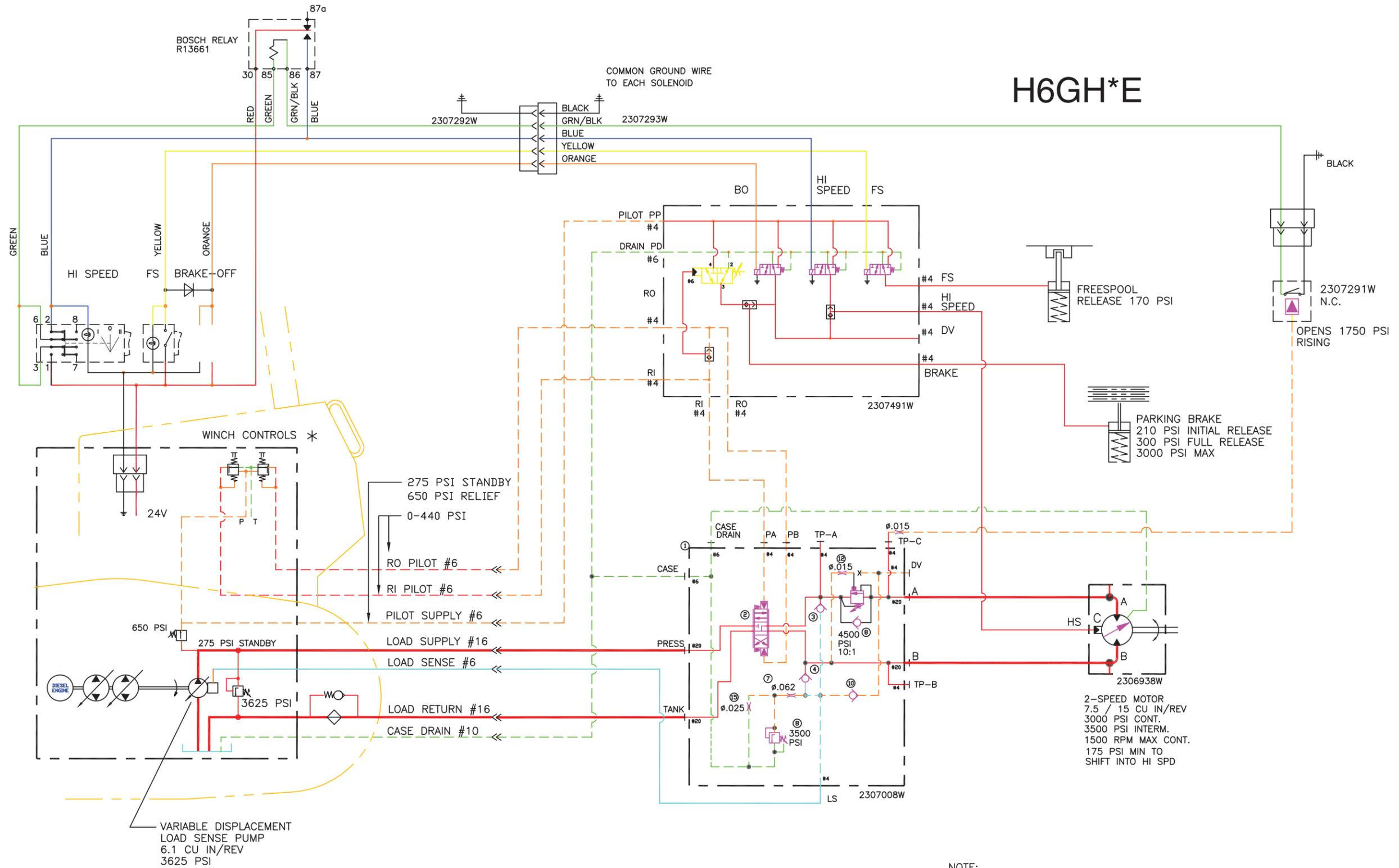
\* NOTE: PILOT OPERATOR ASSY AND PLUMBING TO REAR FACE OF TRACTOR ARE TRACTOR SUPPLIED COMPONENTS ("WINCH READY" OPTION).
