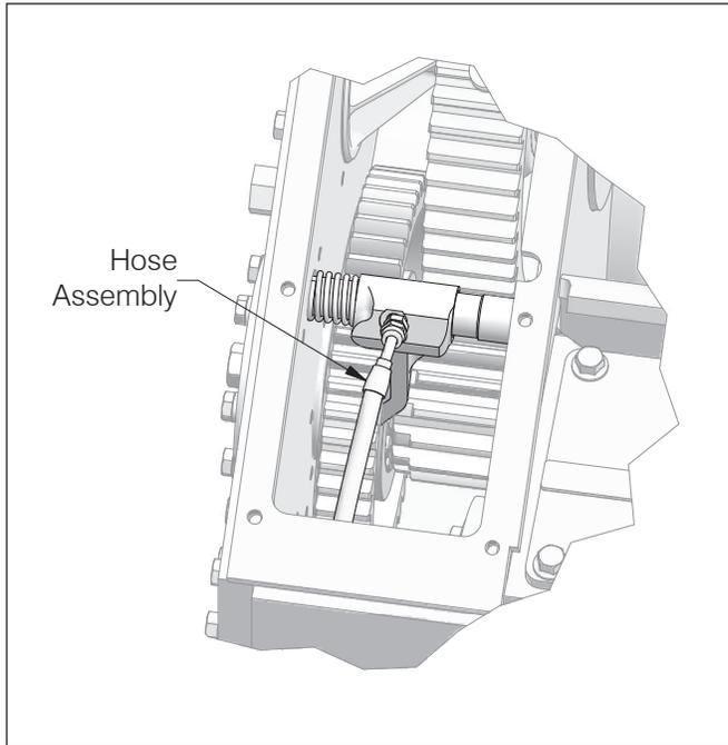
13. Secure the shifter shaft cover and the gasket with capscrews.
