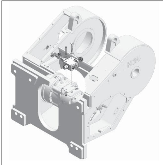
**Hydraulic System Disassembly, High-Performance Winch**
