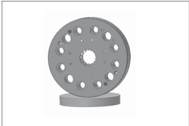
8. Place cartridge on any object which will hold it off the table. Remove screws and timing plate.
