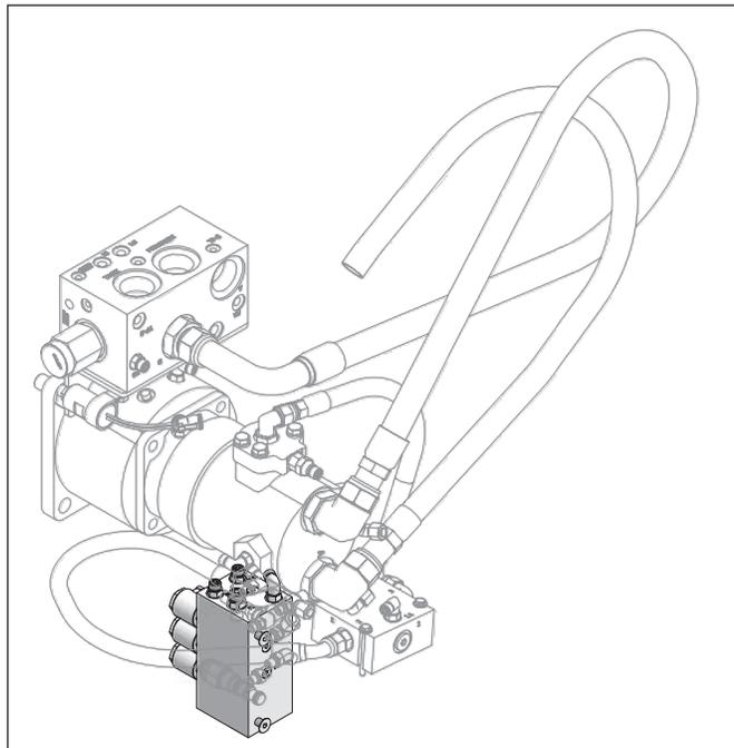
9. Remove the hoses between the high-pressure A and B ports on the motor and the direction manifold assembly.
