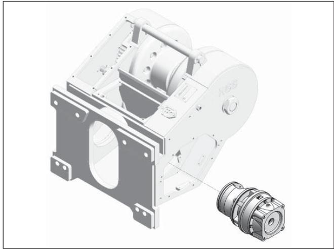
2. Install the reducer mounting, gear retainer, spacer and seal ring in the reducer.
