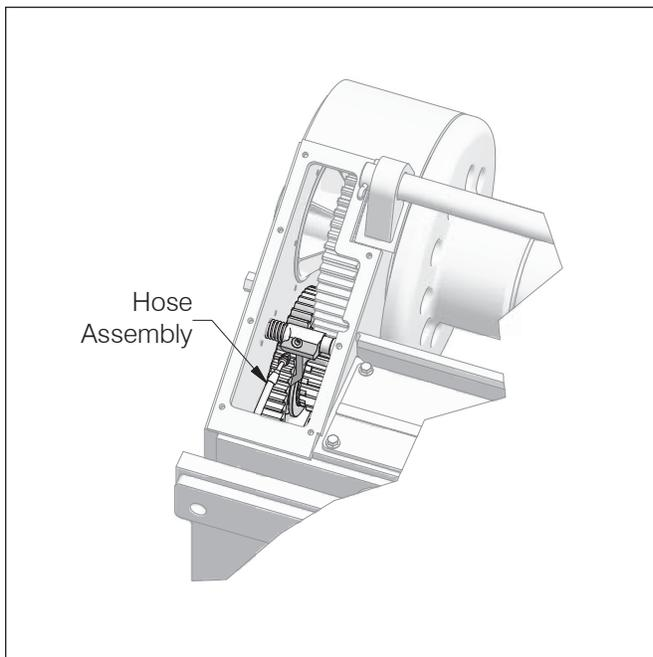
4. Remove the intermediate shaft cover and FREESPOOL piston.
