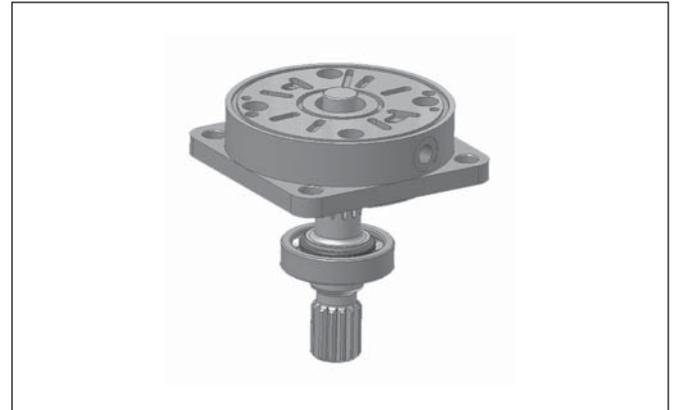
6. Remove snap ring from shaft. Press shaft out of bearing.
