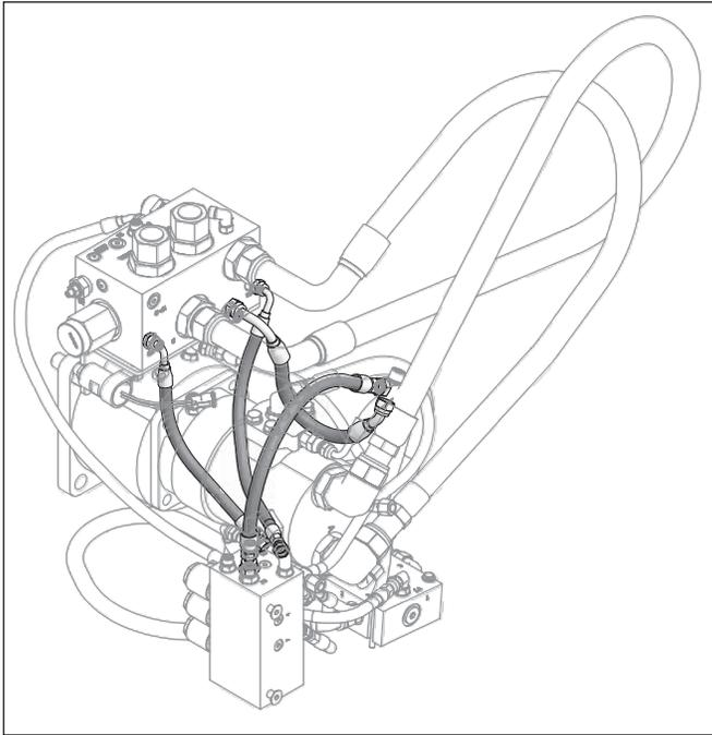
7. Remove the three hoses off the DV port on the logic manifold.
