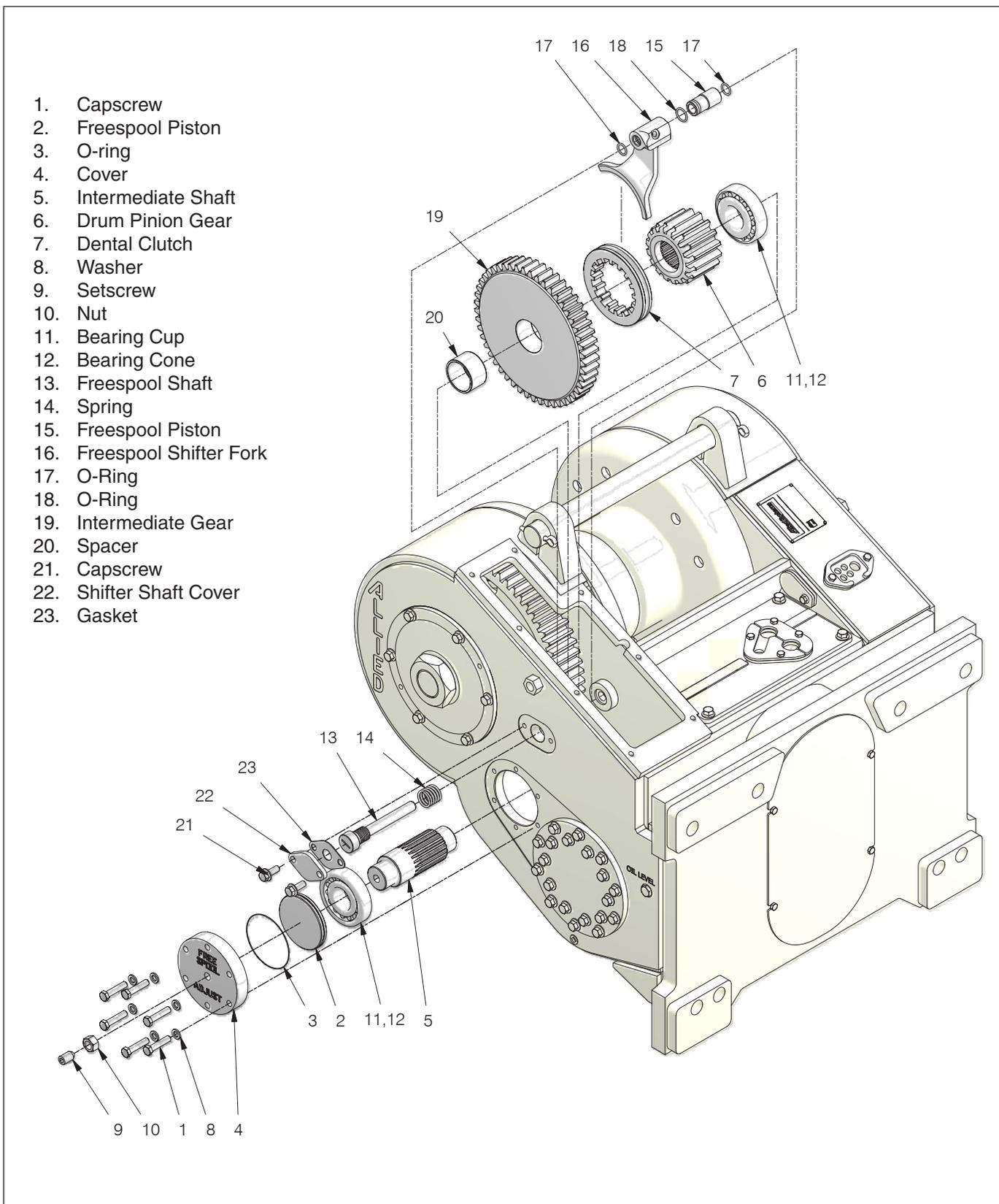
Figure 4-17 Location of Intermediate and Freespool Shaft Components
