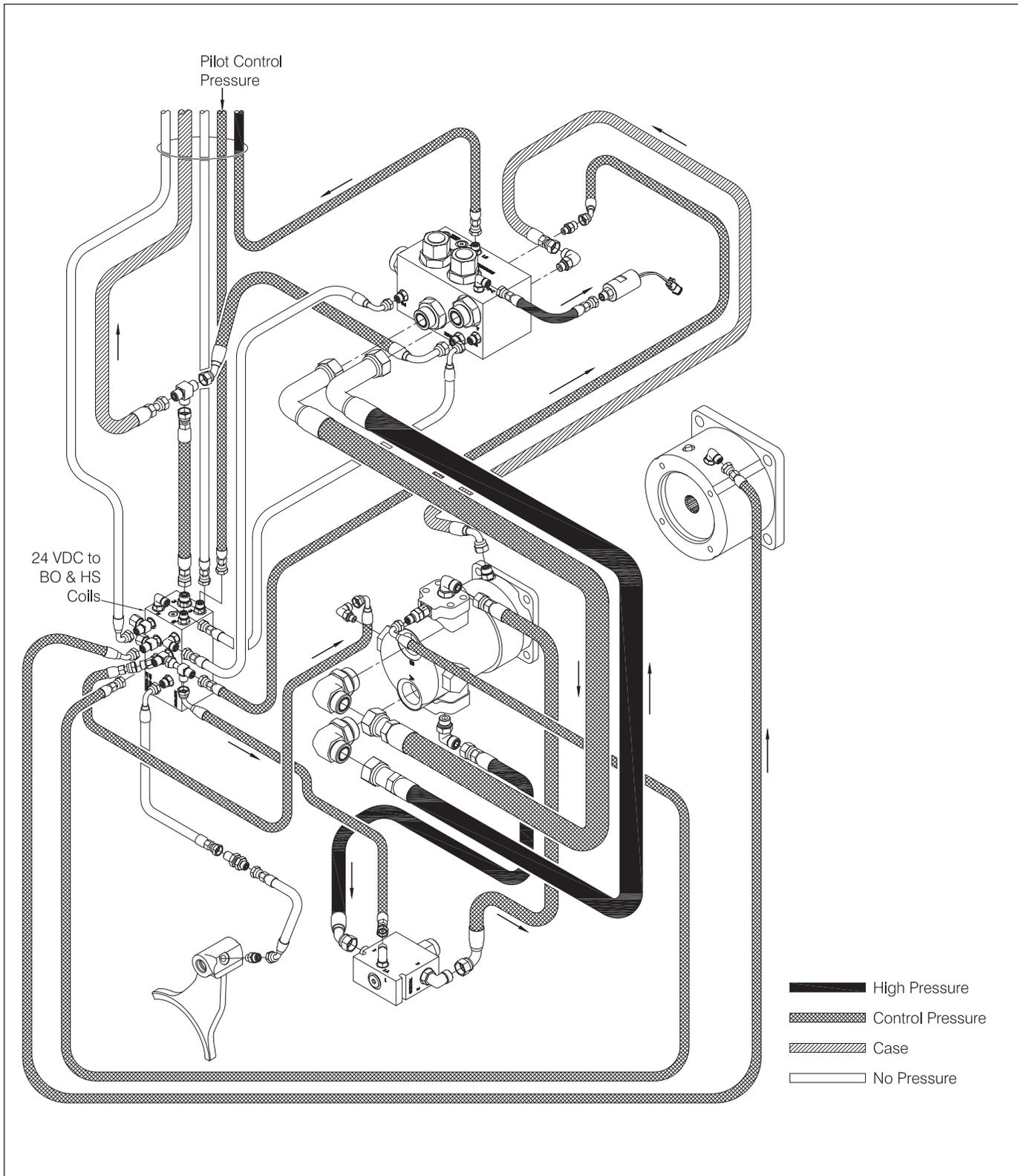
Figure 1-24 Hydraulic System - BRAKE-OFF
