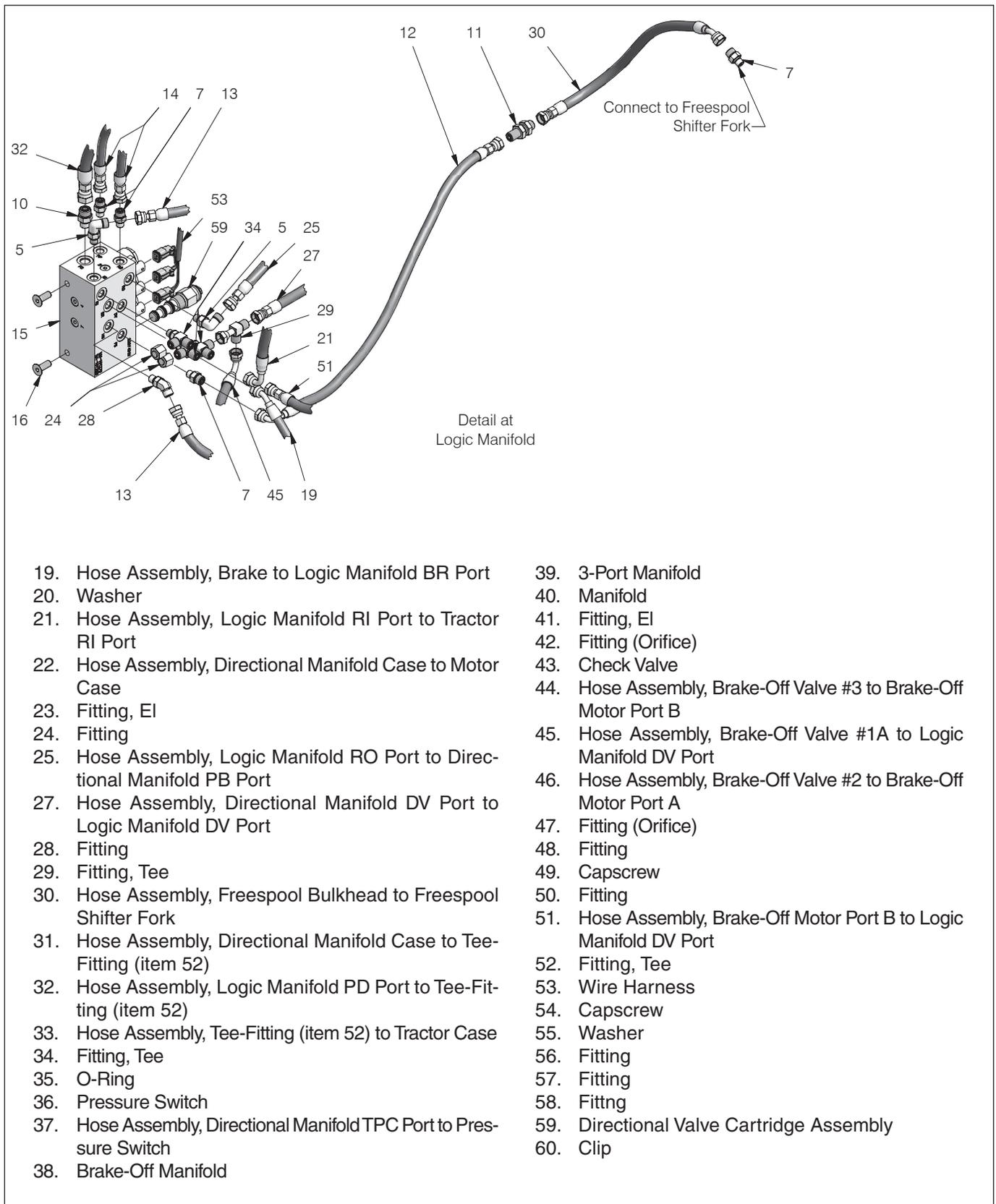
**Figure 4-14 Hydraulic System Components, High-Performance\_2**
