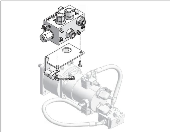
4. Install the hoses between the high-pressure A and B ports on the motor and the directional manifold assembly.
