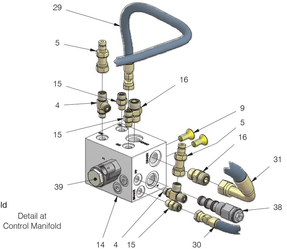
**Figure 4-12 Hydraulic System Components, Rescue Winch\_2**
