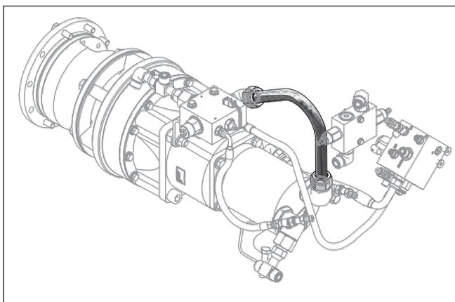
6. Install the hoses at the cross port relief manifold.
