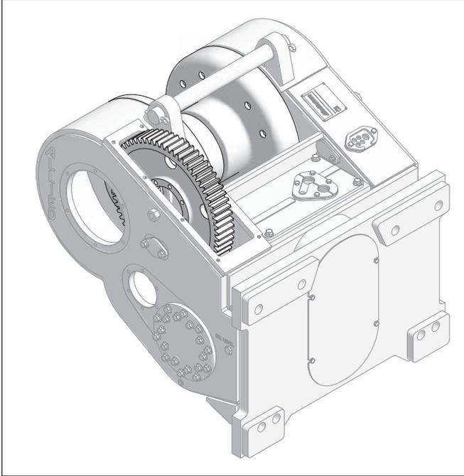
10. Align drum gear with adapter and temporarily secure the drum gear to the adapter, using the retainer plate and two capscrews. This will ensure that the gear will not fall during installation of the shaft.
