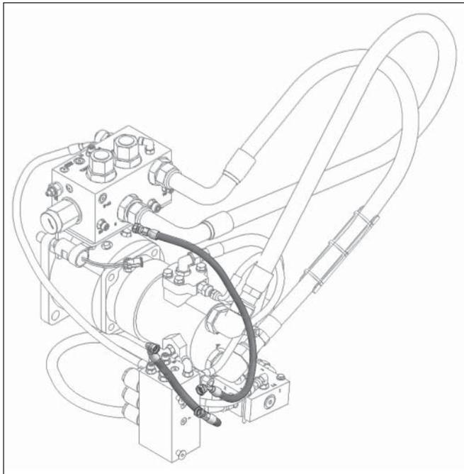
9. Connect the hoses that exit through the frame and the wire harness.
