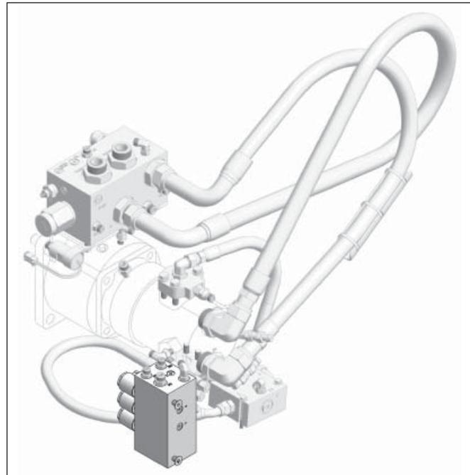
6. Install the hoses to the DV port on the logic manifold.
