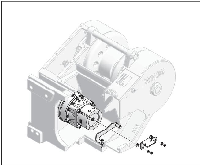
**NOTE: For High-Performance winches, Port A and Port B BRAKE-OFF hoses must be installed before placing motor in winch frame.**
