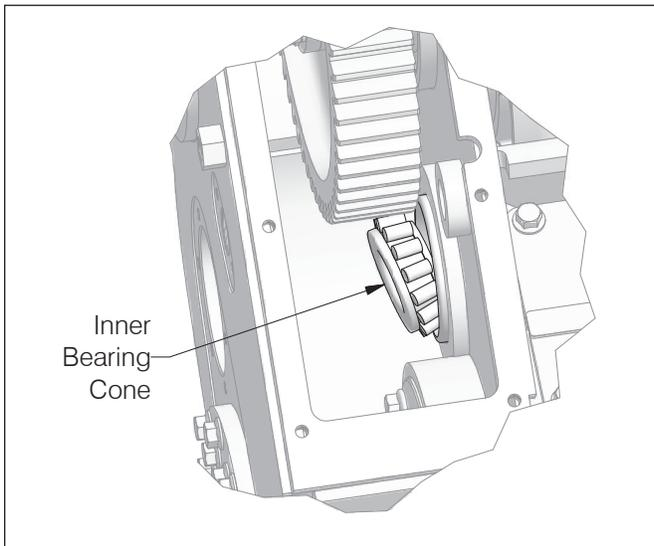
2. Position the FREESPOOL drum pinion in the housing.
