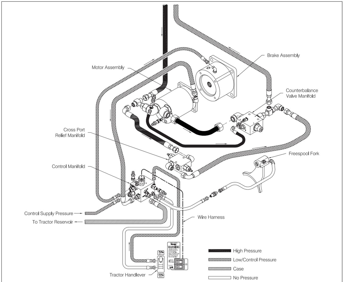
**Figure 1-17 Hydraulic System - LINE-OUT**
