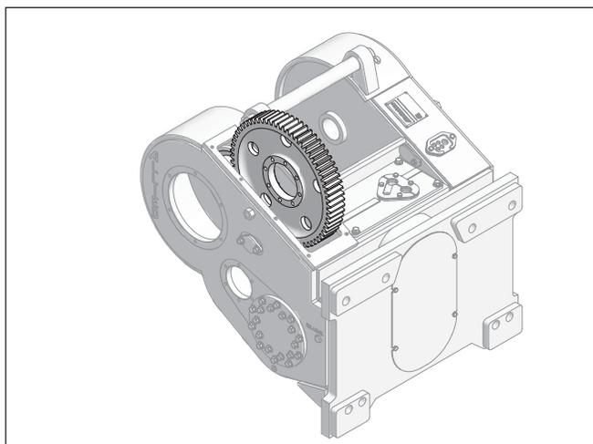
14. Remove and discard adapter seal from winch housing.
