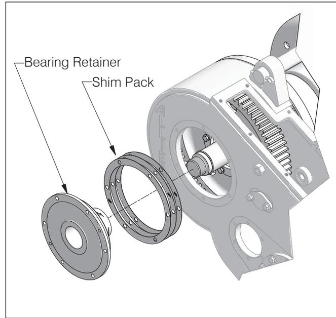
**NOTE: Tag shim pack for reference during reassembly.**
