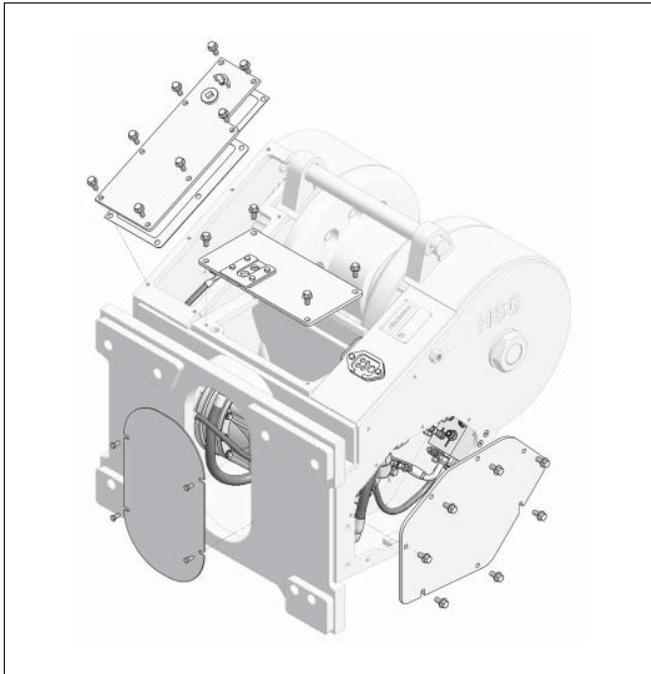
3. Remove the five hoses and wire harness that exit through the frame.
