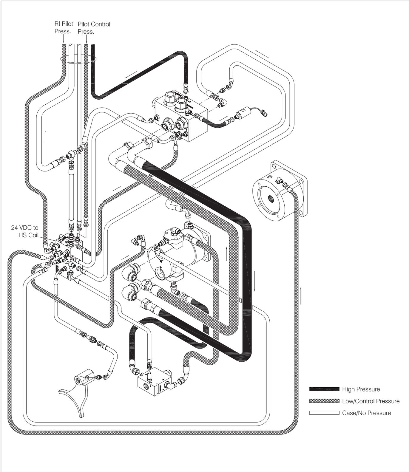
Figure 1-21 Hydraulic System - HI-SPEED LINE-IN
