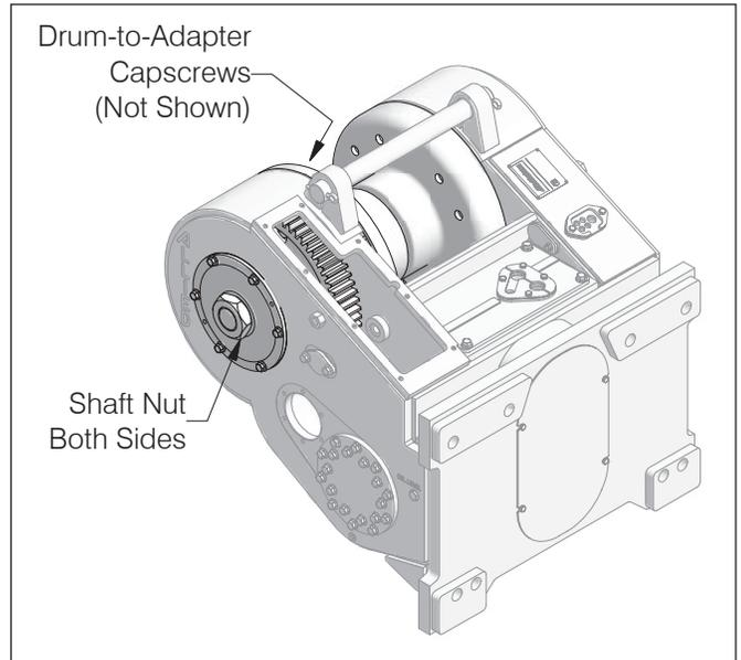
18. Tighten drum-to-adapter capscrews to 155 ft-lbs (21 kg-m) torque.
