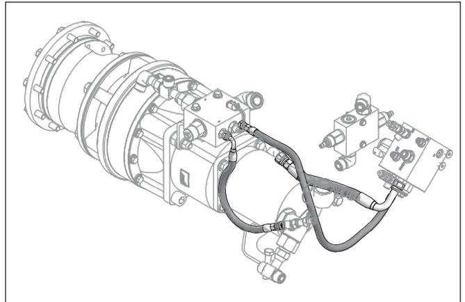
6. Remove the control manifold.
