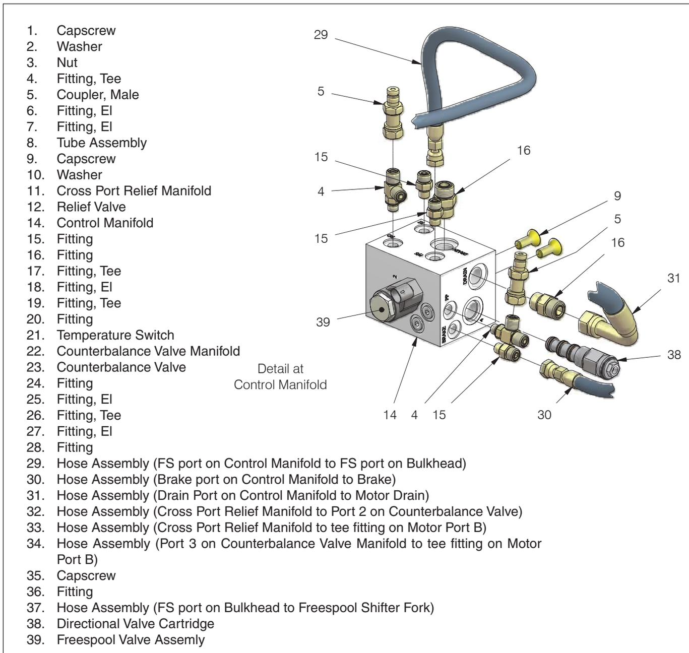
Figure 4-3 Hydraulic System Components, Rescue Winch\_2
