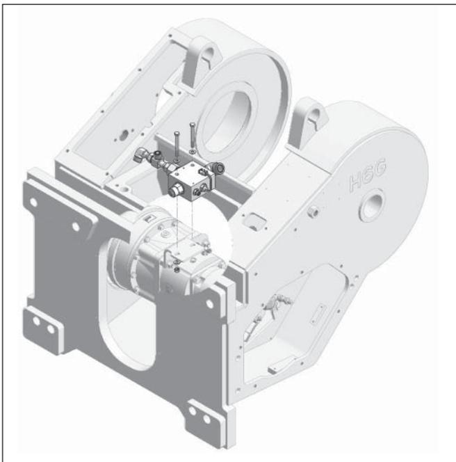
3. Install the control manifold.
