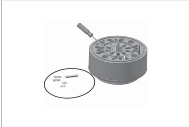
7. Lift up rotor/stator cartridge and remove from the rear housing.
