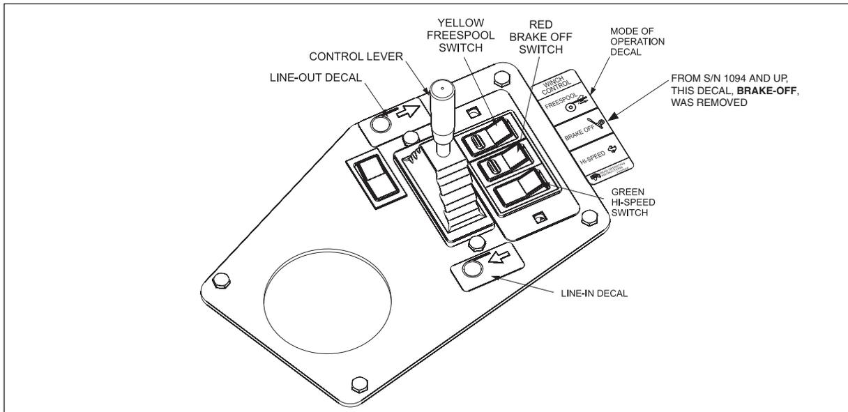
**Figure 1-11 Winch Controls**
