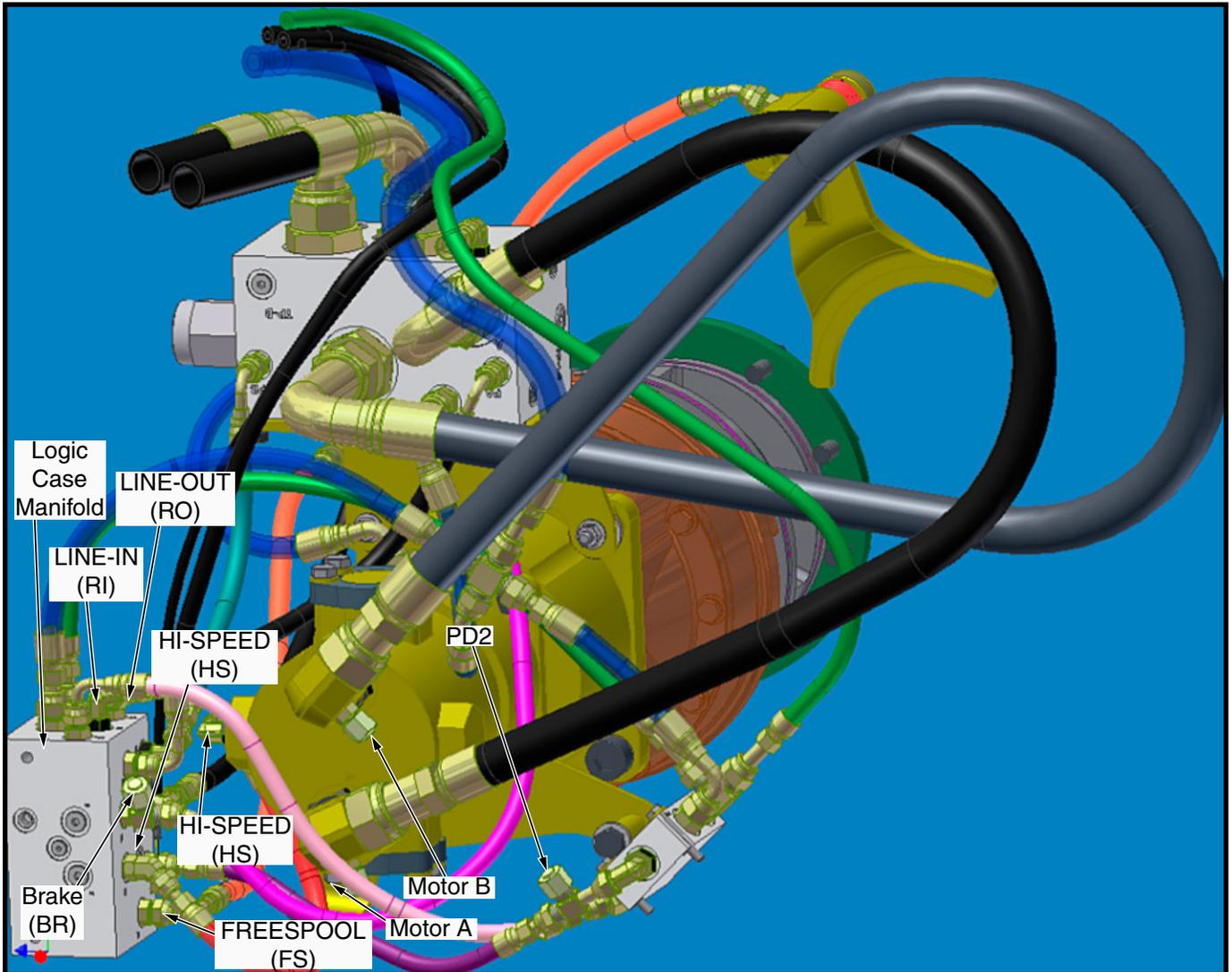
**Figure 3-4 Hydraulic Pressure Test Ports: S/N H6G-1020 and below**
