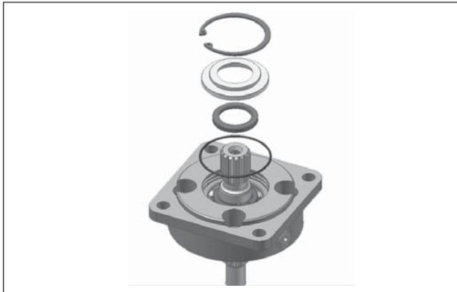
9. Install main body O-ring and ball checks into front housing. Place a small amount of grease over ball checks and O-ring, then wipe off excess grease.
