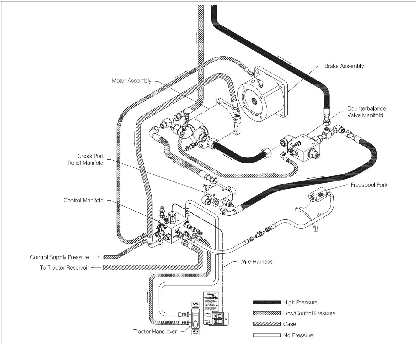
**Figure 1-16 Hydraulic System - LINE-IN**
