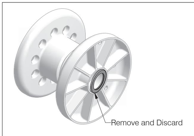
**NOTE:** This seal must be replaced with a new Allied Systems Company-approved seal during reassembly.
