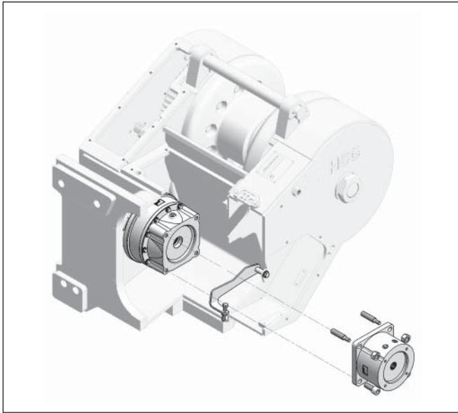
9. Install the hydraulic motor.
