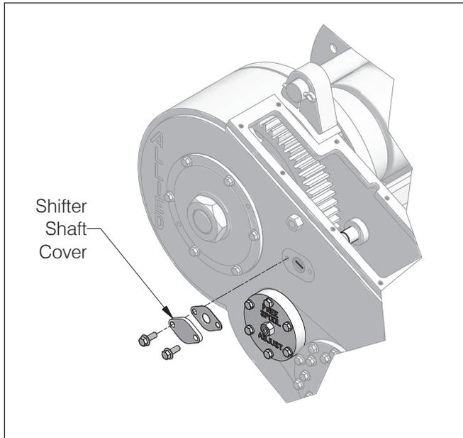
3. Withdraw the shaft by rotating counter clockwise and remove the fork.
