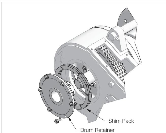
16. Secure retainer with capscrews and lockwashers. Tighten capscrews to 75 ft-lbs (10 kg-m).
