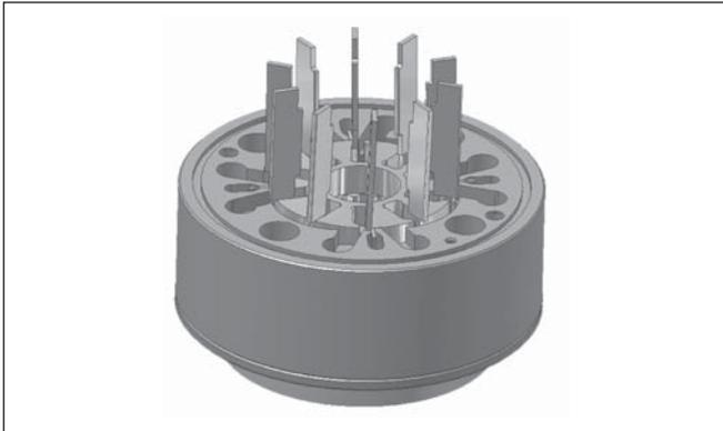
**NOTE: Make sure that the radiused edge of each stator vane points to the rotor and the radiused edge of each rotor vane points to the stator.**
