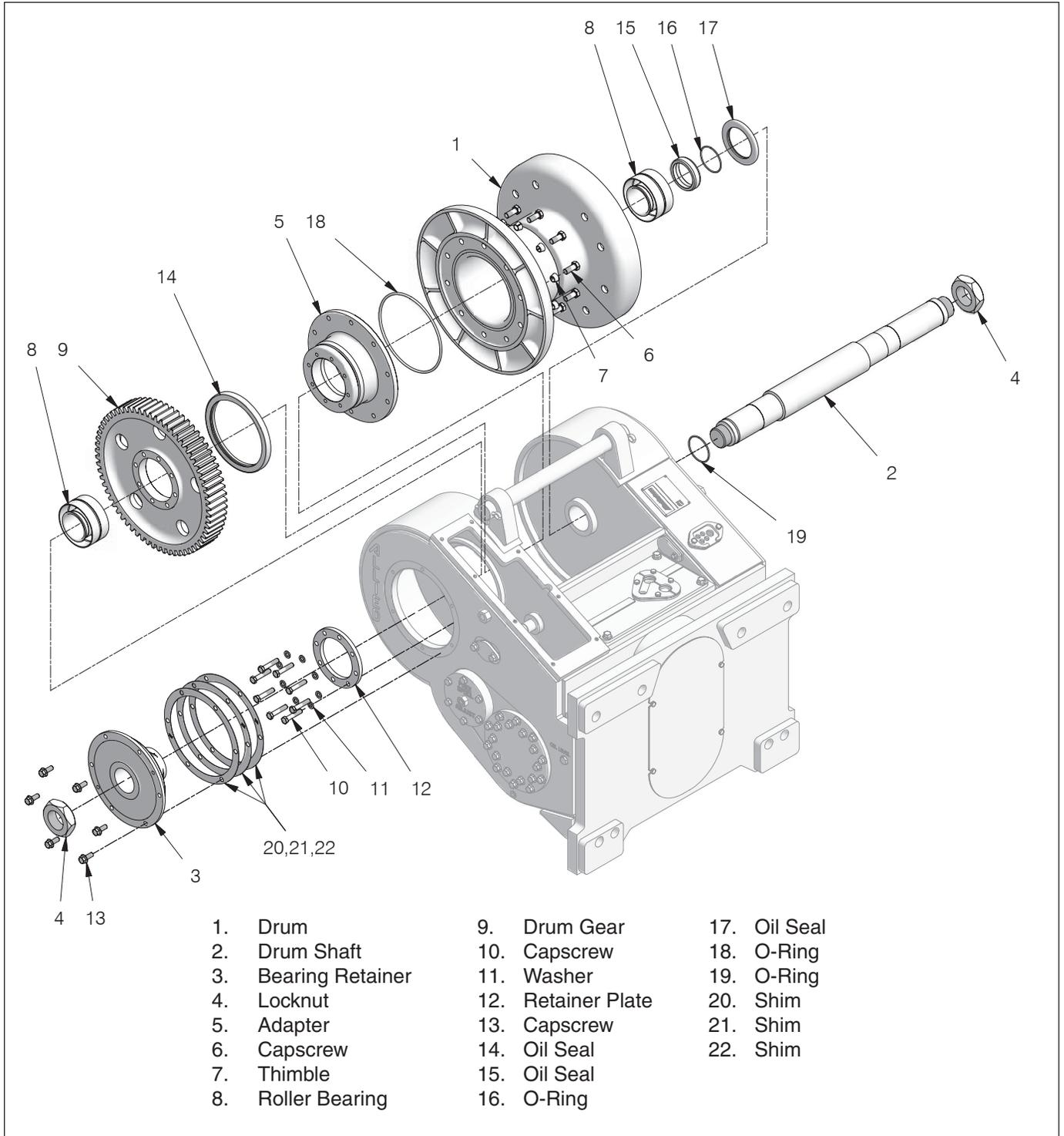
**Figure 4-2 Location of Drum and Drum Shaft Components**
