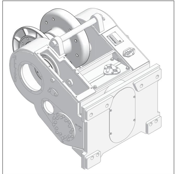
6. Lubricate right-hand drum bore. Coat right-hand seal ring and groove with O-ring lube. Install new seal ring.
