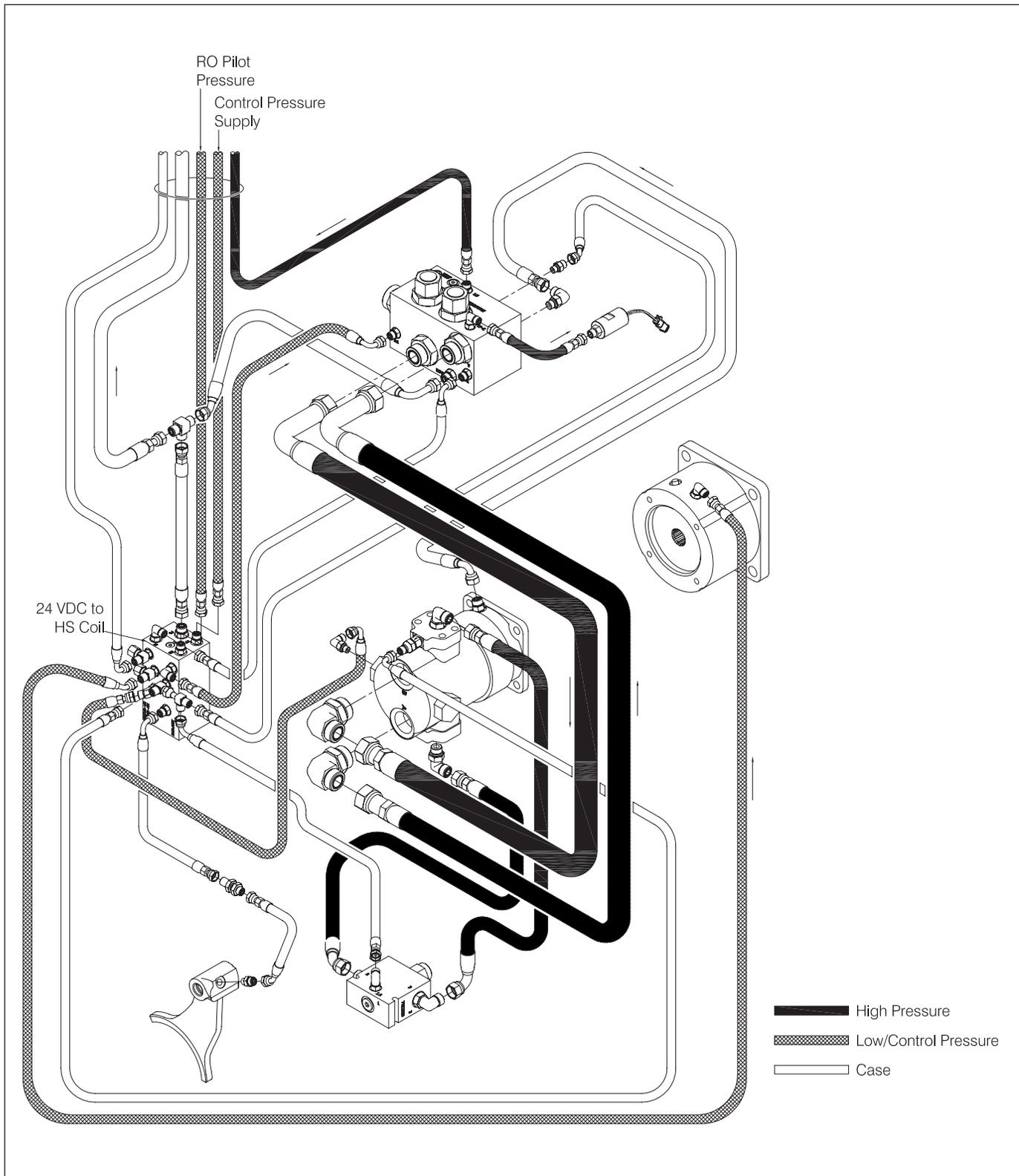
Figure 1-23 Hydraulic System - HI-SPEED LINE-OUT
