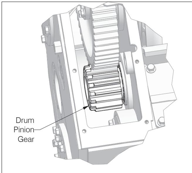
3. Place dental clutch on pinion gear. Ensure chamfered ramp faces pinion.
