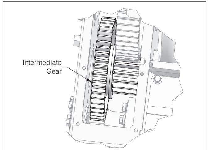
**NOTE: Install intermediate gear with high shoulder down.**
