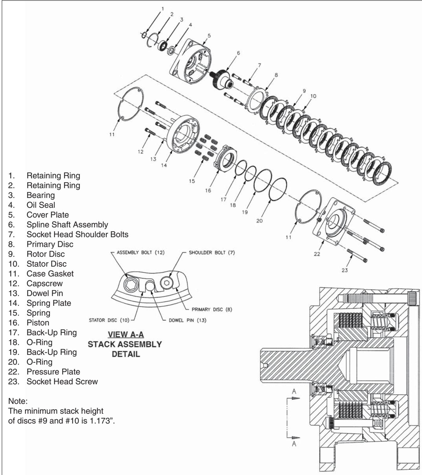
Figure 4-6 Brake Assembly
