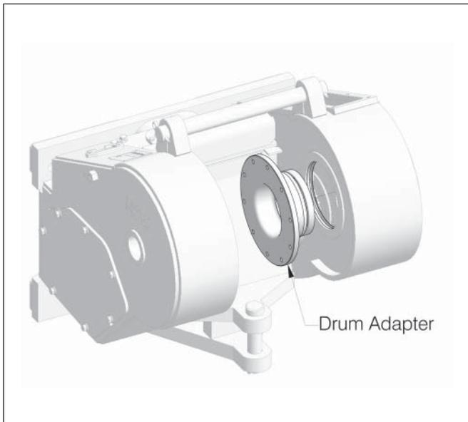
4. Lubricate the left-hand drum bore with Lubriplate or other light lube grease, then install double tapered roller bearing assembly.
