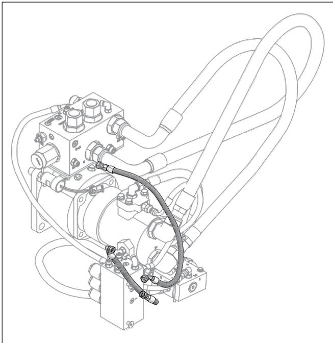
8. Remove the logic manifold.
