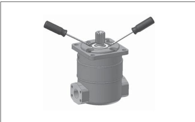
3. Mark one side of the motor for proper assembly, paying careful attention that the cartridge will not be installed upside down. Secure the motor prior to loosening the 5/8-11 bolts.
