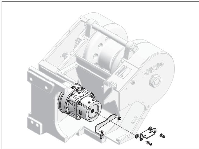
5. Remove manifold support bracket from frame.
