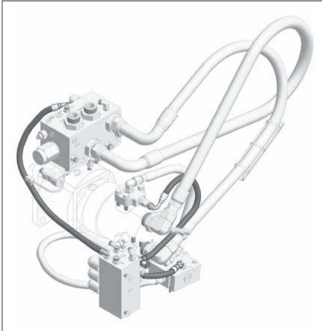
8. Install the hoses connecting the directional manifold to the logic manifold.
