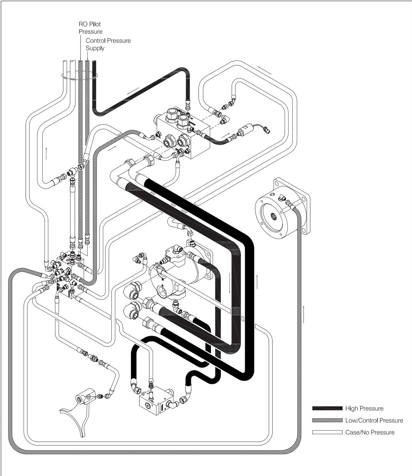
Figure 1-22 Hydraulic System - LINE-OUT
