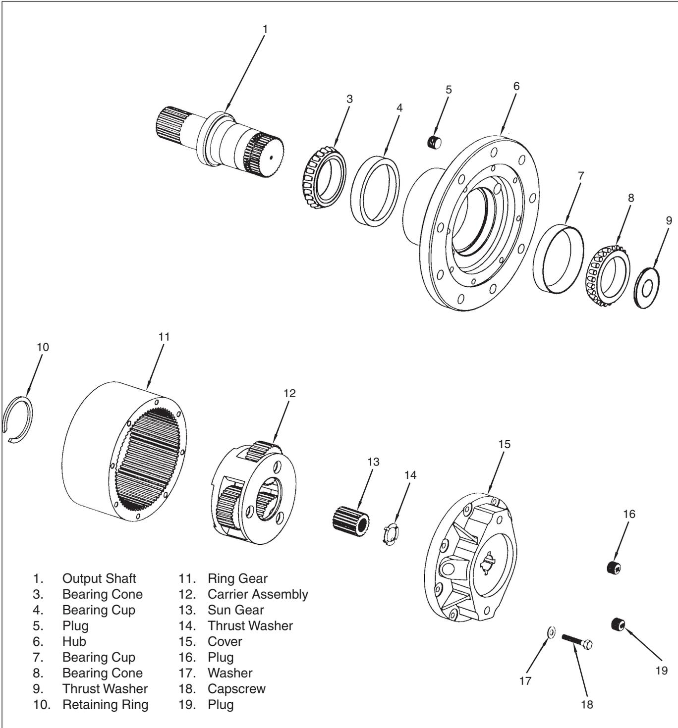
Figure 4-9 Planetary Reducer Assembly
