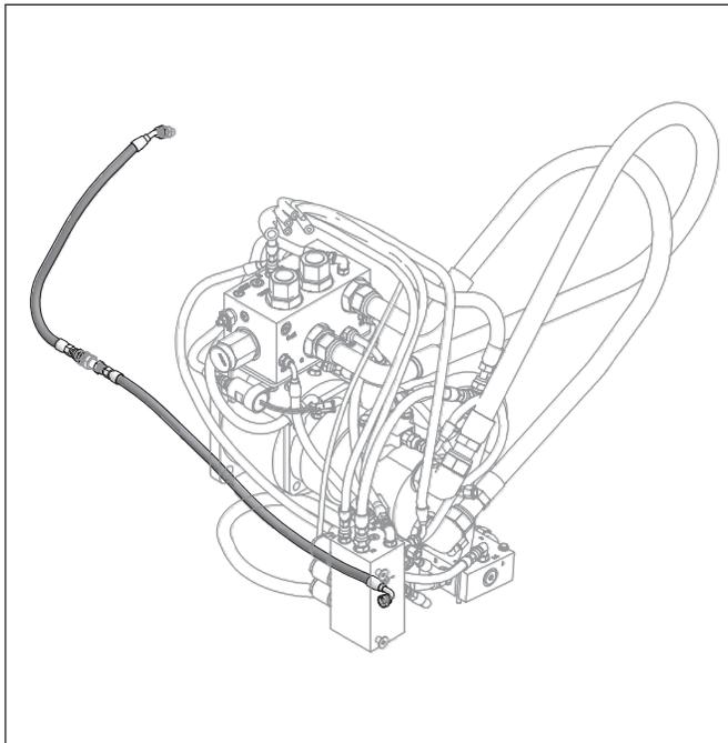
4. Remove both hoses at the directional manifold.
