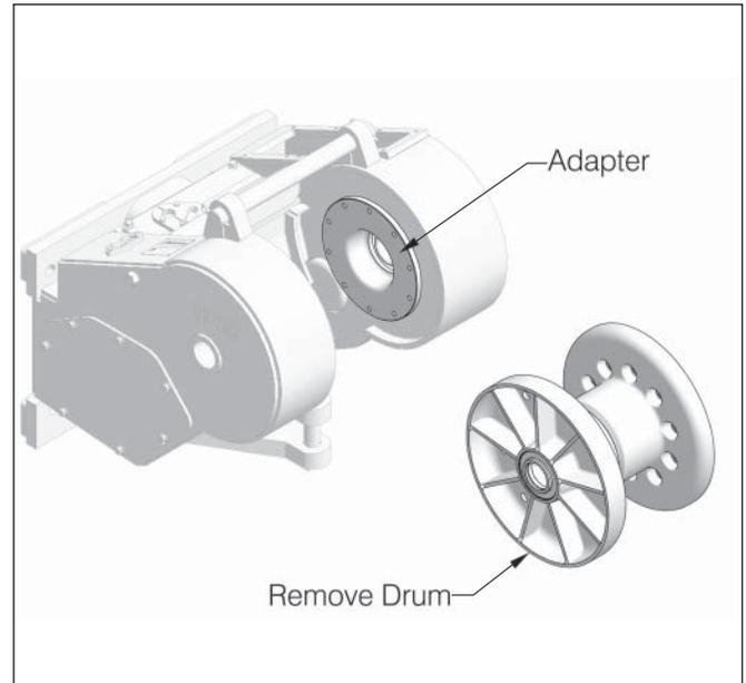
6. Attach a sling around the drum and hoist until there is no slack, then drive the shaft out the right hand side.
