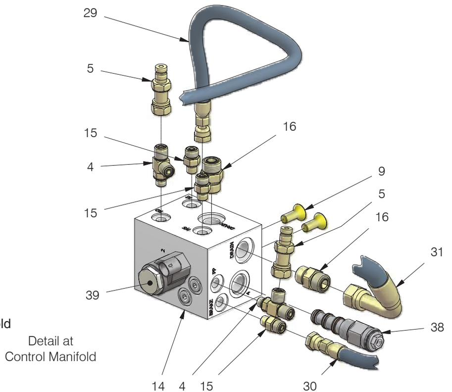
**Figure 4-12 Hydraulic System Components, Rescue Winch\_2**
