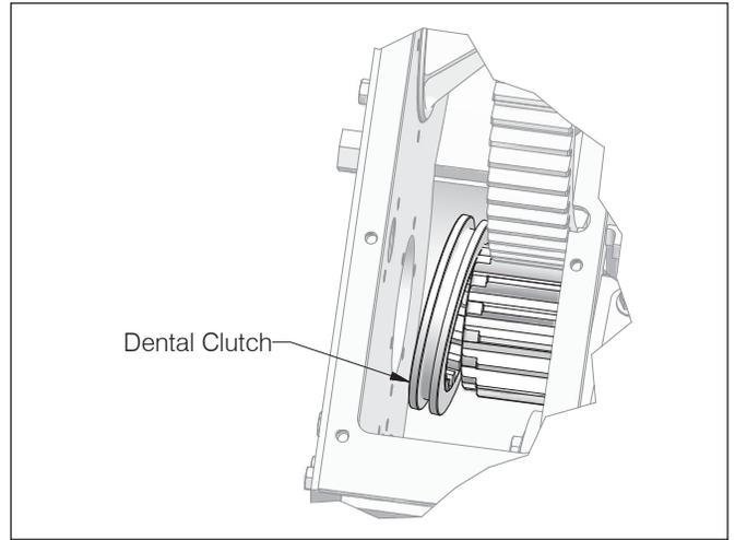
4. Position intermediate gear in housing.
