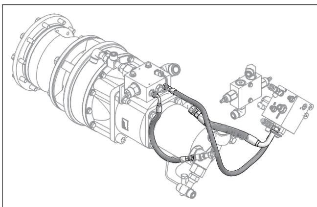
5. Install tube assembly at Port A on the motor.
