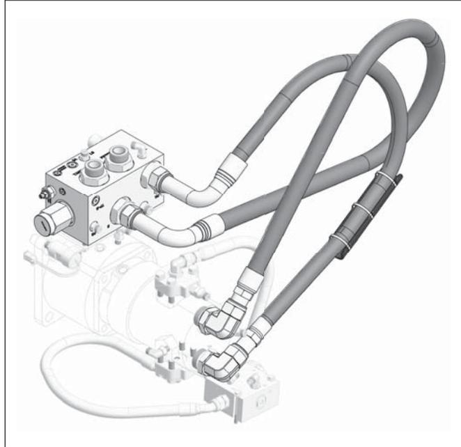
5. Install the logic manifold.
