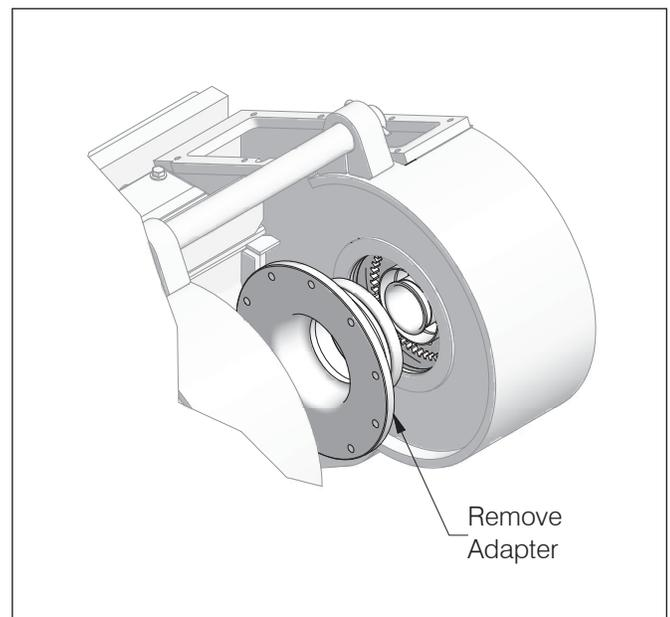
**NOTE: Support or sling the drum gear so that it does not fall during shaft removal.**
