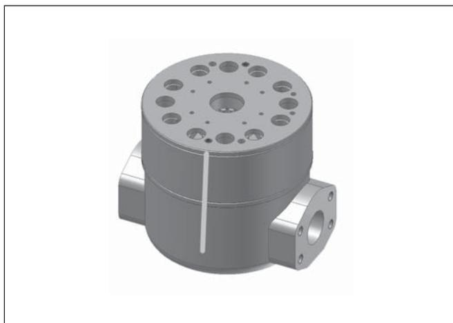
11. Install 5/8-11 bolts. Torque bolts to 50 ft. lbs.
