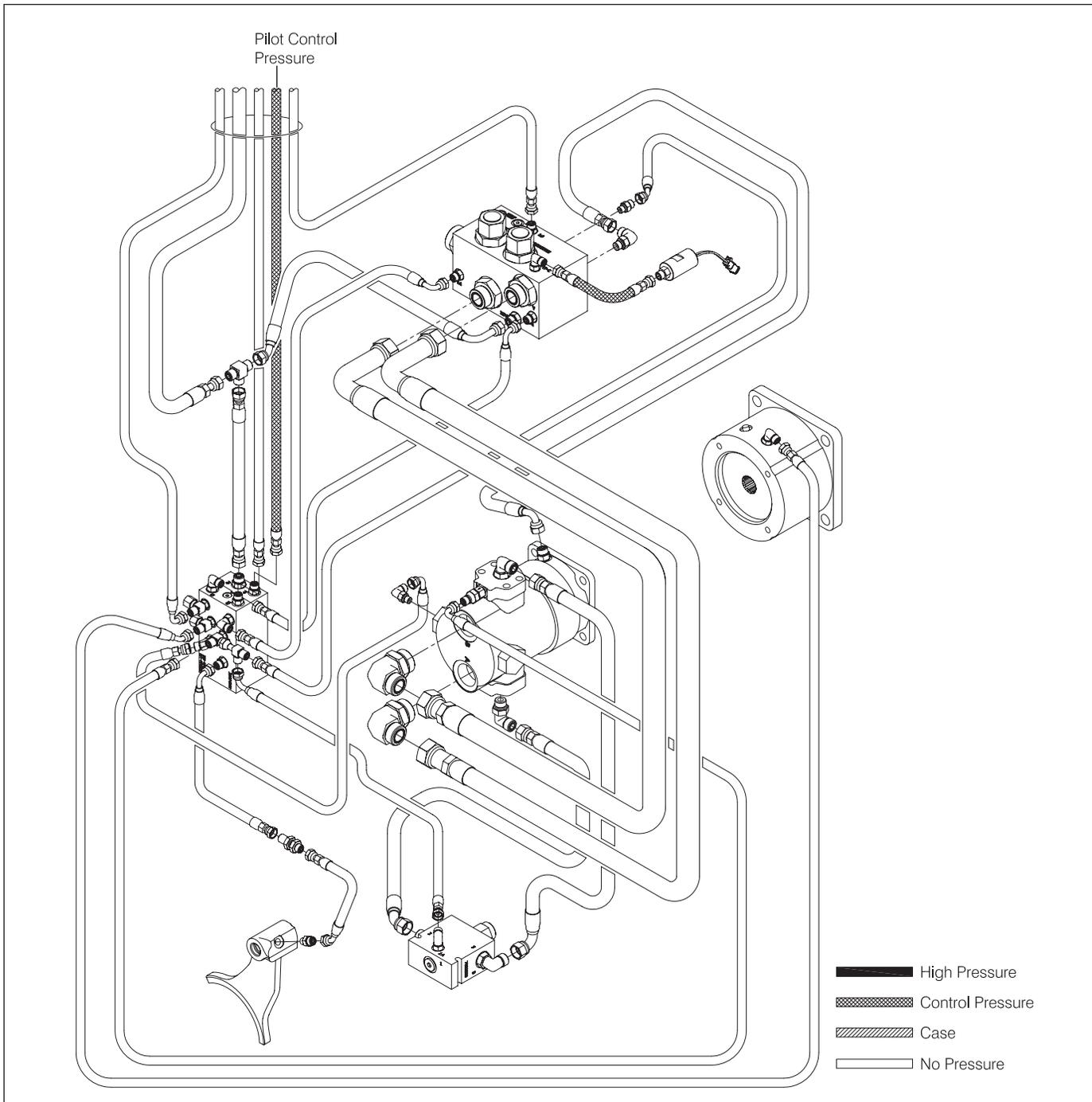
Figure 1-19 Sequence of Operation - BRAKE-ON
