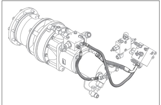
6. Remove the control manifold.
