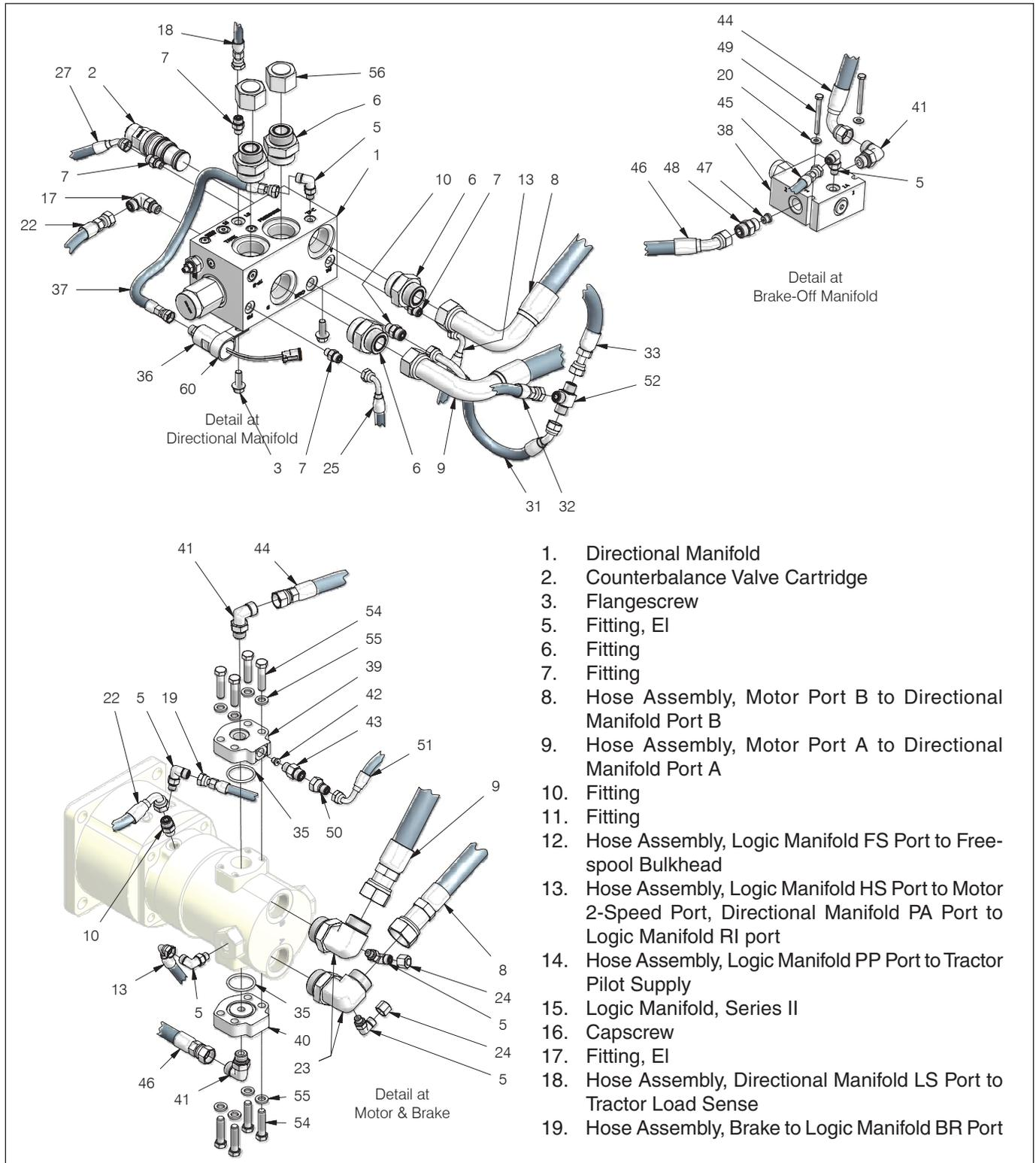
**Figure 4-4 Hydraulic System Components, High-Performance Winch\_1**
