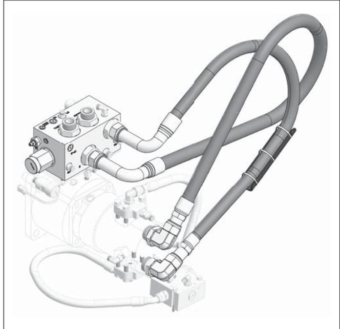
5. Install the logic manifold.
