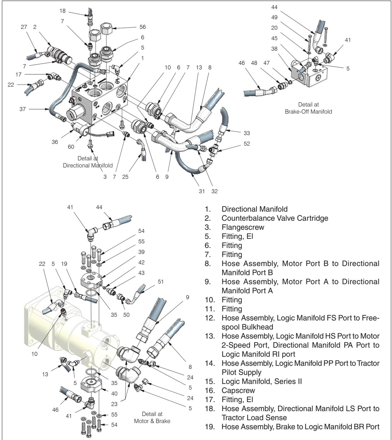
**Figure 4-4 Hydraulic System Components, High-Performance Winch\_1**
