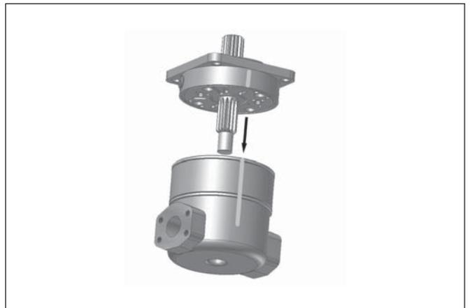
8. Place rotor/stator cartridge onto rear housing. **NOTE: Make sure assembly marks from step 3 in the Motor Assembly section are lined up.**
