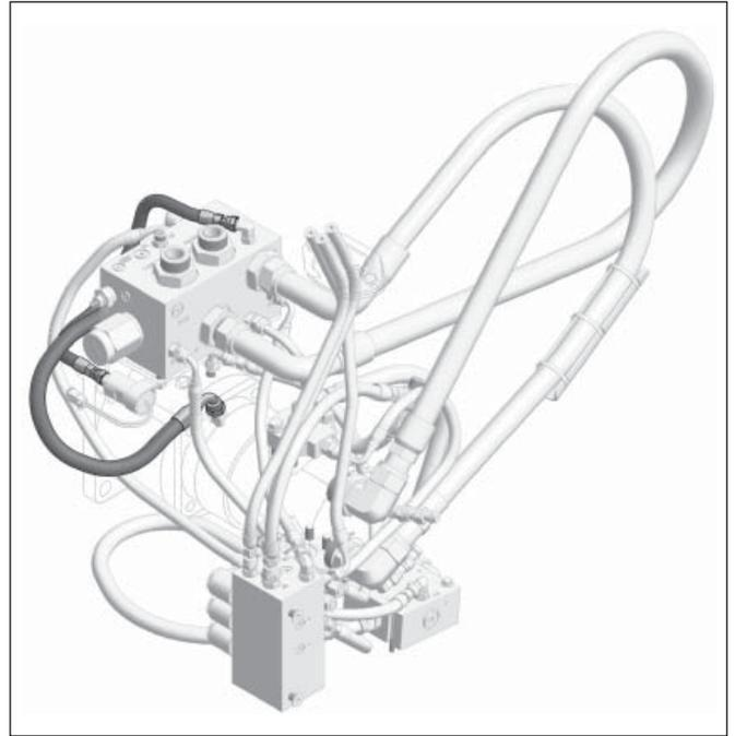
7. Connect the hoses from the logic manifold to the motor and the brake.
