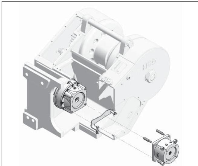
6. Remove planetary reducer assembly.
