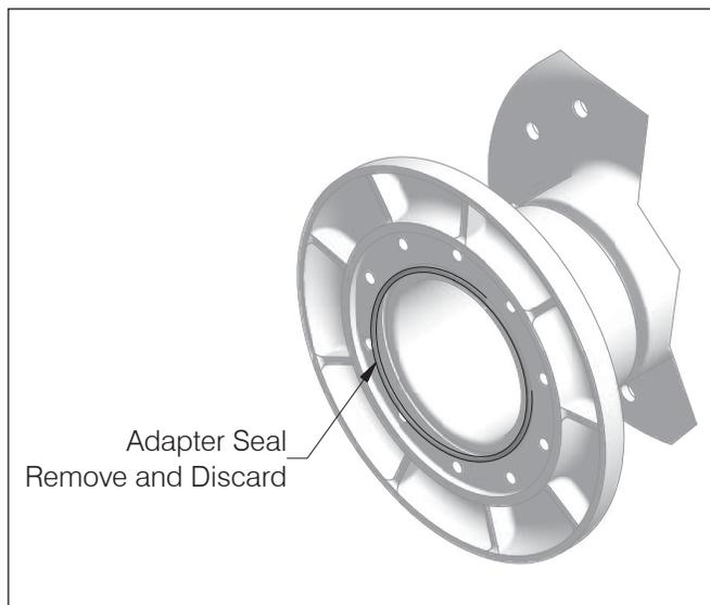
**NOTE:** This seal must be replaced with a new Allied Systems Company-approved seal during reassembly.
