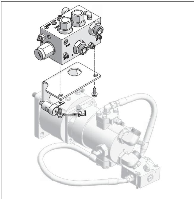
12. Remove the brake-off manifold assembly from frame.
