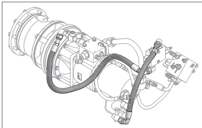
4. Remove tube assembly at Port A on the motor.
