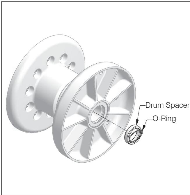
7. Move the drum into position while being careful not to move the seal ring.
