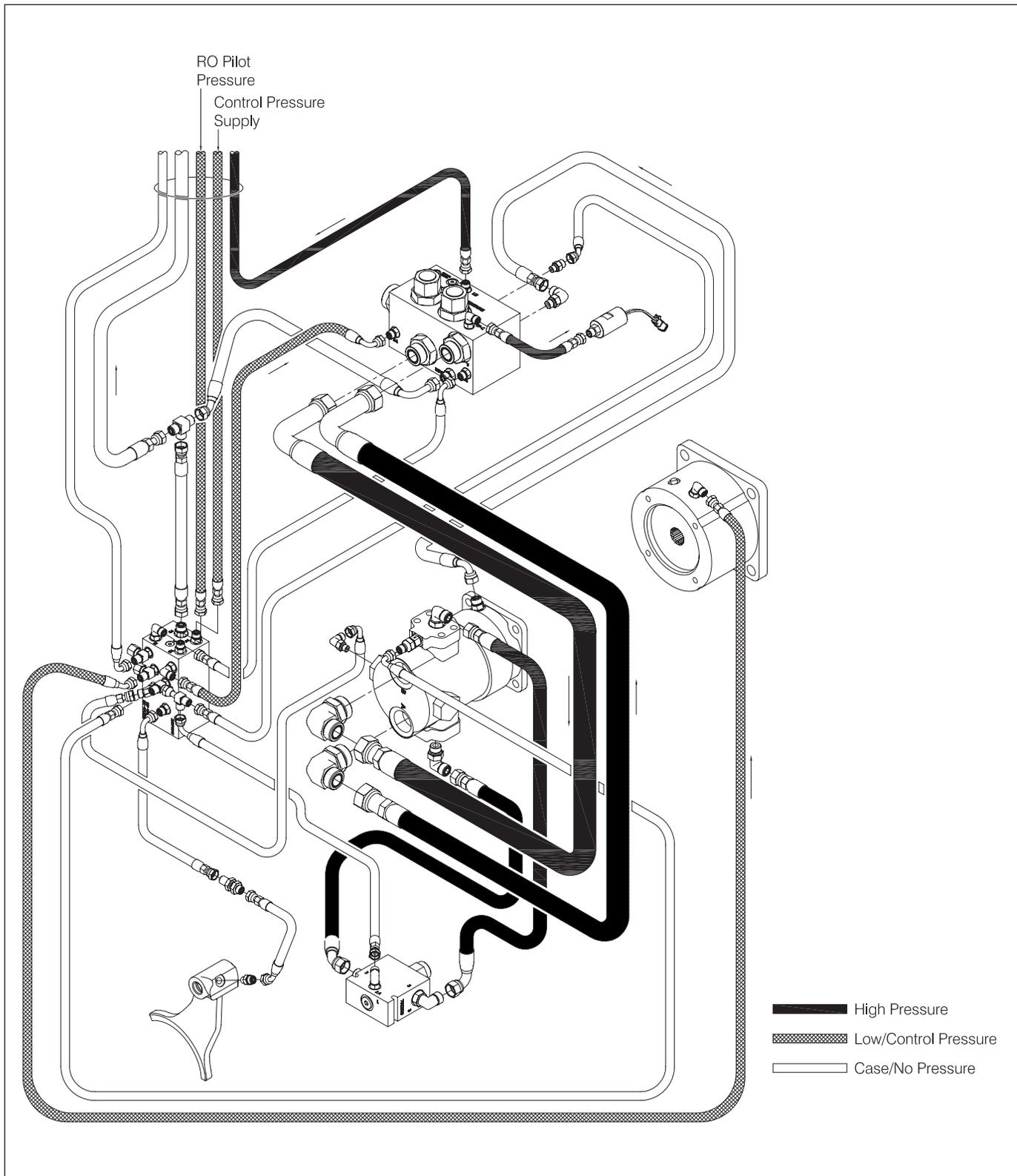
Figure 1-22 Hydraulic System - LINE-OUT
