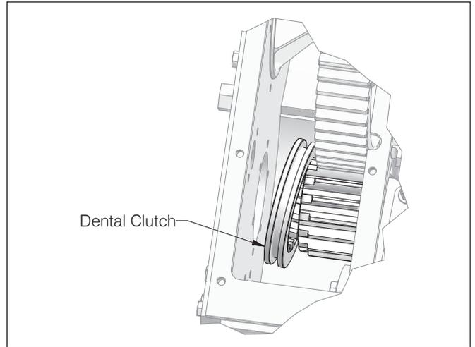
4. Position intermediate gear in housing.
