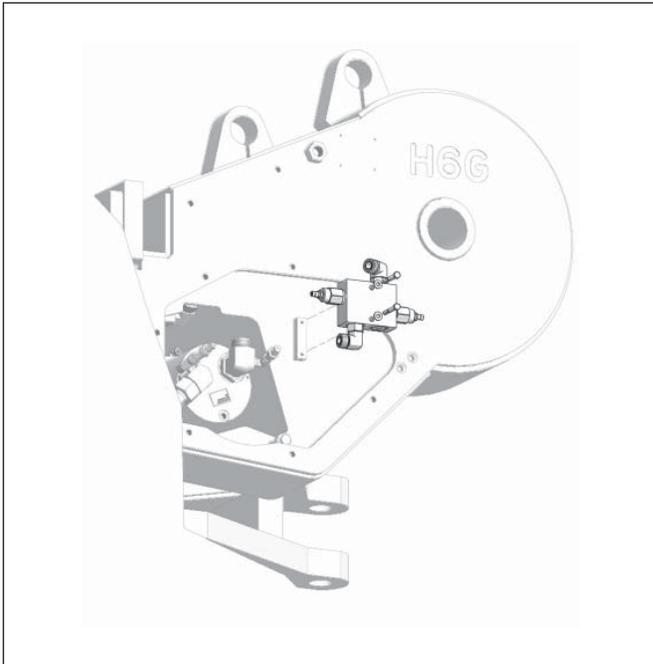
8. Remove the counterbalance valve manifold.
