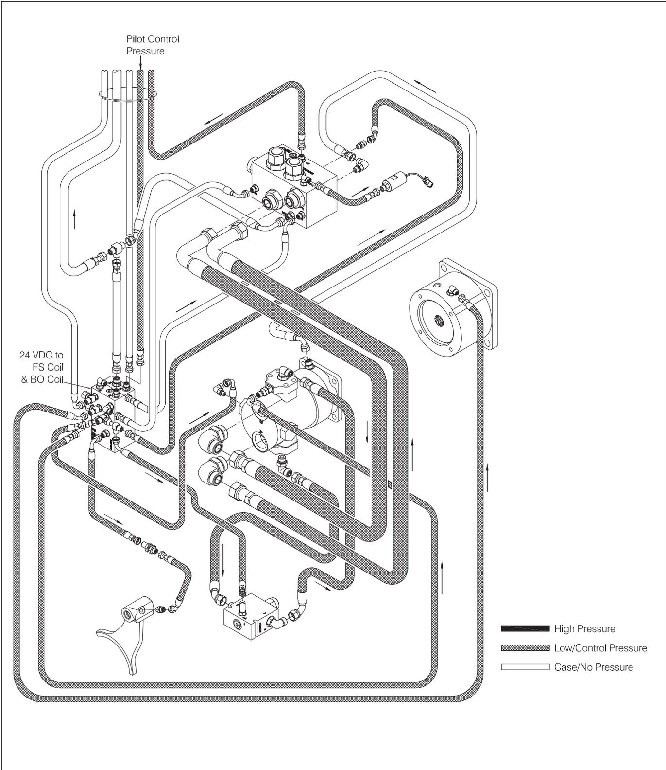
Figure 1-25 Hydraulic System - FREESPOOL
