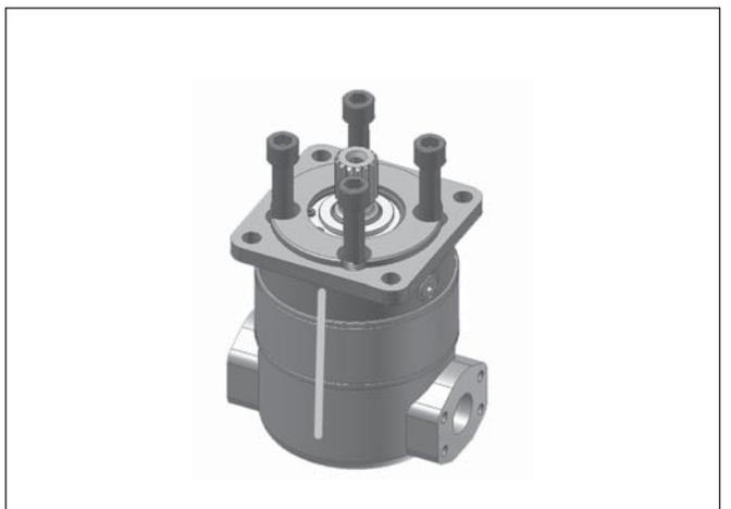
12. Rotate shaft in both directions to assure that the shaft turns smoothly. Torque motor to 190 ft. lbs. Rotate shaft again in both directions to assure that the shaft turns smoothly.
