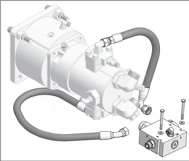
2. Install the directional manifold bracket.
