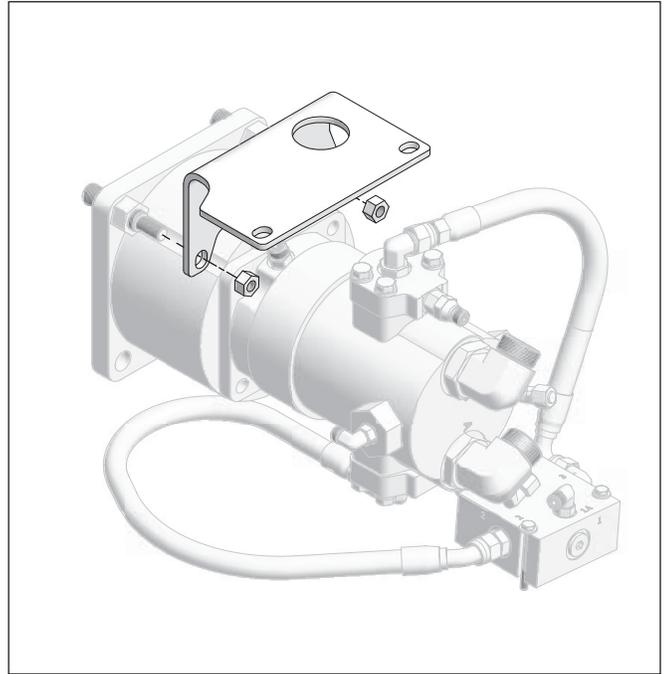
10. Remove the directional manifold assembly.
