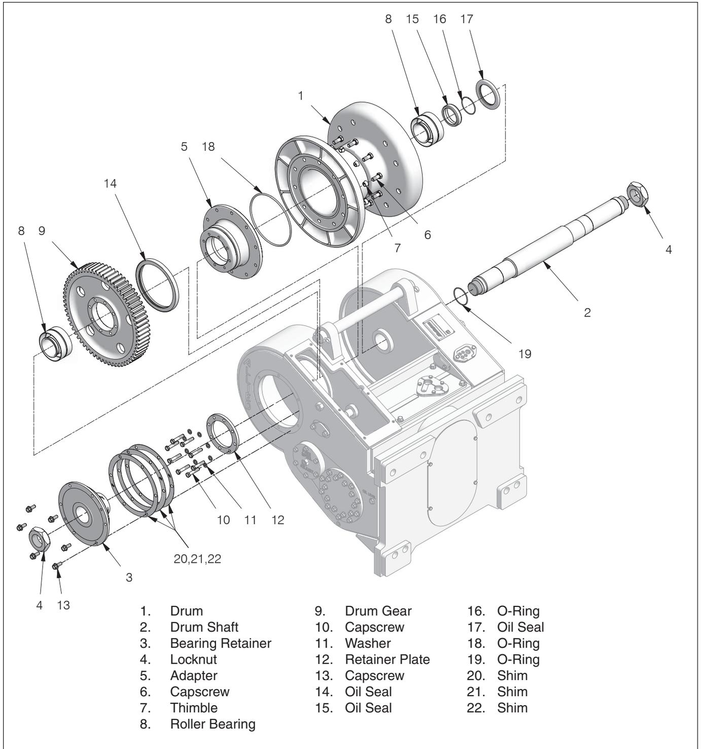
**Figure 4-16 Location of Drum and Drum Shaft Components**
