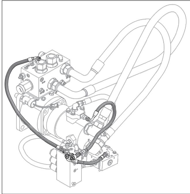
6. Remove the two hoses connecting the logic manifold to the motor and brake.
