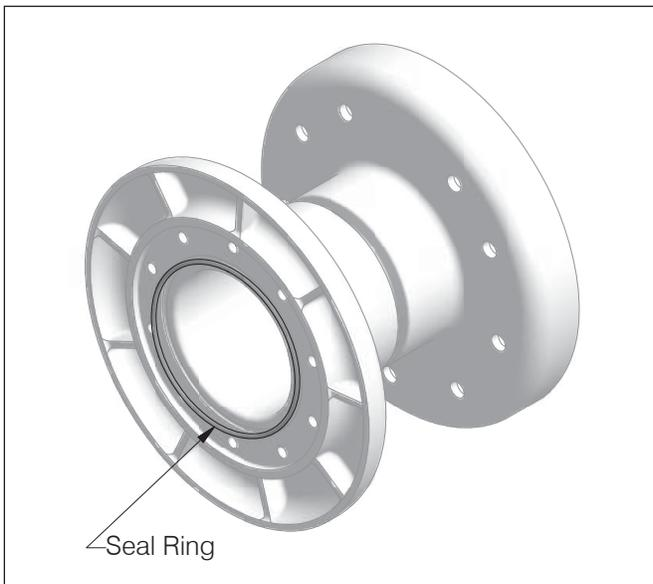
8. Align adapter and drum holes, then install the thimbles and screws. Tighten progressively and evenly to ensure uniform compression of seal ring. Do not tighten to final torque.
