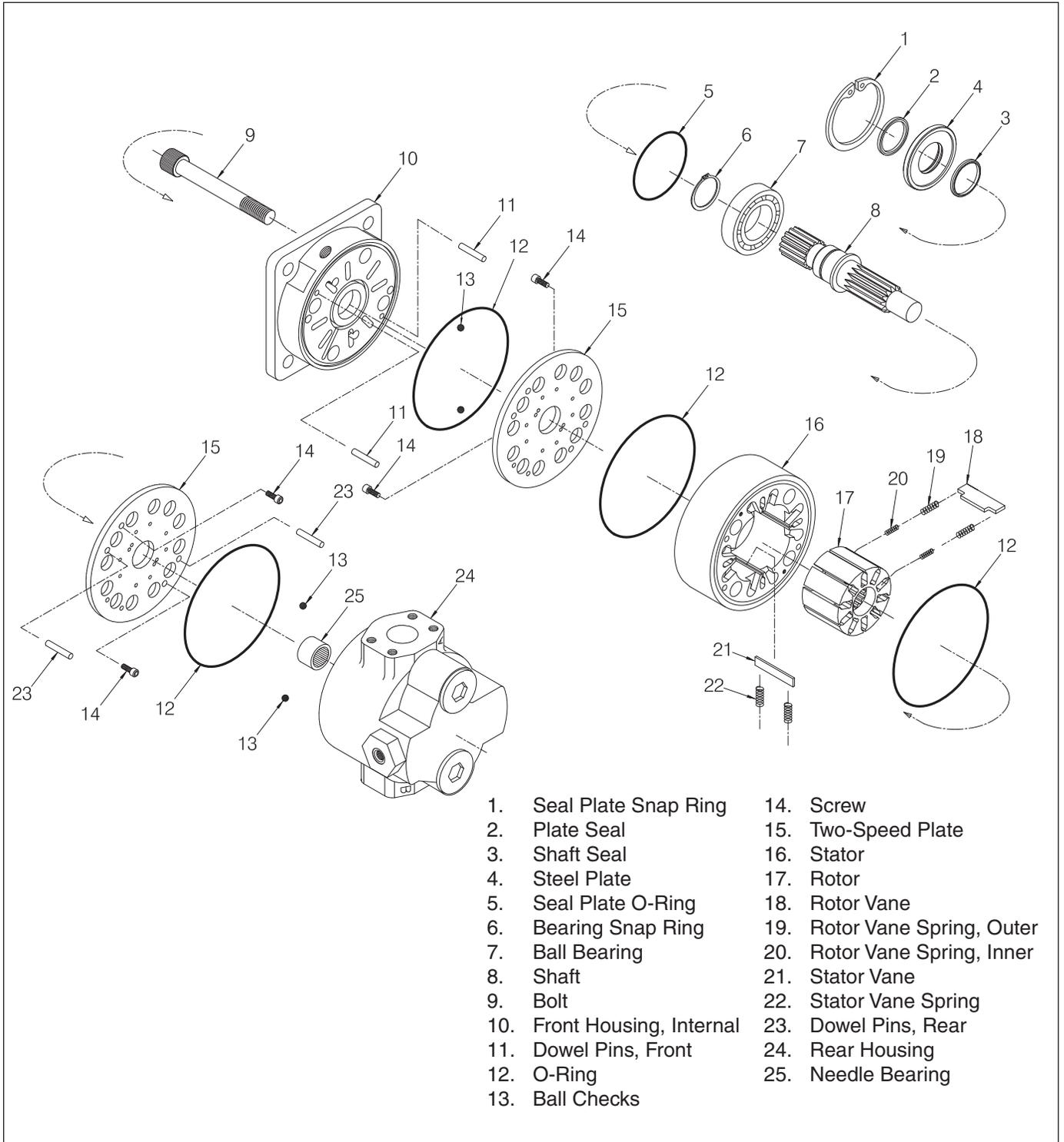
**Figure 1-14 Motor (Two-Speed Shown)**
