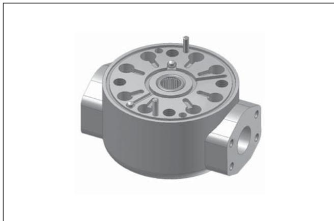
10. Install dowel pins into rotor/stator cartridge. Pour a small amount of clean oil into the cartridge, then install front housing. Make sure alignment marks are lined up.
