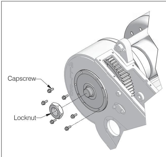
4. Remove retainer ring by removing retainer capscrews.
