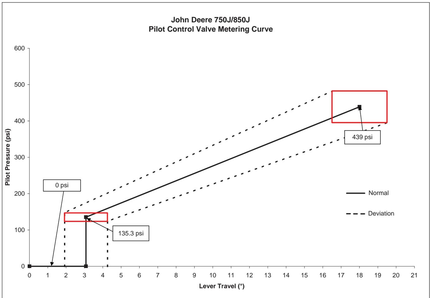
**Figure 2-1 Output Pressures from Pilot Controller Unit on Control Lever vs. Angle of Lever Deflection**
