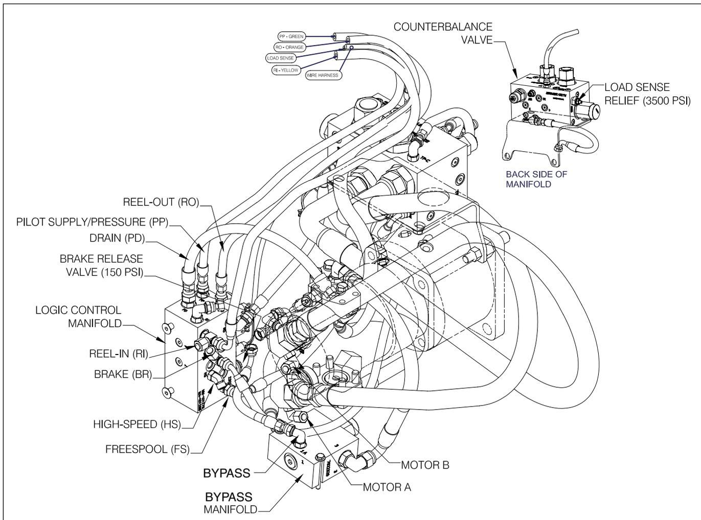
Figure 3-5 Hydraulic Pressure Test Ports S/N H6G-1021 and above (some items removed for clarity)
