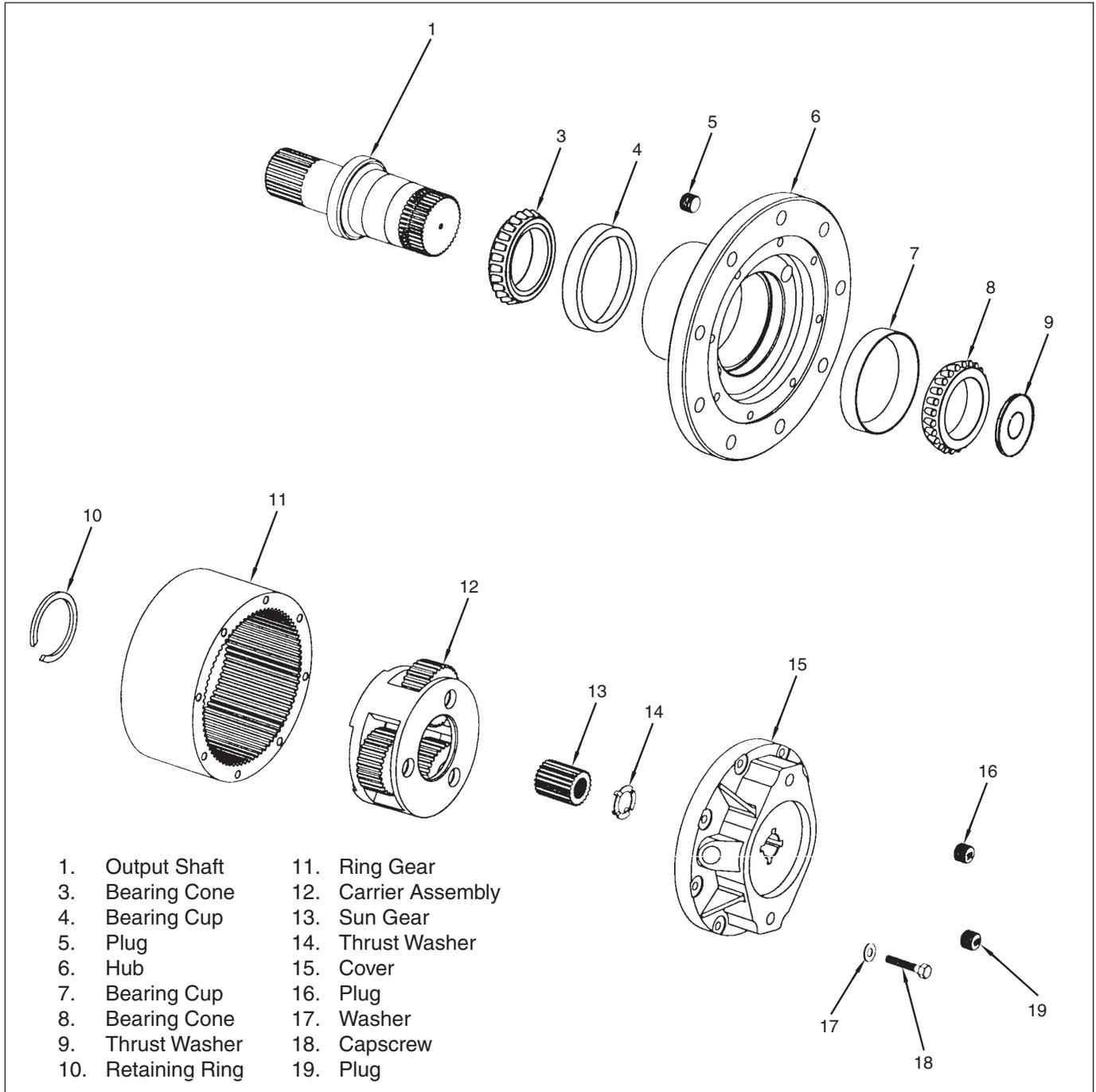
Figure 1-12 Planetary Reducer
