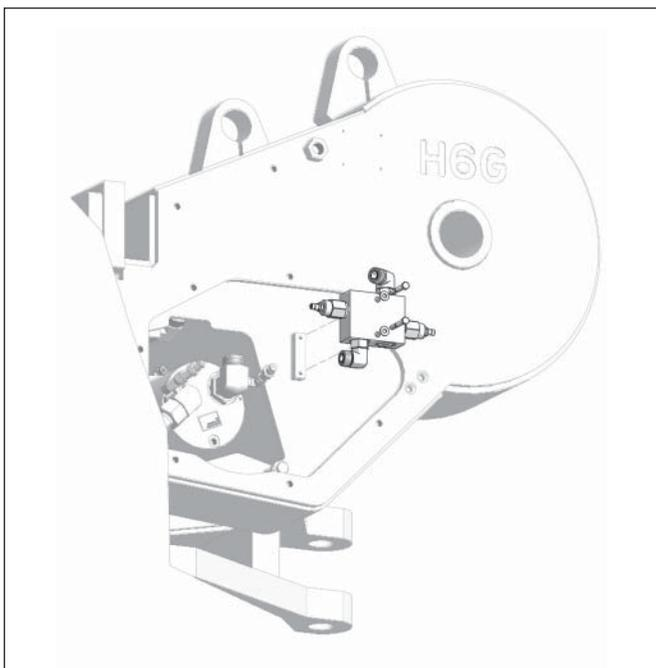
4. Connect the hoses between the control manifold and counterbalance valve manifold.
