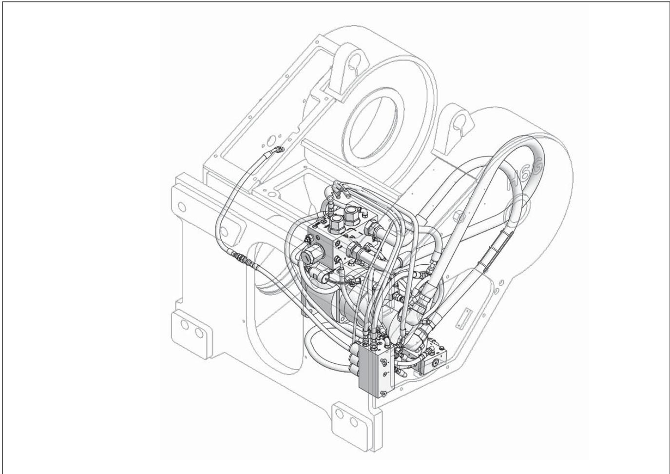
Figure 4-15 Hydraulic System, High-Performance Winch
