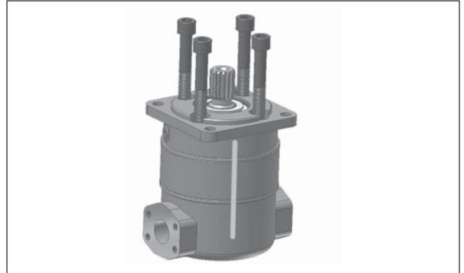
4. Remove front housing. **NOTE: Two 5/16" ball checks and one main body O-ring may be dislodged and fall free.**
