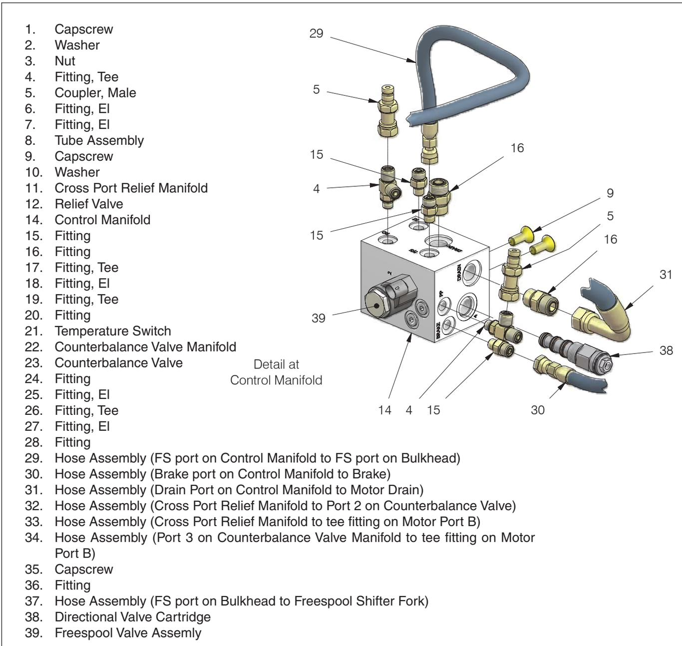
Figure 4-3 Hydraulic System Components, Rescue Winch\_2
