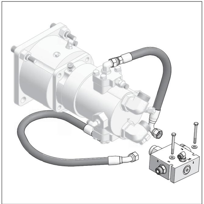
**NOTE: Port A and Port B brake-off hoses can remain on motor during motor shaft removal procedures.**
