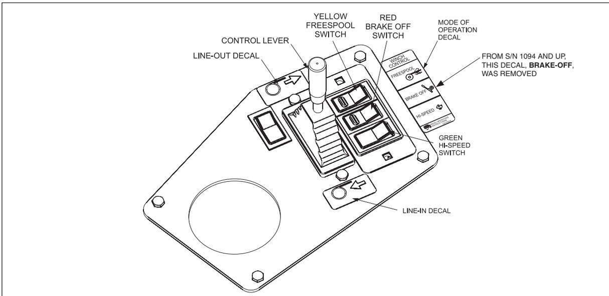
**Figure 1-11 Winch Controls**
