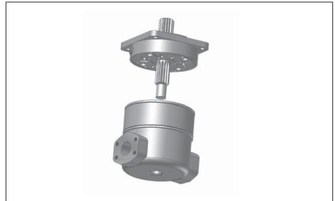
5. With the seal plate removed, press shaft and ball bearing out of front housing.
