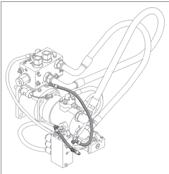
8. Remove the logic manifold.
