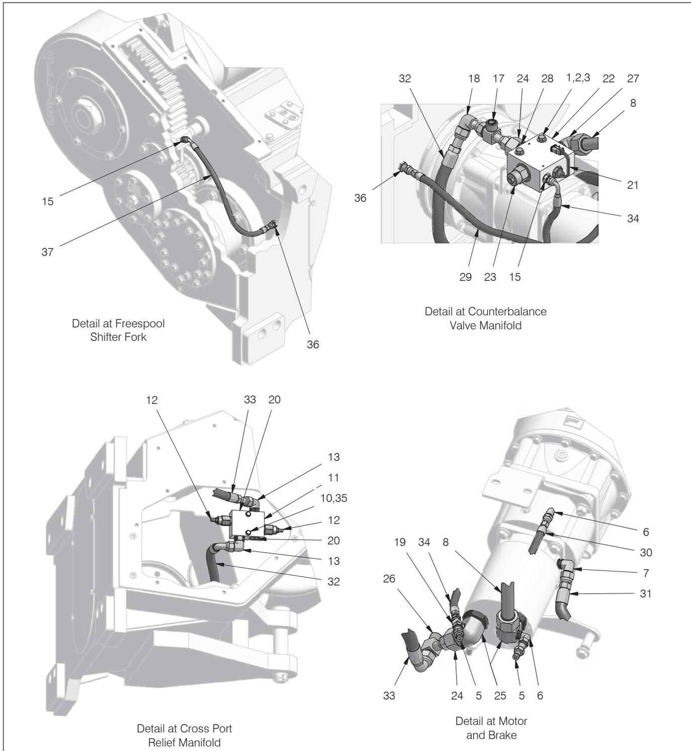
**Figure 4-12 Hydraulic System Components, Rescue Winch\_1**
