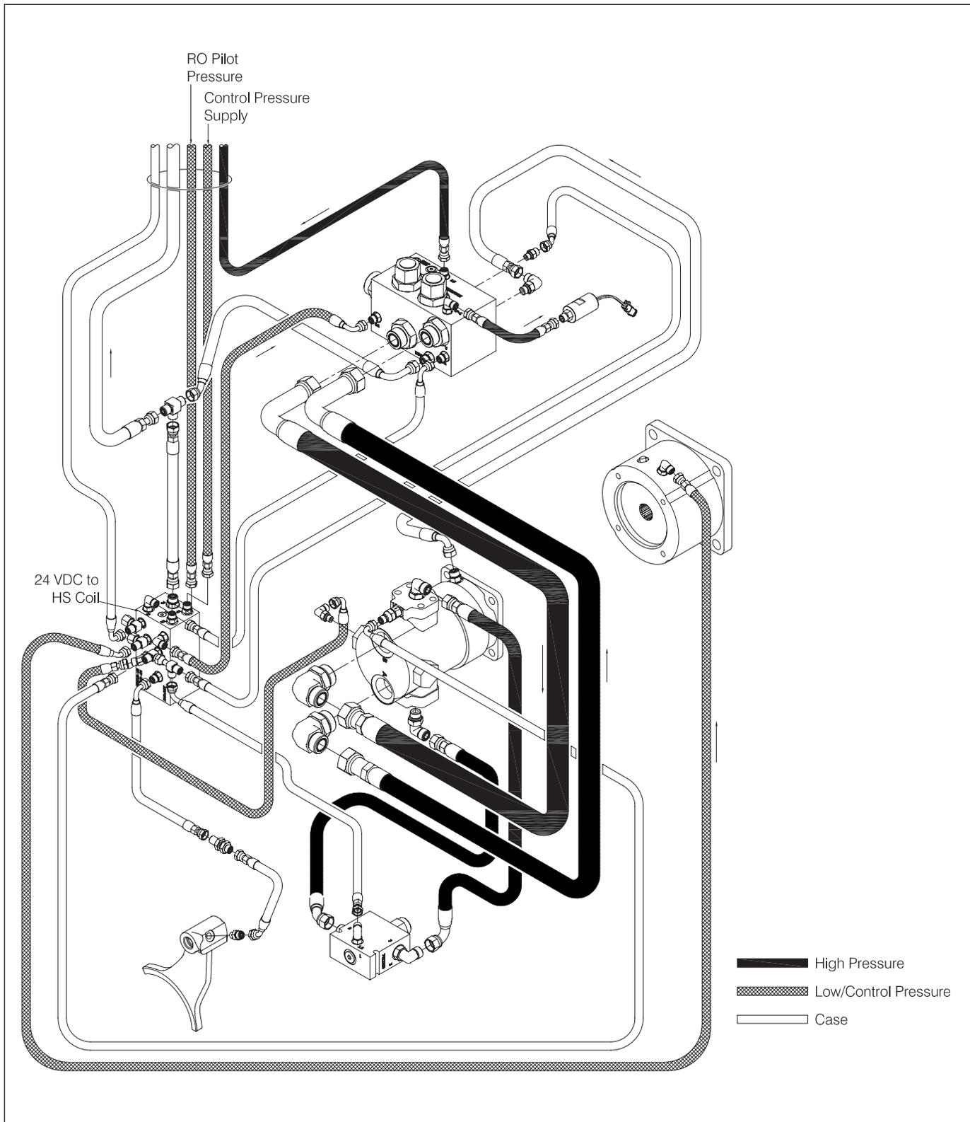
Figure 1-23 Hydraulic System - HI-SPEED LINE-OUT
