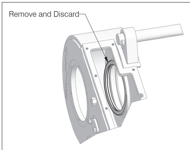
**Hydraulic System Disassembly, Rescue Winch**
