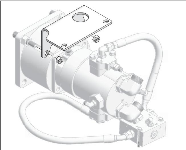
3. Install the directional manifold assembly.
