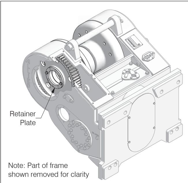
11. Make sure that double-tapered roller bearing, seal and spacer are properly seated in the left-hand side of the drum. Then install the shaft until it bottoms solidly against the left hand tapered roller bearing. Tighten left hand nut.
