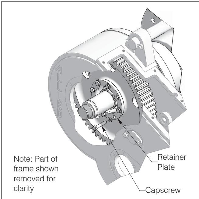
**NOTE: Capscrews cannot be installed unless drum gear and drum adapter have been aligned as indicated in Step 8.**
