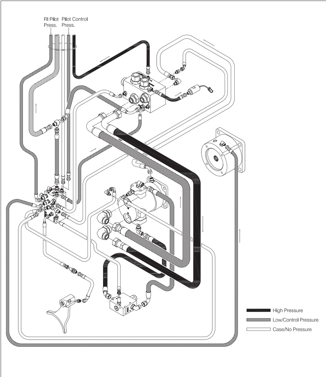
Figure 1-20 Hydraulic System - LINE-IN
