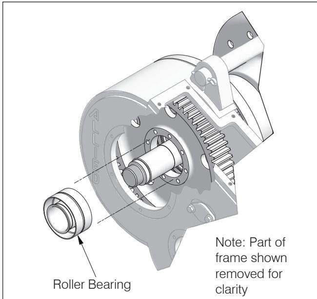
8. Carefully remove the drum from winch frame. Ensure that the adapter does not fall.
