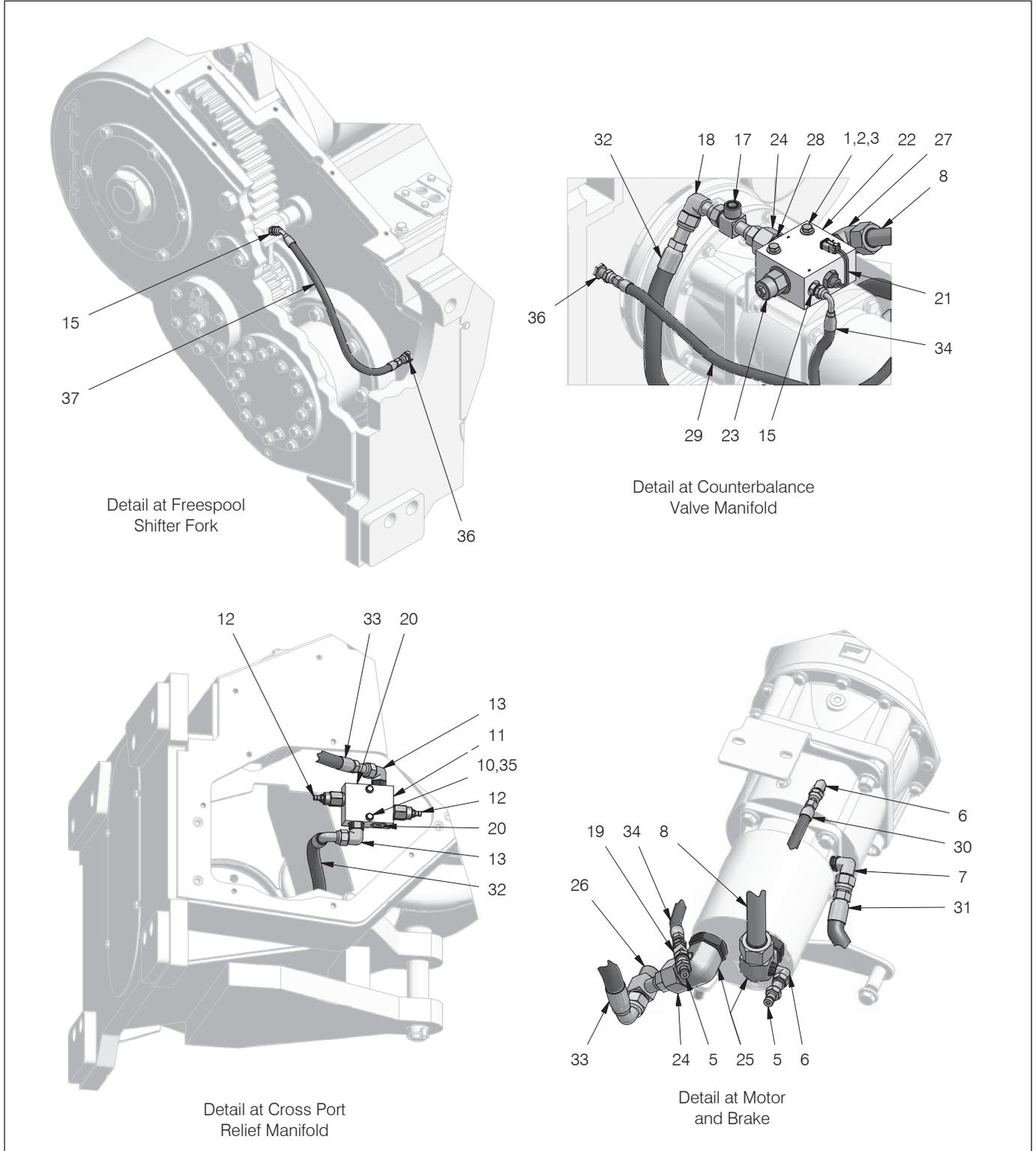
**Figure 4-3 Hydraulic System Components, Rescue Winch\_1**
