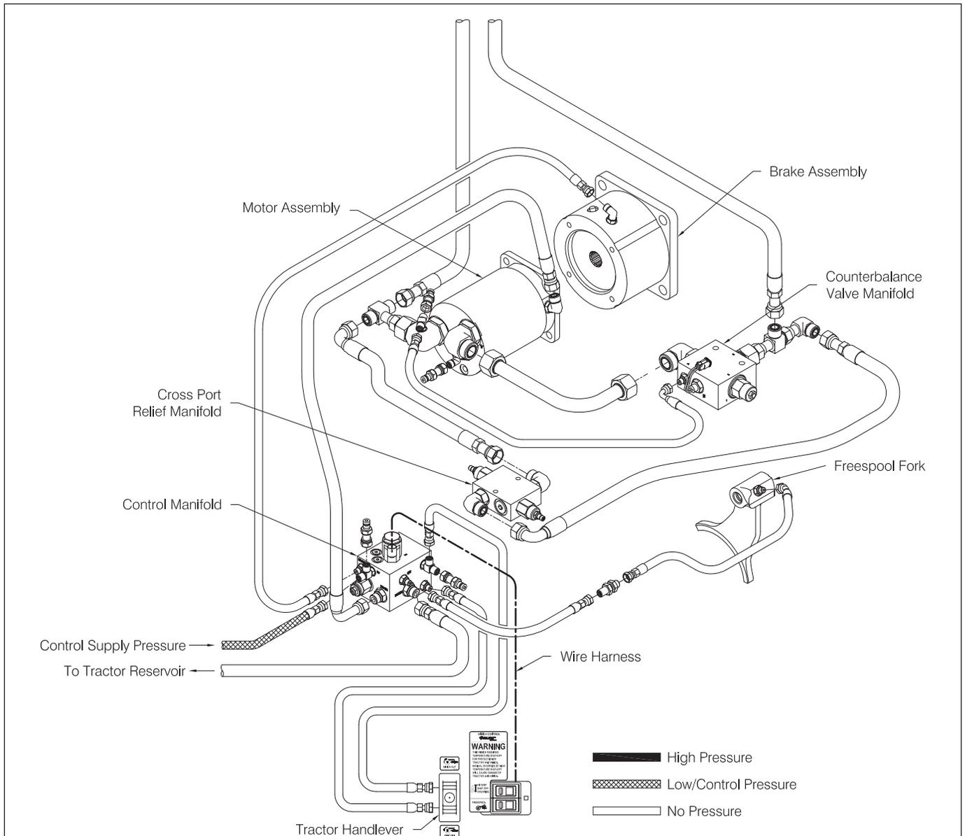
**Figure 1-15 Sequence of Operation - BRAKE-ON**
