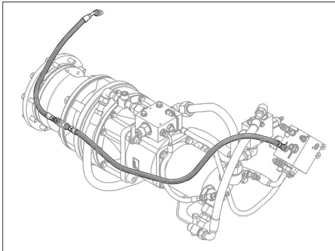
3. Remove the two hoses at the Cross Port Relief Manifold.
