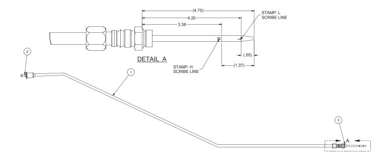
PRODUCTION: VERIFY H & L MARKS MATCH OEM DIPSTICK BEING REPLACED.
