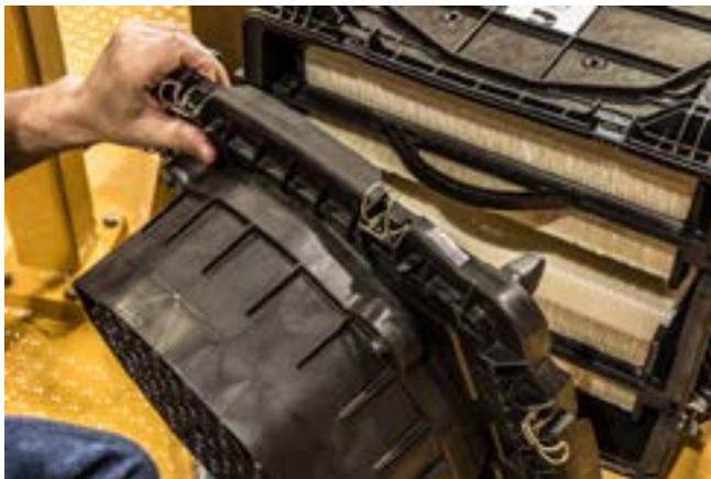
Figure 5-5-21 Remove Service Cover
