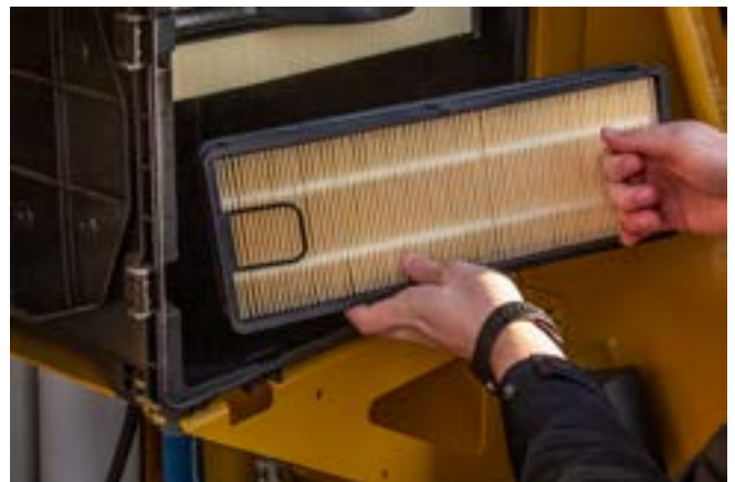
Figure 5-5-23 Remove Secondary Elements
