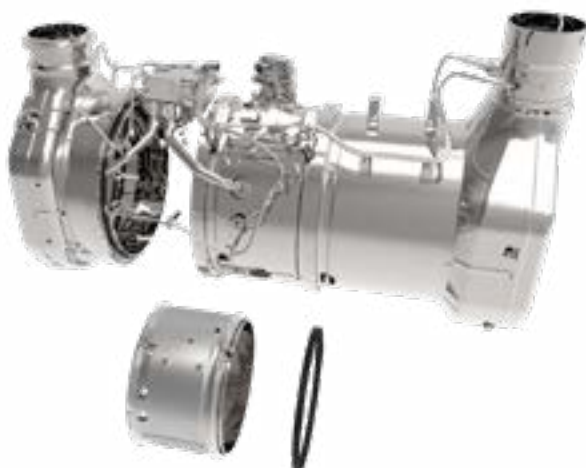
Figure 5-5-27 Detaching Diesel Particulate Filter
