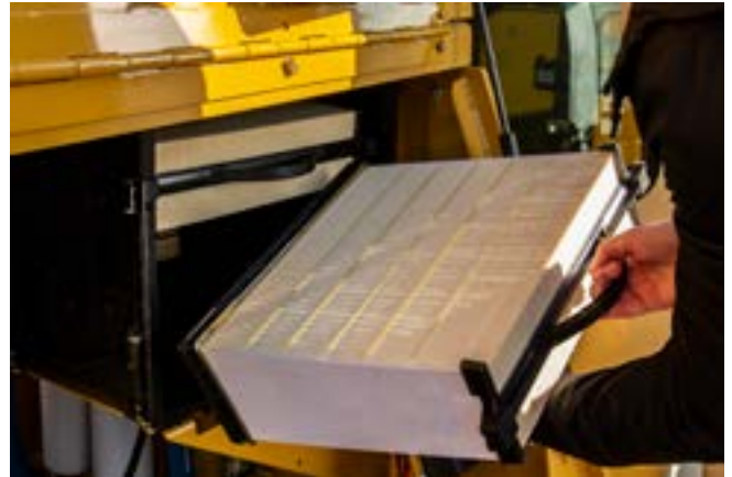
Figure 5-5-22 Remove Primary Elements
