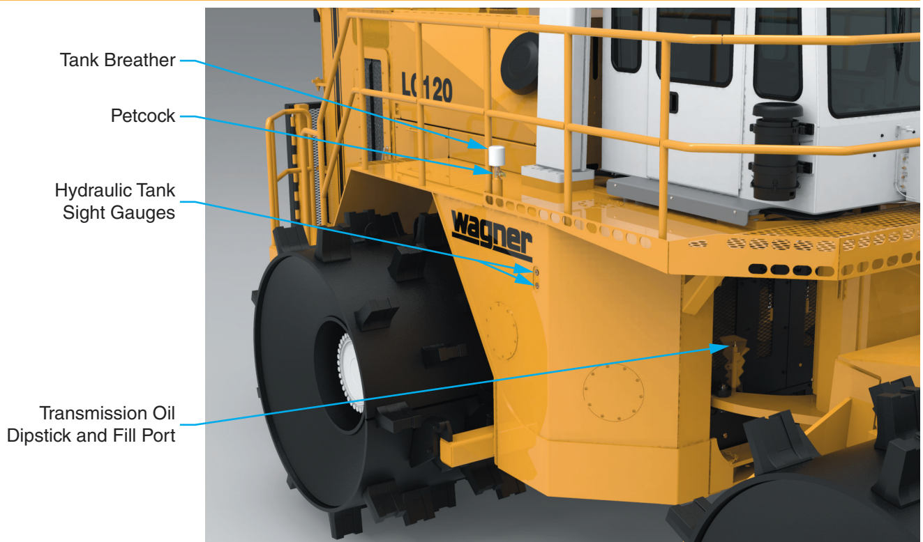
Figure 4-2-5 Hydraulic Oil and Transmission Oil Maintenance Locations
