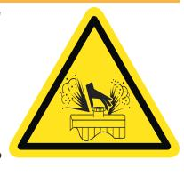
remove the radiator cap only when the engine is cool.
