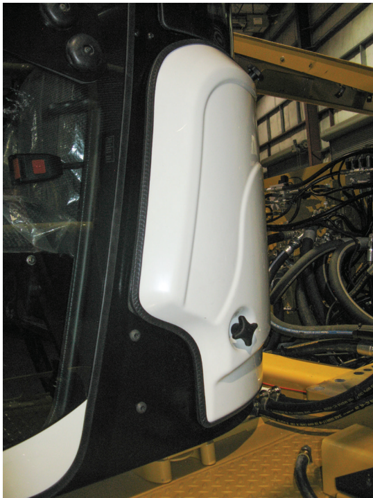
Figure 5-5-21 Cab Air Intake Filter Location
