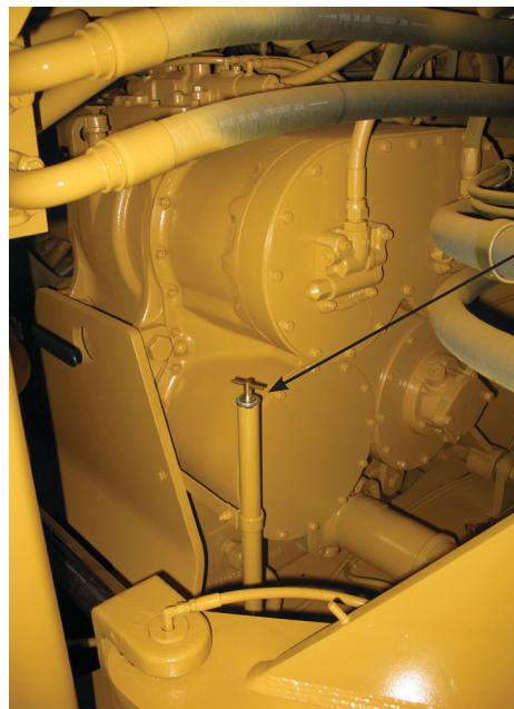
Figure 5-4-1-8 Transmission Oil Dipstick and Fill
