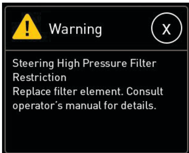
Figure 5-4-1-9 Hydraulic Filter Warning (example)
