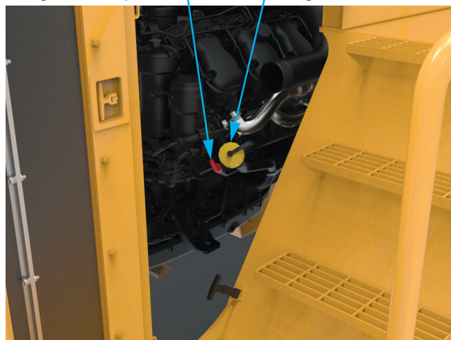
Figure 4-2-2 Engine Oil Maintenance Points
