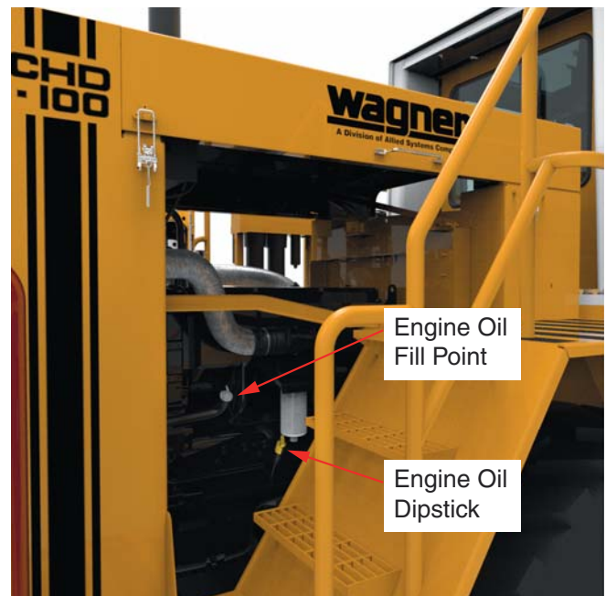
Figure 4-2-2 Engine Oil Maintenance Points
