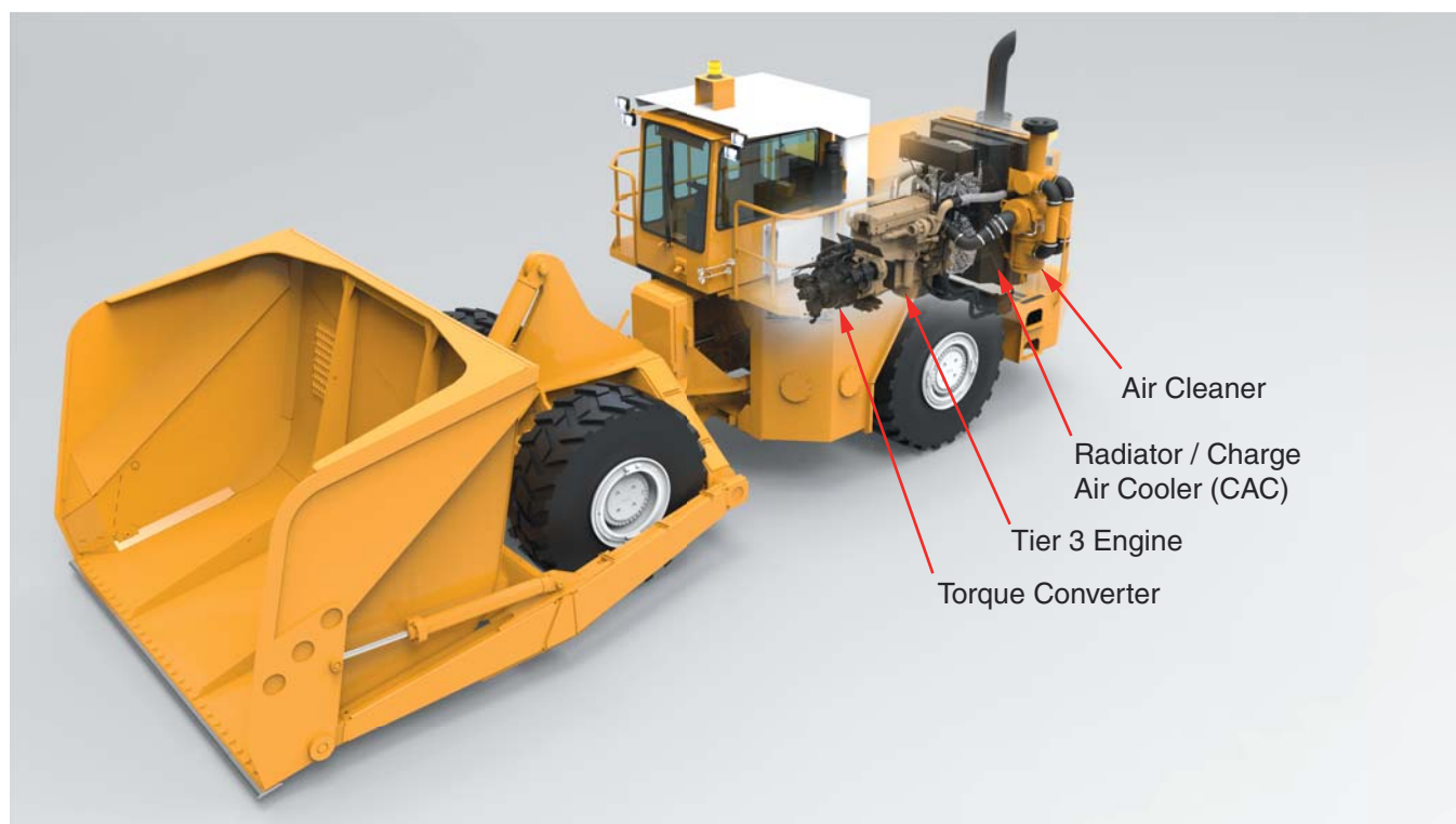
Figure 3-1-1 Power Unit (Model CHD100 with Cummins Tier 3 Engine Shown)
