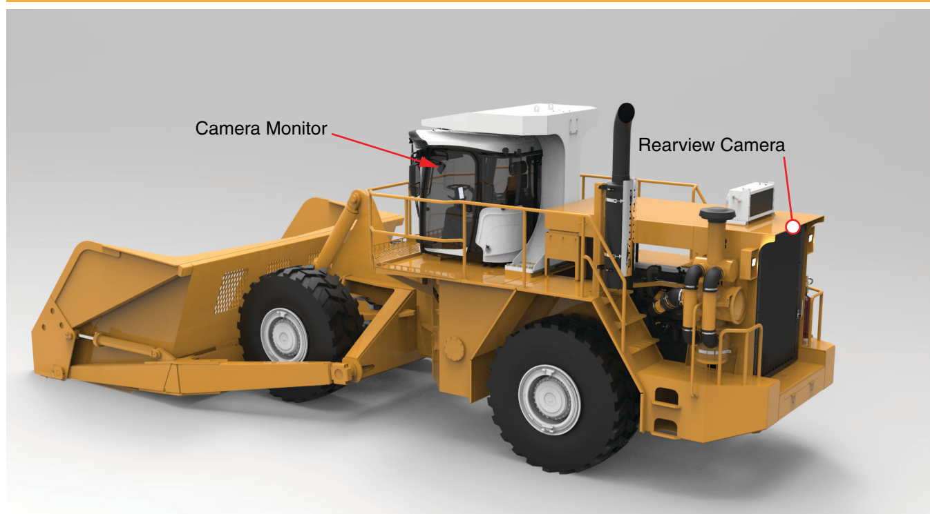
Figure 2-9-1 Cameras and Monitor Locations
