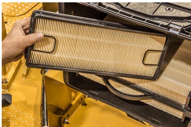
Figure 5-5-12 Remove Secondary Elements
