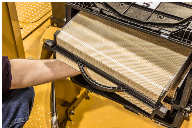
Figure 5-5-11 Remove Primary Elements
