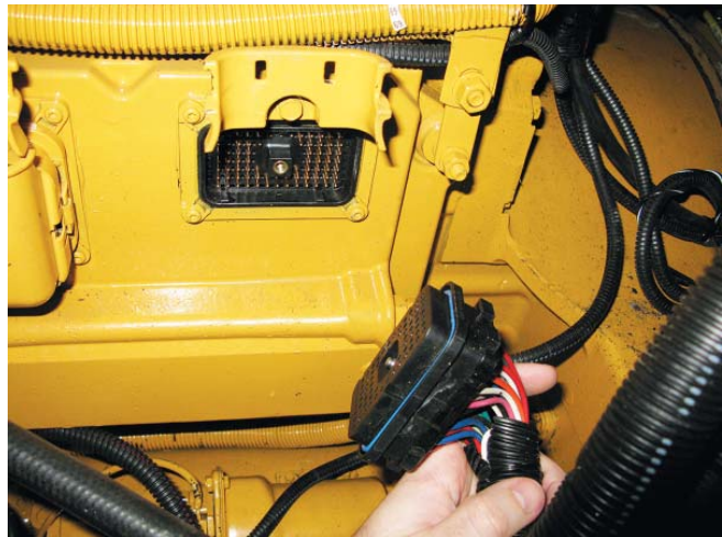
Figure 5-1-2 Disconnect ECM(Electronic Control Module)
