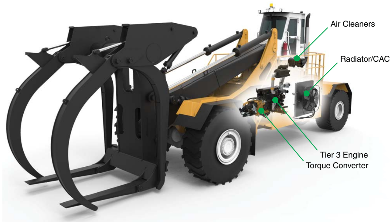
Figure 3-1-1 Power Unit (Model L490 with Cummins Tier 3 Engine Shown)
