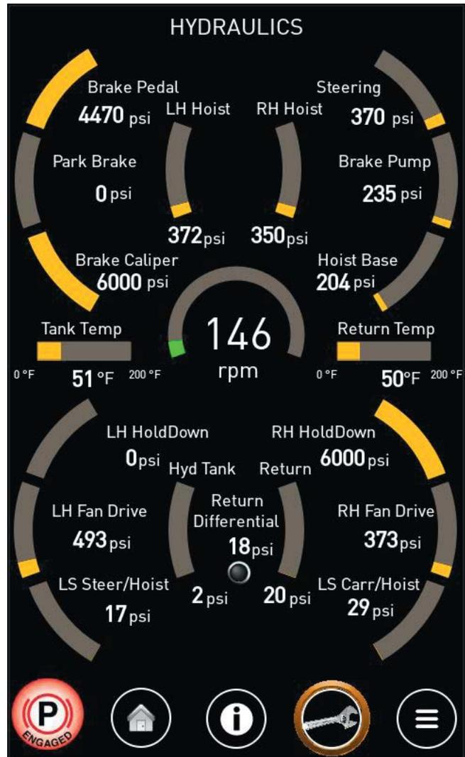
Figure 2-2-9 Hydraulics Screen
