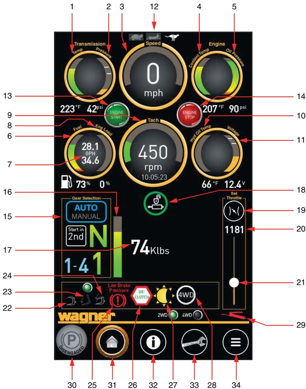
Figure 2-2-2 Home Screen, Smart Screen Operator Interface
