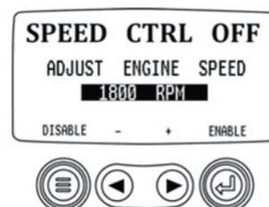
**NOTE: Once enabled Engine Speed Control will stay enabled even through power cycles. To turn OFF, you must disable the feature from the SPEED CTRL screen.**
