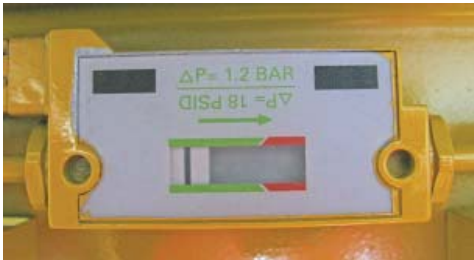
Figure 6-28 Differential Pressure Indicator
