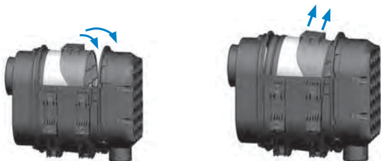
Figure 6-12 Remove Primary Filter
