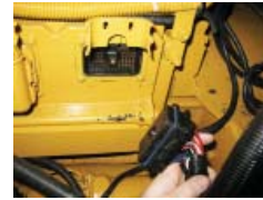
Figure 6-3 ECM (Electronic Control Module)
