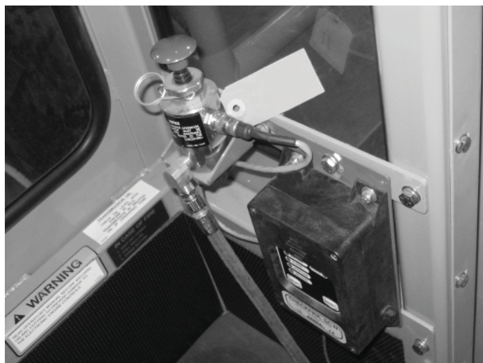
Figure 3-18 Fire Suppression System. Shown with Automatic Detection and Activation System
