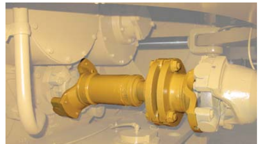
Figure 5-7 Front driveline assembly with shear bolts
