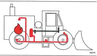
**4.** Dry chemical extinguishing agent is discharged through fixed nozzles into protected areas, suppressing the fire.
