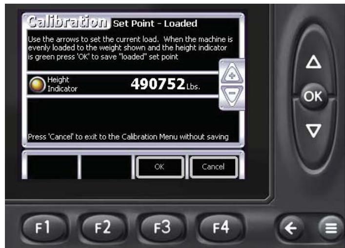
Figure 8 - Calibrate Loaded Screen
