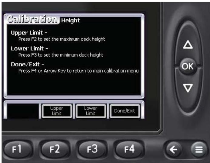
Figure 10 - Calibrate Height Menu Screen
