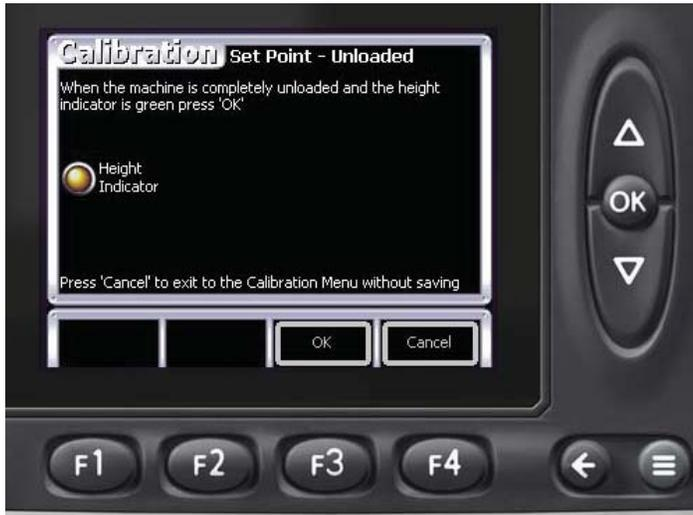
Figure 9 - Calibrate Unloaded Screen
