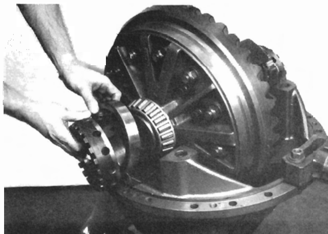
Figure 7 Remove adjusting nuts and taper bearing cups.
