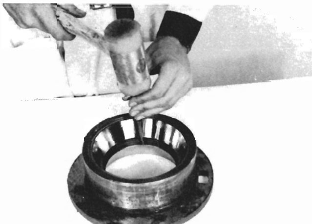
Figure 19 Remove pinion bearing cups only if they are to be replaced or if the bearing cage is damaged.
