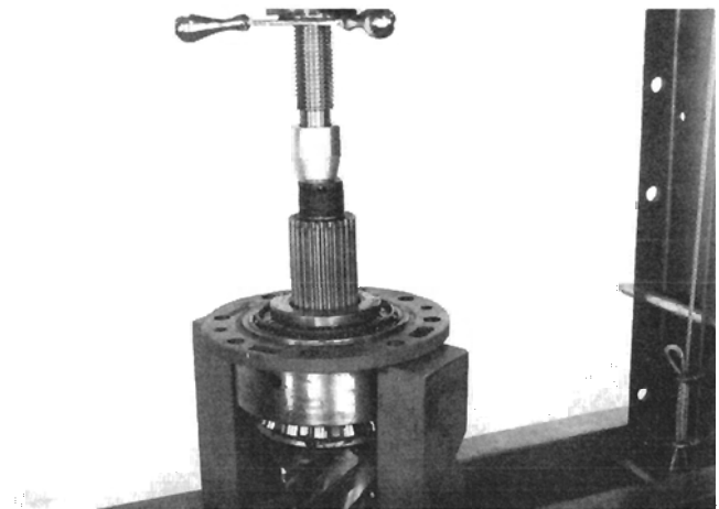
Figure 15 Press pinion shaft and center bearing from outer bearing and bearing cage.
