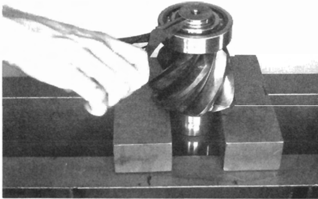
Figure 17 Remove inner pinion bearing retainer ring.
