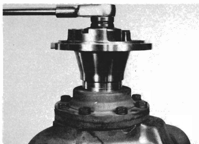
Figure 9 Remove companion flange nut.
