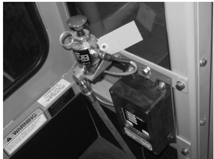
Fig. 3-18 Fire Suppression System Shown with Automatic Detection and Activation System
