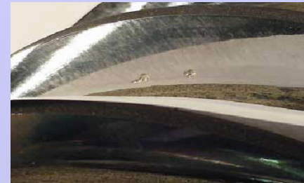
Pitting starting at SAP
