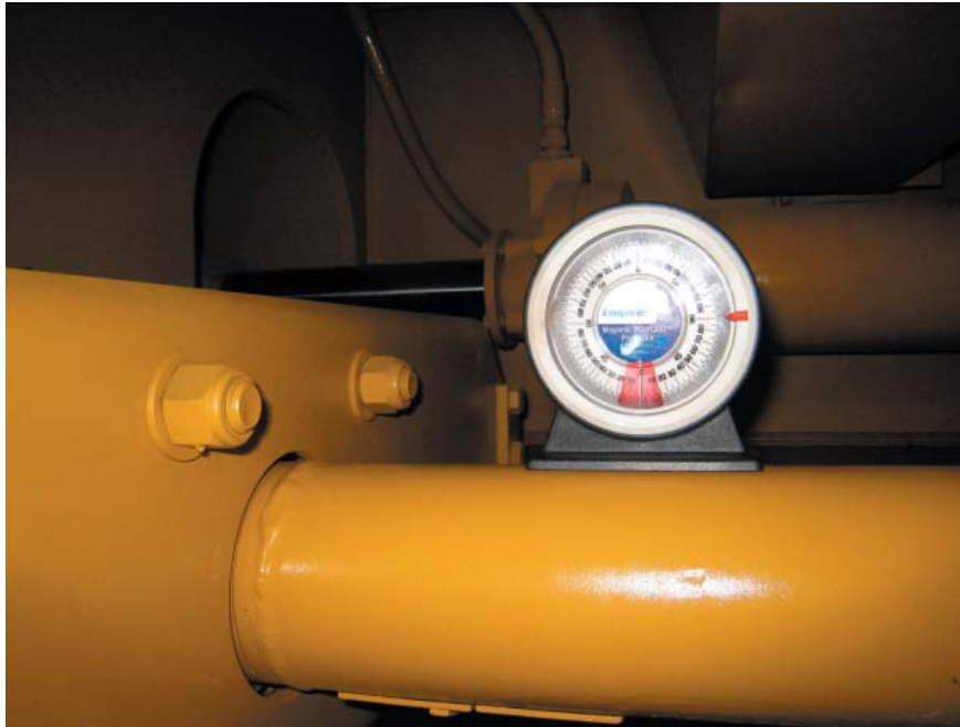
Figure 2: Using a magnetic angle detector to check driveline support is perpendicular to the center line of the driveline.
