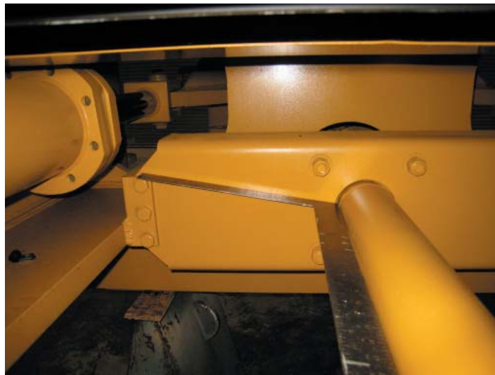
Figure 1: Using square to check driveline support is perpendicular to the center line of the driveline.
