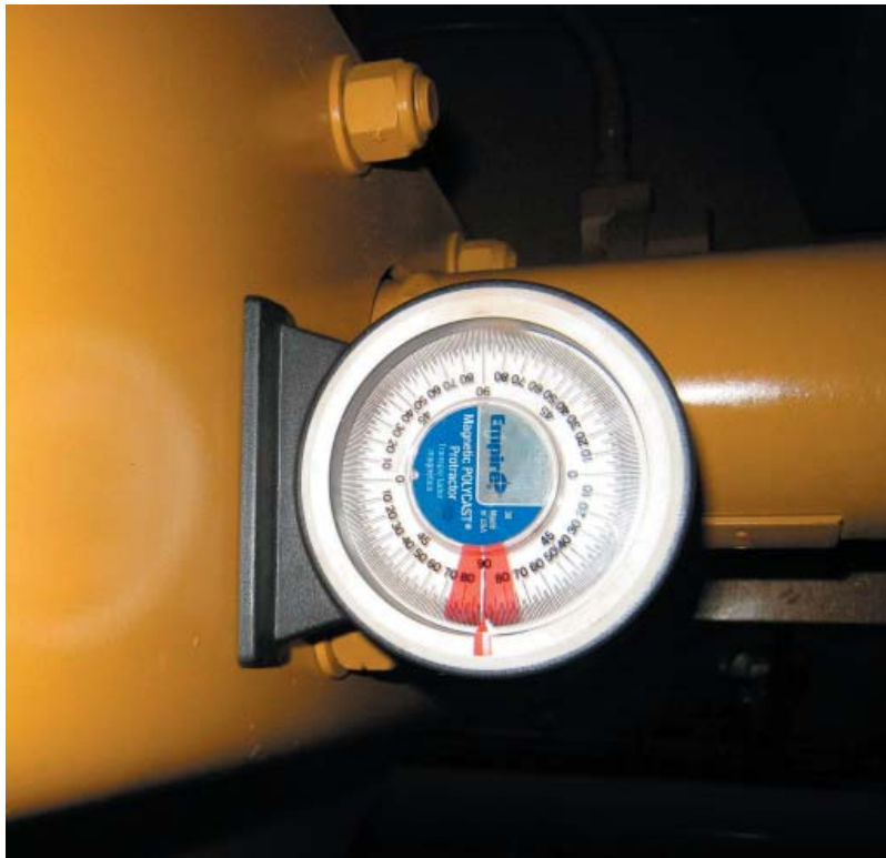
Figure 3: Using a magnetic angle detector to check driveline support is perpendicular to the center line of the driveline.
