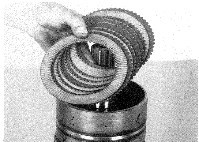
Figure 94 Remove inner and outer clutch discs.
