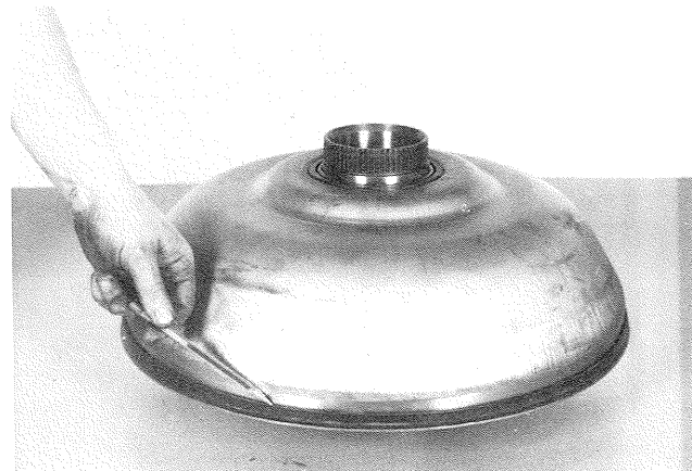
Figure 262 Install a new oil baffle oil seal ring on oil baffle. Position oil baffle on impeller assembly.
