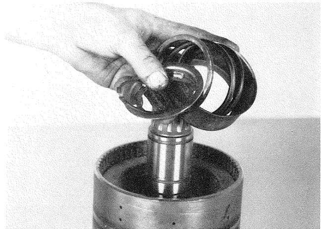
Figure 93 Remove piston return spring and inner and outer spring retainers.
