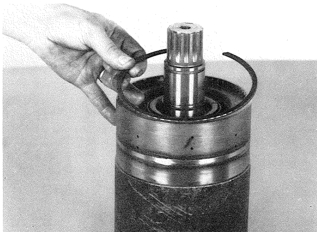
Figure 90 Remove end plate retainer ring.
