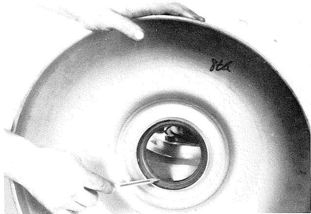
Figure 261 Apply a light coat of Loctite 638 to the outer diameter of the oil baffle oil seal. Press oil seal in oil baffle with lip of seal down.
