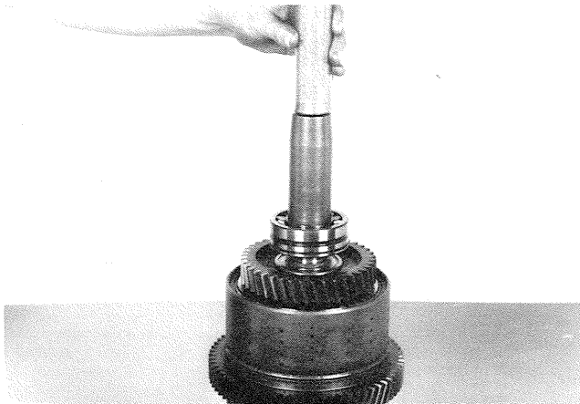
Figure 180 Install clutch shaft front bearing. NOTE: Bearing outer retainer ring groove must be down.
