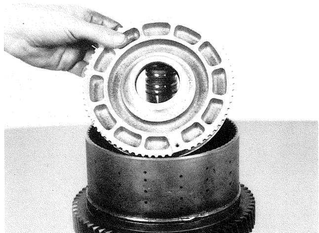
Figure 124 Remove clutch piston.
