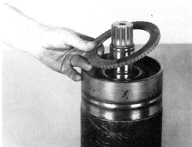
Figure 91 Remove end plate.
