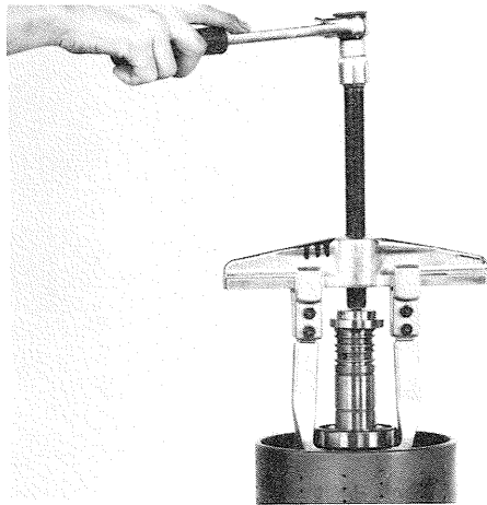
Figure 43 Remove clutch gear inner bearing.
