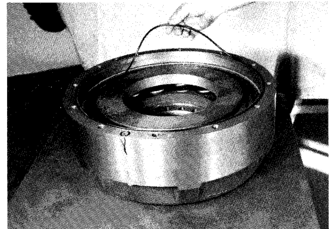
Figure 18 Install outer cover "O" ring seal.
