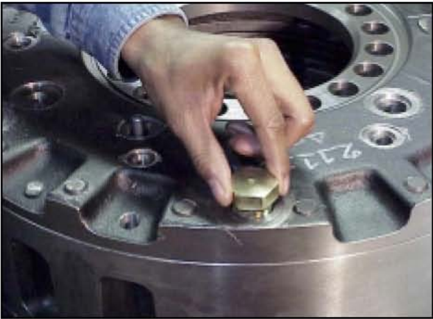
Figure 11 Remove the cooling port plugs or fittings.
