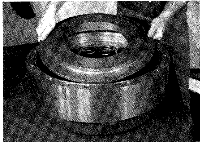
Figure 16 Install piston pressure ring.
