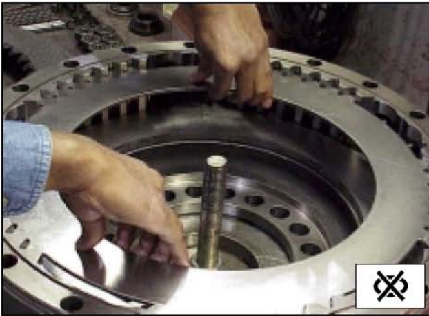
Figure 31 Install reaction plate over pressure plate.
