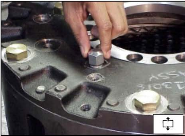
Figure 8 Remove the cap from the wear indicator.
