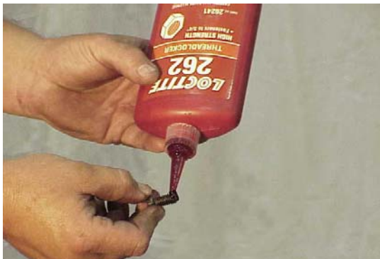
Apply Loctite 262 or equivalent to lock plate screws. Tighten to 25–28 lbf/ft [34–38 Nm].
