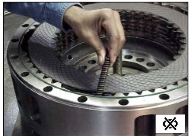
Figure 35 Install retractor springs over guide pins.
