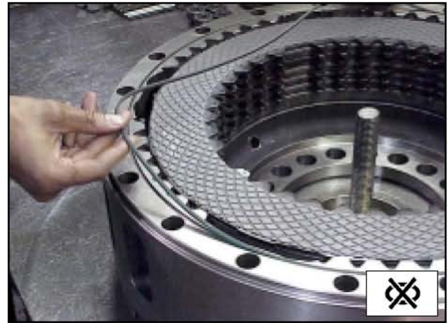
Figure 34 Install cover seal O-ring in groove.
