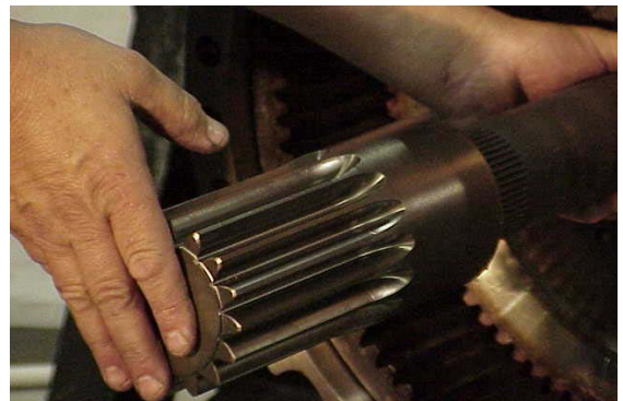
Install axle shaft and sun gear.
