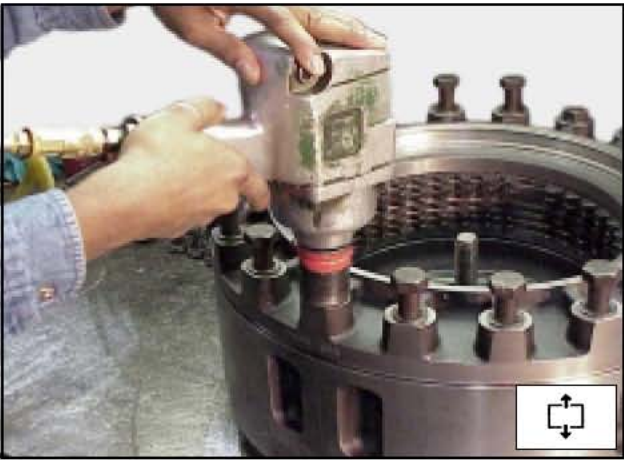
Figure 12 Remove the cover capscrews.
