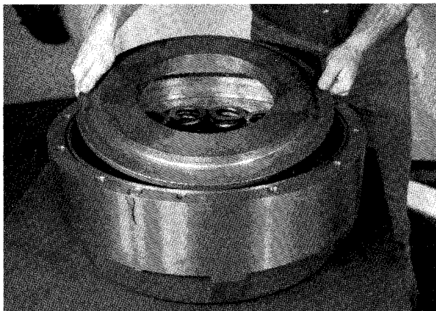
Figure 11 Remove piston pressure ring.
