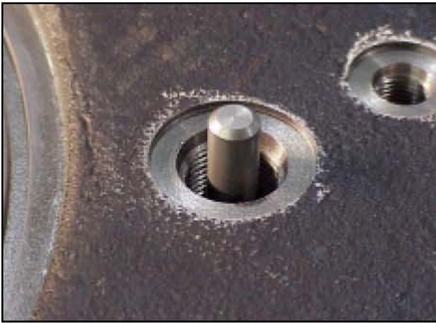
Figure 9 Wear indicator pin.
