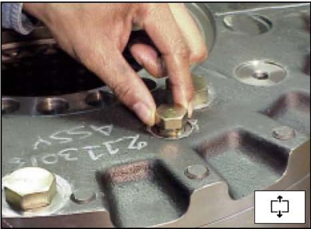
Figure 10 Remove the piston inlet port fittings or plugs.
