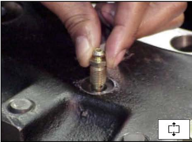
Figure 7 Remove the bleeder screw.
