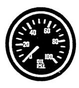
Fig. 3-6 Engine Oil Pressure Gauge
