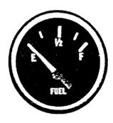
Fig. 3-4 Fuel Level Gauge
