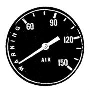
Fig. 3-10 Air Pressure Gauge
