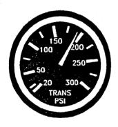
Fig. 3-8 Transmission Circuit Pressure Gauge
