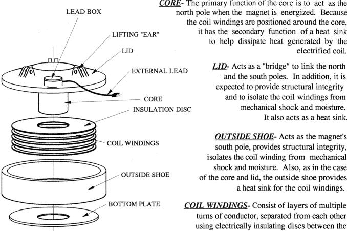
CORE- The primary function of the core is to act as the north pole when the magnet is energized. Because the coil windings are positioned around the core, it has the secondary function of a heat sink to help dissipate heat generated by the electrified coil.
