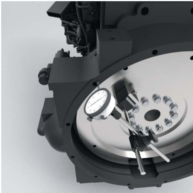
Figure 1 Face Runout of Flywheel Housing
