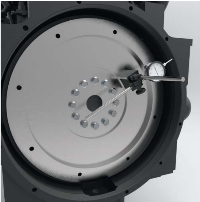
Figure 3 Bore Runout of the Flywheel Housing
