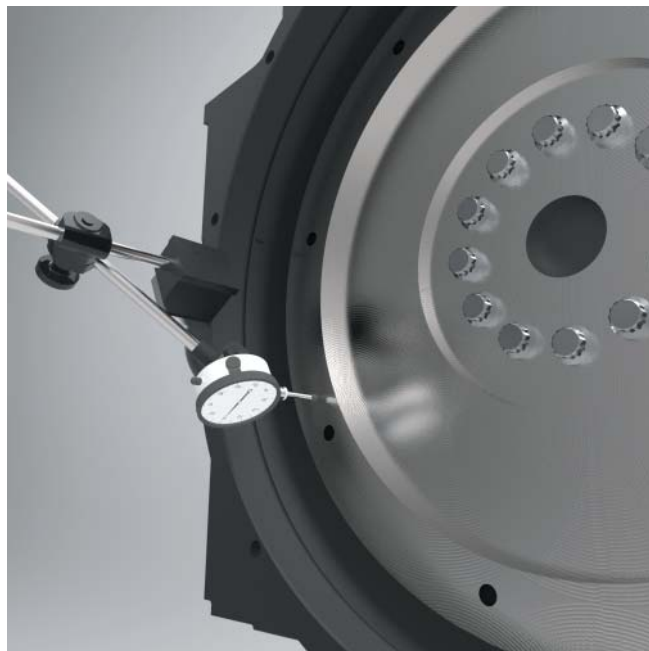
Figure 6 Face Runout of the Flywheel
