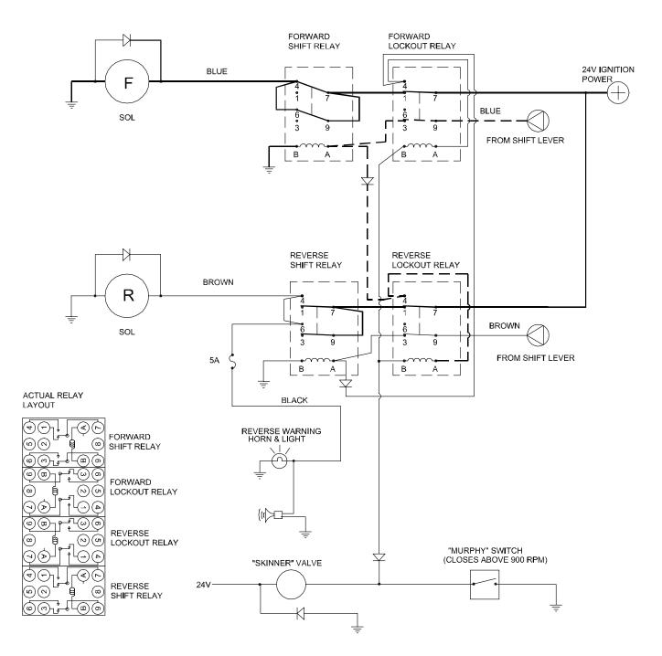
Shifting to "neutral" or "reverse" on the shift lever merely removes power to the relay coil, breaking the power to the forward solenoid. (The diode at the forward solenoid acts as a voltage-spike suppressor.)
