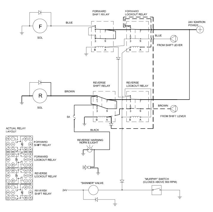
Again, shifting out of reverse merely stops power to the relay coil, allowing the contacts to open and cutting off power to the reverse solenoid.
