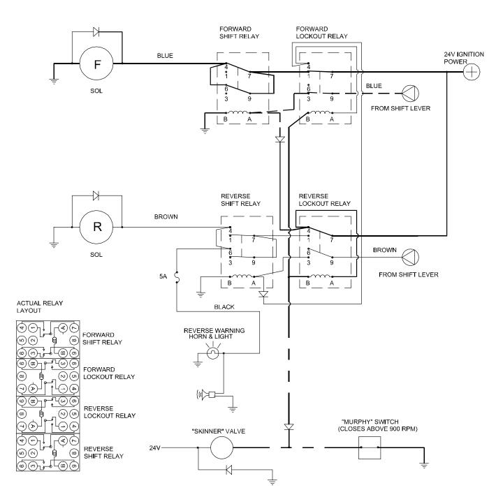
This lockout relay opens the reverse solenoid circuit, anbd this relay *holds* itself open until the engine speed goes below 900 rpm.
