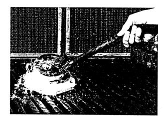
Use of compressed air will both speed drying and ensure removal of small abrasive and metal particles.
