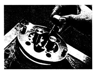
3. Remove the center housing (25) from adapter (7). Lay the pump on its side while holding onto the housing. Use a soft head hammer to tap on the ends of the drive and driven shafts (the ends that were in the cover). Do not use a screw driver or wedge to pry apart the separate sections. This will damage the machined sealing surfaces.
