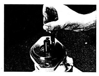
18. **Install the pipe plug (8)** in the adapter (7). Note: When pump is used as a motor in series, remove pipe plug and install a small external drain line.
