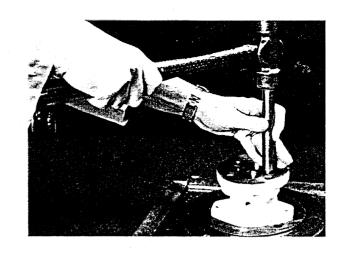
Sub assemble bushing (9) by installing O-ring (11) towards counterbore and inserting back-up ring (10) next to the O-ring (away from the counter bore). Lubricate exposed O-ring and back-up ring to prevent cutting them on installation.
