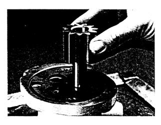
Install the second snap ring (22A). Install driven gear (23) in the adapter.
