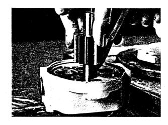
6. Bearings should be examined for evidence of spalling of rollers and fracture of stamped cages. Check roughness of outer race by sliding rollers around periphery of cage. If bearings were not removed, bearing condition can be checked by seeing if rollers move smoothly and easily with finger pressure. Any bearing showing excessive wear or other damage will need to be replaced.
