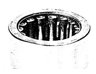
7. Check inside of housing (25) for visible signs of wear. Typically, housing wear will match gear teeth wear, and if gear assemblies require replacement, so will the housing.
