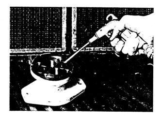
As with disassembly instructions, check the shaft number of the pump you are working on. Alternate procedures are listed for pumps with shaft numbers 50, 51, 52, 53 and 54.
