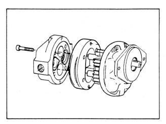
In Hydreco gear pumps, slippage is minimized by controlled clearance between the gear teeth and gear housing bores and minimum running clearance between the face of the gears and the wear plates.
