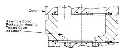
14. Install the cover and housing assembly onto the adapter (7). Don't forget to have the high pressure pockets of the wear plates positioned 180° opposite of each other. Note that the wear plate in the cover (29) can still be rotated even with the housing attached.
