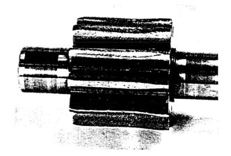
c. Edges of gear teeth have developed ridges.
