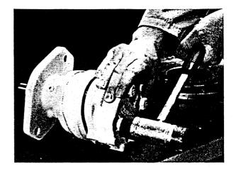
IMPORTANT: Keep the gears meshed together until they have been marked to ensure replacement in the same position.
