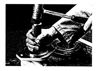
Remove adapter from the fixture and install snap ring (5).
