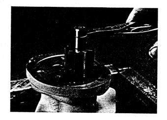
If using original gears, make sure to align marks made during disassembly.
