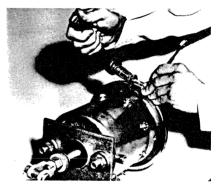
3 Note location of pressure plate inlet port with respect to spring chamber. Loosen clamp band nuts and bolts and remove clamp band halves.
