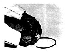
**13** Remove felt wiper ring and O-Ring from piston.
