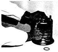
1 Install nylon bushing in cylinder center boss groove. Bushing must be installed so that side with bevel edge faces toward inside of cylinder. Lubricate and install small O-Ring in other groove.
