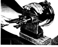
2 Mount the unit on 90° bracket and secure with stud nuts.
