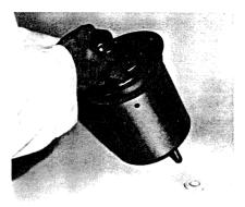
3 Insert piston assembly all the way into cylinder, holding felt wiper ring in place as piston is inserted.
