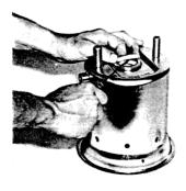
14 Remove O-Ring and nylon bushing from cylinder center boss. Use a sharp pointed instrument to remove bushing; work clockwise from cut to pry bushing out of groove; then remove backup ring.
