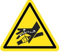
Relieve all hydraulic pressure before disconnecting any hydraulic line.
