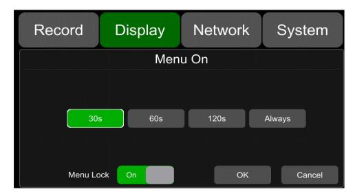
**Menu lock:** Menu on duration can be set to 30s, 60s, 120s, and Always. When set to 30s, 60s, or 120s, that is, after opening the menu, if there is no operation in 30s, 60s, or 120s, the menu will be hidden. When it is set to always, the menu will always be open.
