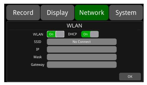
WLAN: ON/OFF status of WLAN
