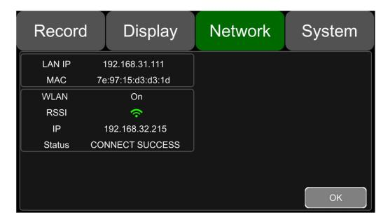
LAN IP: Static IP or automatically obtained dynamic IP
