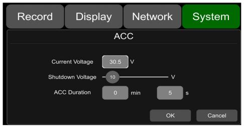
The default configuration of "Shutdown Voltage" and "ACC Duration" is shown above.
