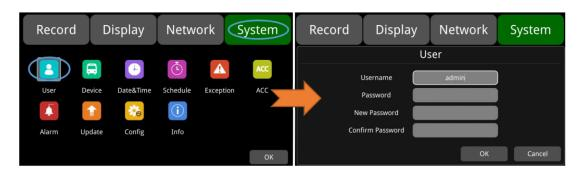
• Username admin and password are required to change the menu lock status. Below figure shows how to change the menu lock status from "on" to "off".
