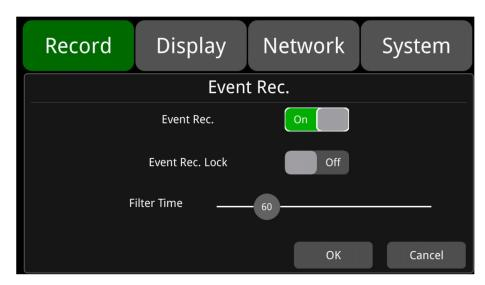
**Event recording:** Types of event recording include acceleration sensor triggered alarms and 1-5 triggered alarms. If event recording is on and the alarm parameters are set, the event recording will be triggered when the above event occur. If event recording is off, even if the event occurs, it will not trigger event recording. This feature is set on by default.
