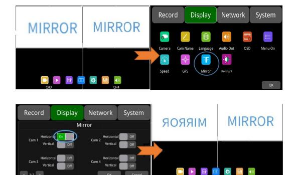
**Vertical:** when it is set to ON, the corresponding recording channel will flip vertically; when it is set to OFF, there will be no flip. Below are setting steps.
