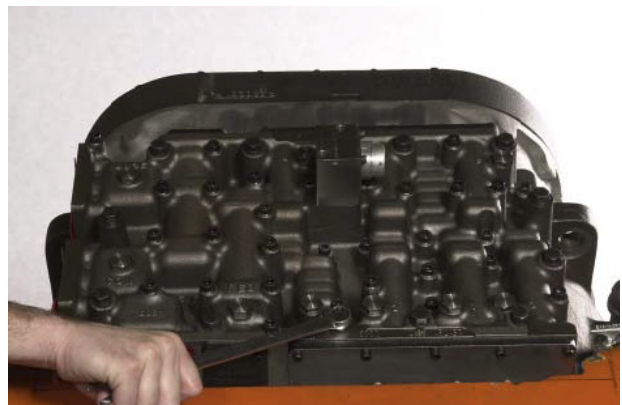
FIGURE 5: Remove control valve bolts and lockwashers.
