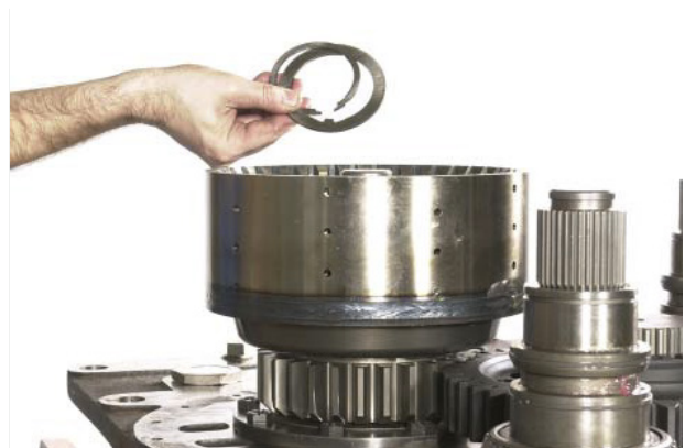
FIGURE 92: Install keyed washer and washer retaining snap ring.
