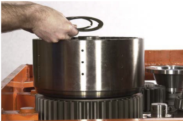
FIGURE 124: Install bearing washer and bearing snap ring.
