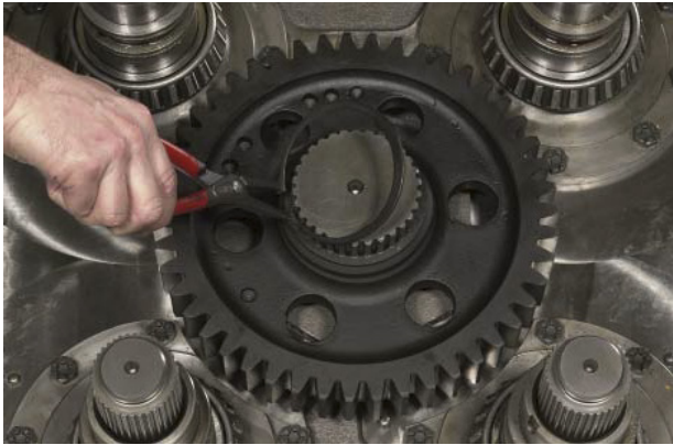
FIGURE 89: Install idler gear retaining snap ring.
