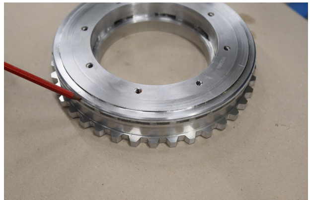
FIGURE 15: Install clutch piston ring and expander after assembly apply grease on piston ring
