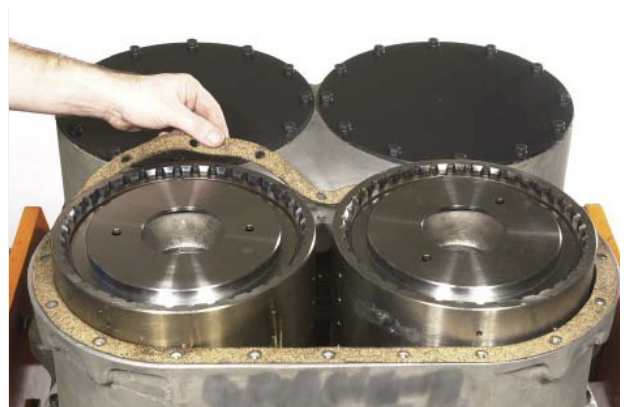
FIGURE 104: Install new gasket.
