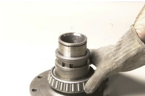
FIGURE 72: Warm bearing cone to 120° C [248° F] and install on clutch support.
