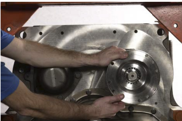
FIGURE 8: Remove input flange.
