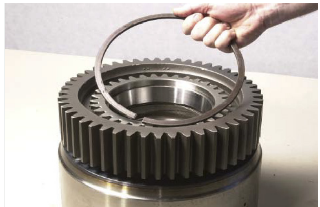
FIGURE 69: Instal clutch hub gear retaining snapping.
