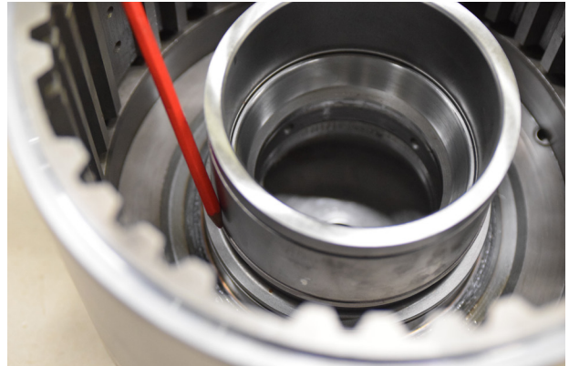
FIGURE 14: install clutch piston ring and expander after assembly apply grease after assembly apply grease on piston ring
