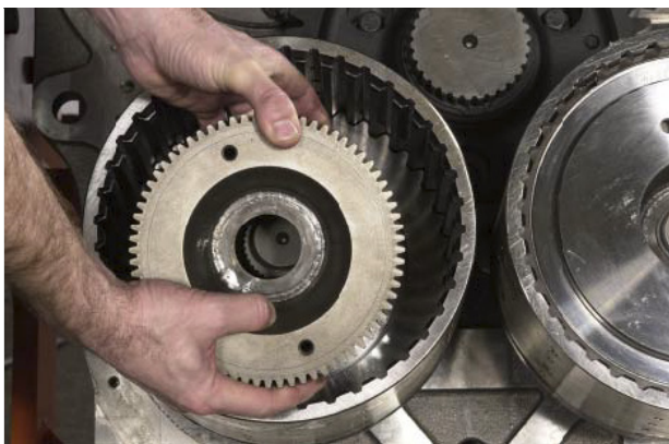
FIGURE 37: Remove clutch disc hub.
