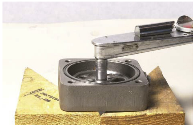
FIGURE 141: Install bolt and torque to specified torque.
