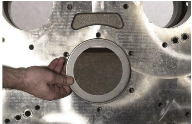
FIGURE 77: Install oil shield.
