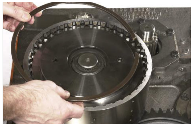
FIGURE 98: Install end plate retaining snapring.
