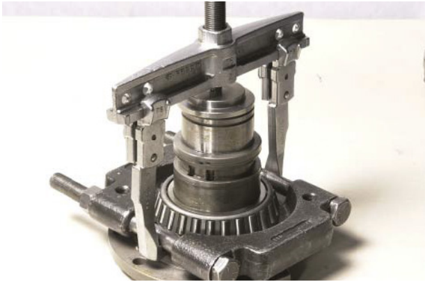
FIGURE 70: Remove clutch support bearing cone.
