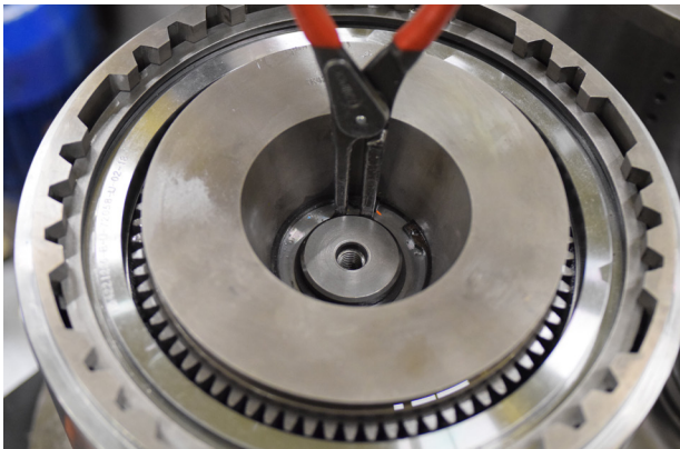
FIGURE 1: Remove clutch hub snap ring
