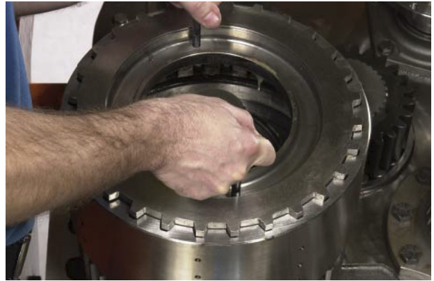
FIGURE 125: Install clutch piston.
