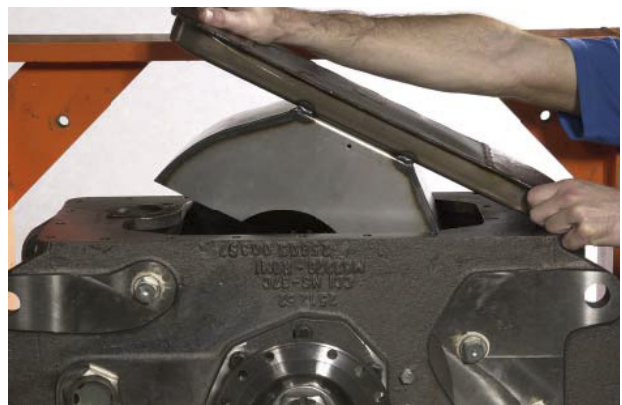
FIGURE 4: Remove oil sump frame and screen.
