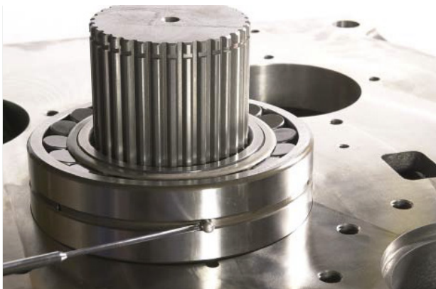
FIGURE 80: From the other side install idler shaft and bearings as an assembly.
