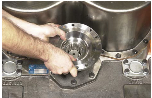
FIGURE 147: Install output flange.
