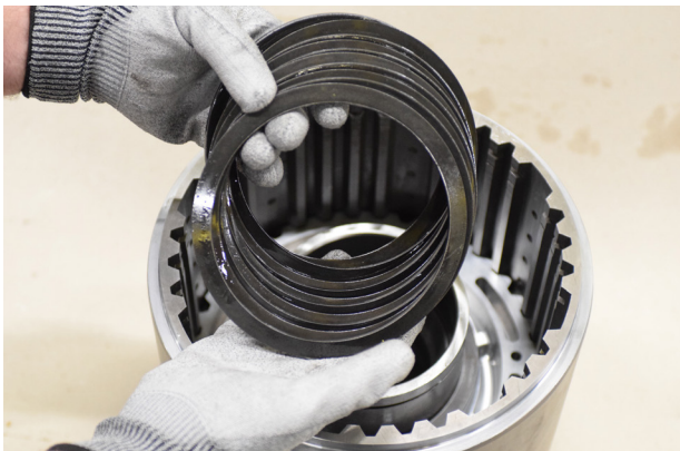
FIGURE 18: Install belleville springs washers (10).
