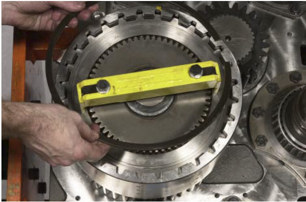
FIGURE 132: Use special tool to press end plate down and install end plate retaining ring.
