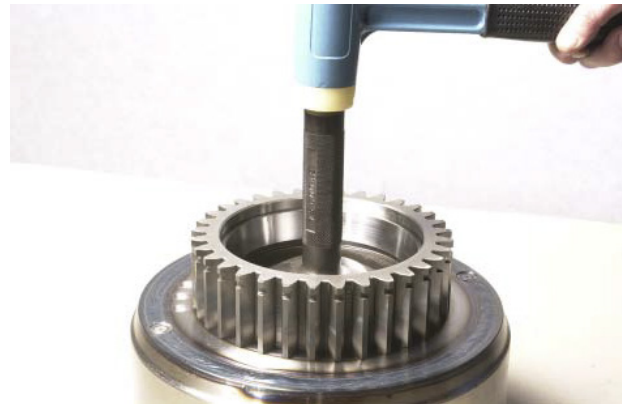
FIGURE 56: Remove piston ring outer race and outer support bearing cup.
