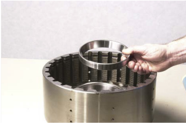
FIGURE 65: Install clutch inner bearing cup.
