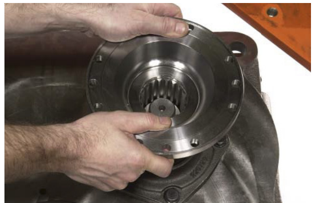
FIGURE 116: Install input flange.
