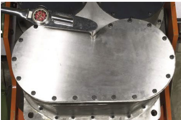
FIGURE 107: Place cover, lockwashers and bolts and torque to half the specified torque.
