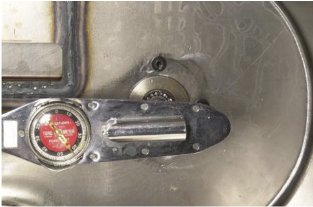
FIGURE 143: Install sealing washers and bolts. Torque to specified torque.
