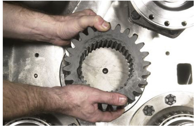
FIGURE 120: Install idler gear.
