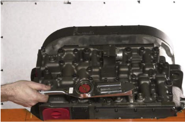
FIGURE 155: Install screws and torque to specified torque.
