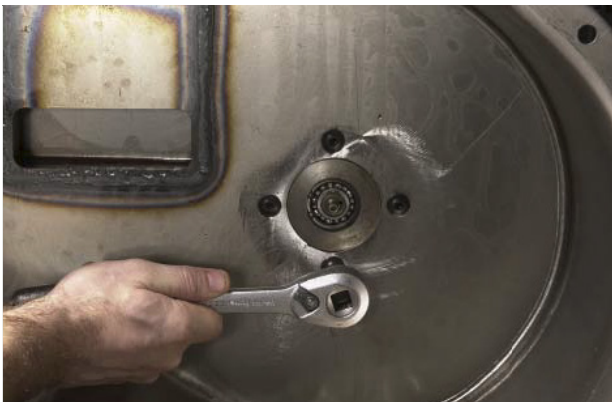
FIGURE 134: Speed drive housing to case screws and sealing washers and gently tap speed drive housing from cover.
