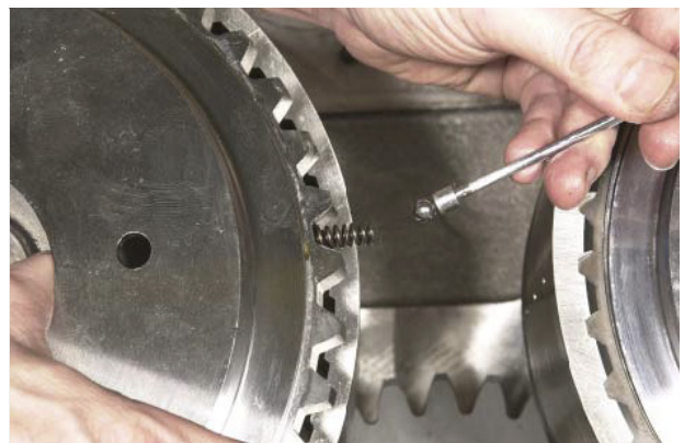
FIGURE 35: Locating ball and spring on either side of the end plate.
