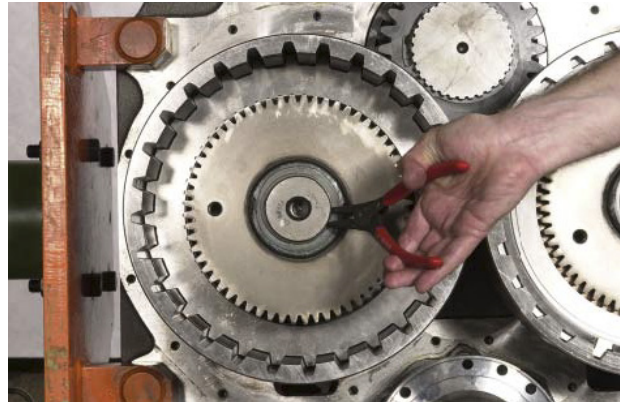
FIGURE 14: Remove clutch disc hub retaining ring.
