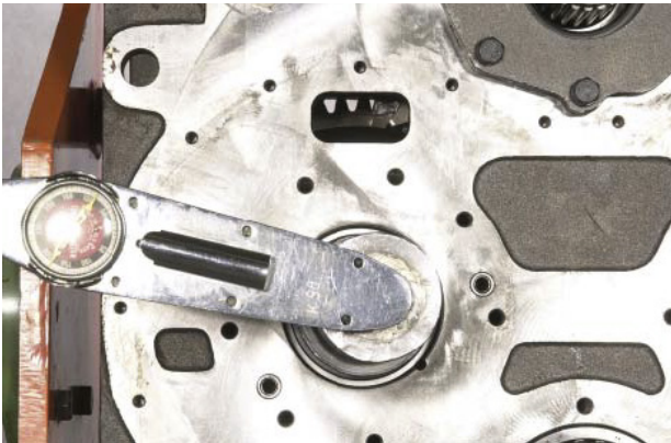
FIGURE 85: Torque to specified torque
