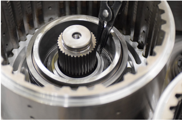
FIGURE 6: Open clutch support snap ring
