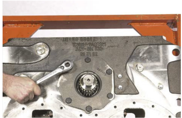
FIGURE 43: Remove rear output flange bearing cap.
