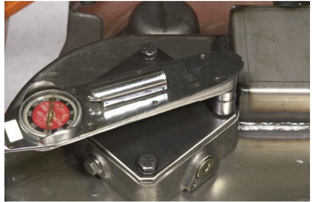
FIGURE 146: Install gasket and speed drive cover. Place bolts and torque to specified torque.
