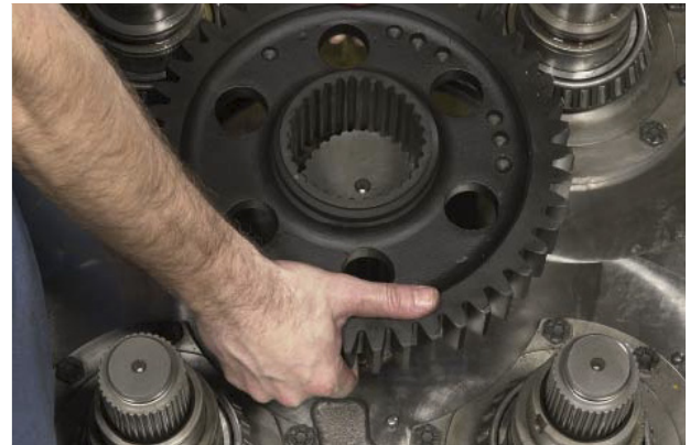
FIGURE 88: Install idler gear
