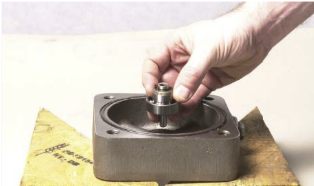
FIGURE 138: Install speedo drive axle and bearing.
