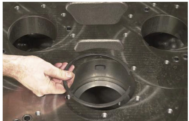
FIGURE 78: Install bearing locating snap ring.
