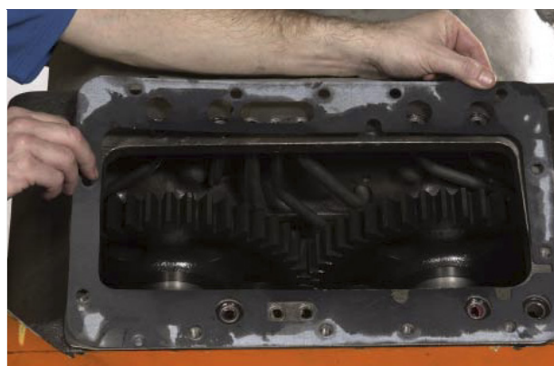
FIGURE 154: Install new control valve to transmission case gasket.
