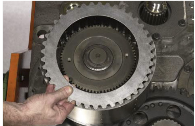
FIGURE 96: Install one outer clutch plate. Alternate friction and clutch plates till proper amount is reached.
