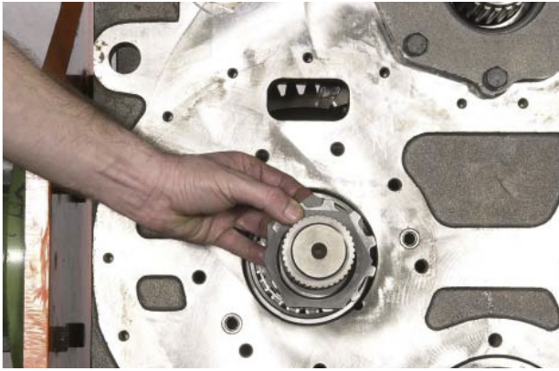
FIGURE 84: Install clutch drum shafts & gears. Install bearing lock nut, nut lock and lock nut.
