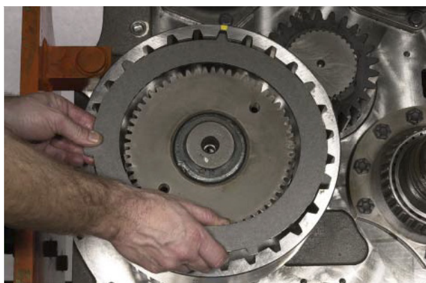
FIGURE 128: Install outer disc.
