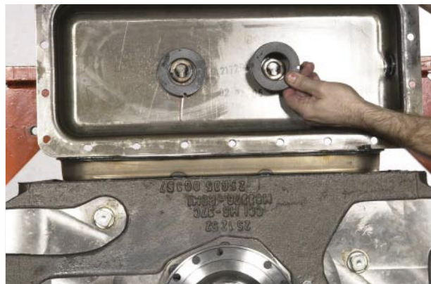
FIGURE 152: Clean and replace magnets in oil sump.
