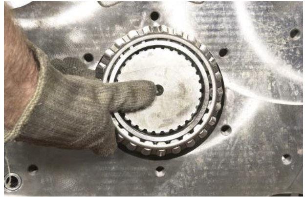
FIGURE 81: Warm idler shaft bearing cone to 120° C [248° F] and install on idler shaft. Install 2nd bearing in the same manner. See figure below for installation sequence.
