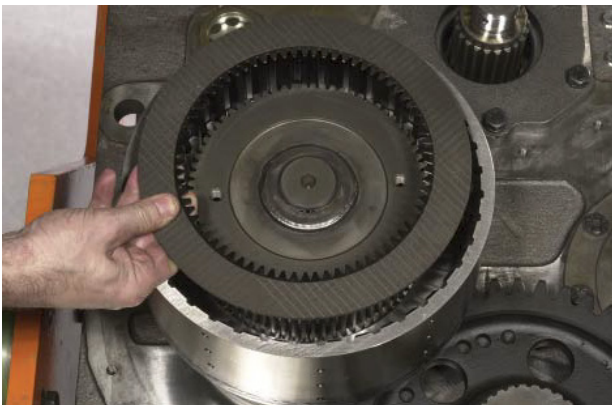
FIGURE 95: Install one friction plate.
