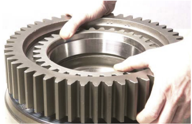
FIGURE 68: Install clutch hub gear.
