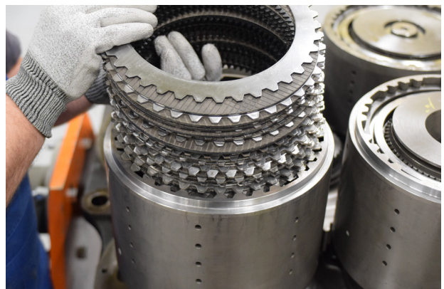
FIGURE 28: Install clutch patch, clutch pack shims. It is purchased as a pack
