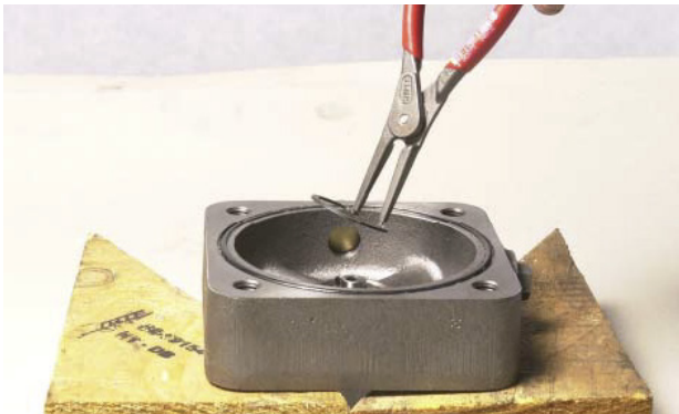
FIGURE 139: Install bearing locating snapring.
