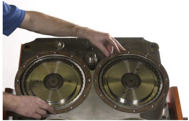
FIGURE 102: Install 2 new gaskets
