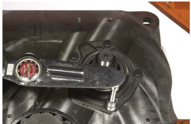
FIGURE 115: Install lockwashers and bolts and torque to specified torque.
