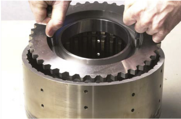
FIGURE 59: Use 2 bolts to remove clutch piston.
