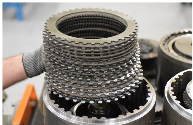
FIGURE 5: Remove clutch pack steel and friction disc's
