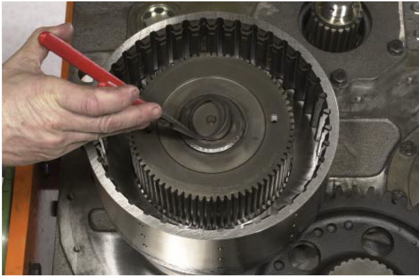
FIGURE 94: Install disc hub retaining ring.
