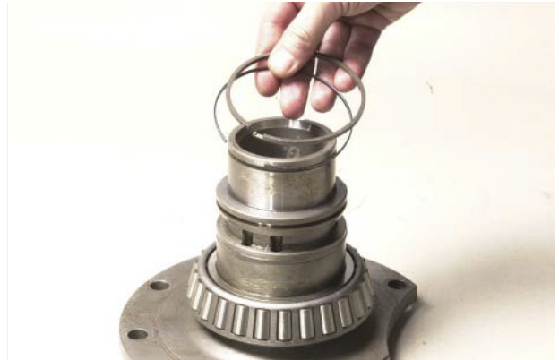
FIGURE 73: Install clutch support piston rings.
