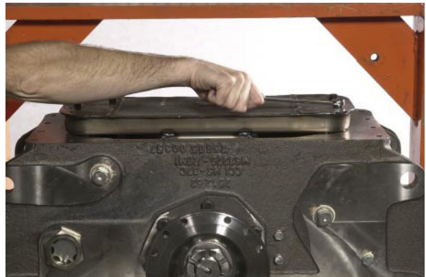
FIGURE 3: Remove oil screen bolts and lockwashers.
