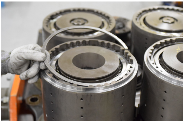
FIGURE 30: Install end plate snap ring.
