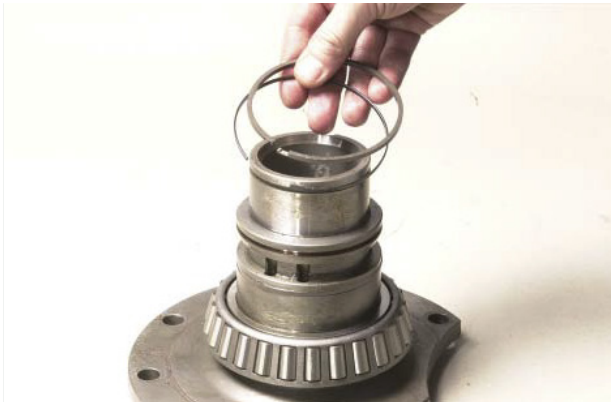
FIGURE 71: Remove clutch support piston rings.
