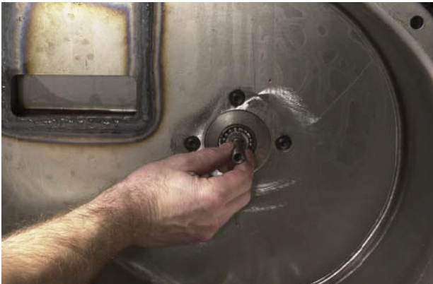
FIGURE 133: Remove speed drive spring.
