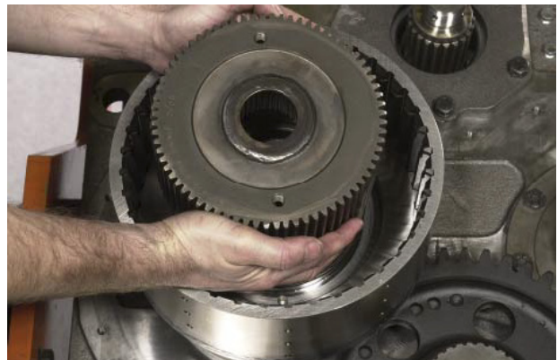
FIGURE 93: Install disc hub.
