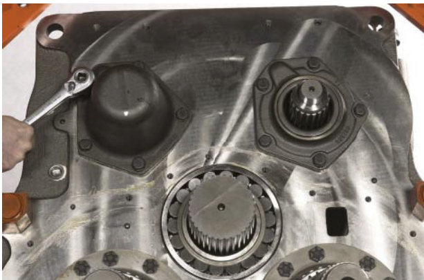
FIGURE 25: Remove reverse shaft bearing cap.
