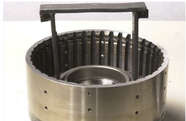
FIGURE 57: Press return springs and remove spring retaining snap ring.
