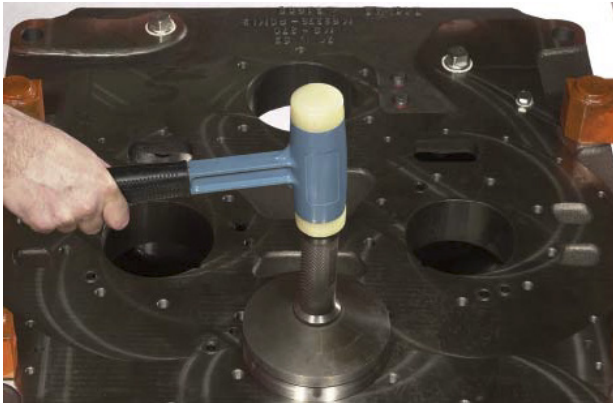
FIGURE 79: Tap idler shaft bearing cup into place.
