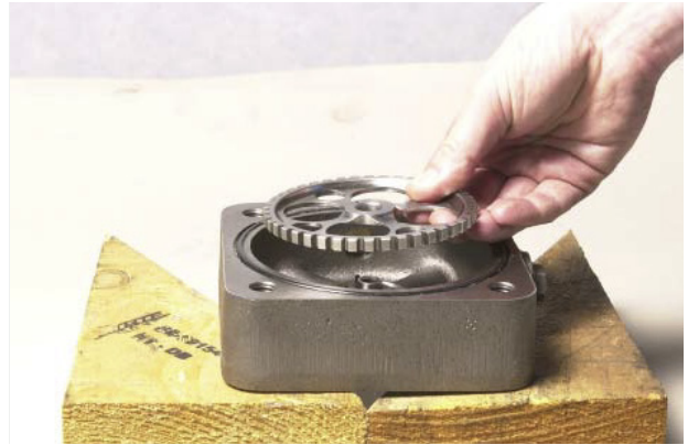
FIGURE 140: Install speedo drive gear.
