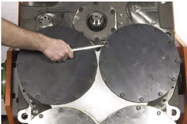
FIGURE 31: Remove forward, reverse, 3rd and 4th clutch cover bolts and lockwashers.
