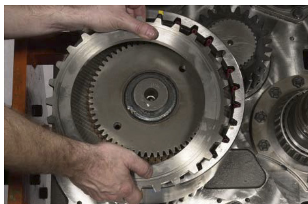
FIGURE 131: Install end plate.
