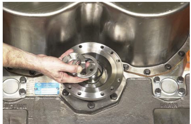
FIGURE 148: Install Flange o-ring, washer and lock nut.
