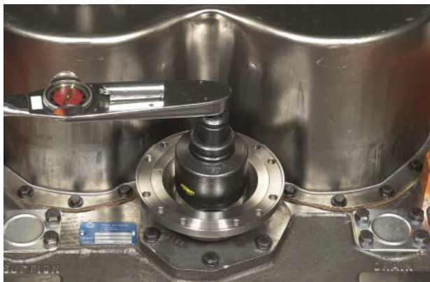
FIGURE 149: Torque nut to specified torque.
