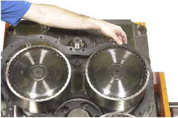
FIGURE 99: Install new gasket.
