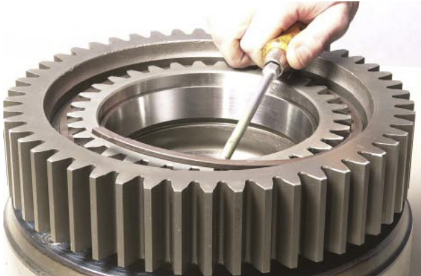
FIGURE 54: Use this procedure for all drums. Remove clutch hub gear snap ring.
