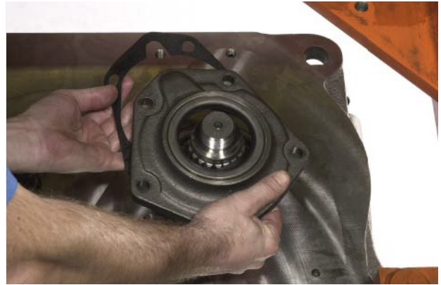
FIGURE 114: Install new gasket and input shaft bearing cap.
