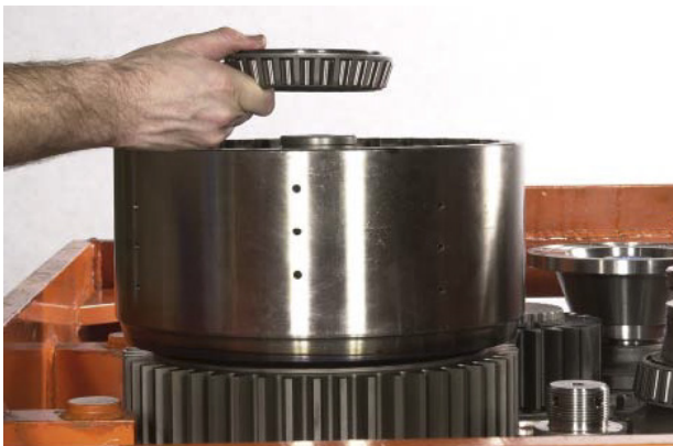
FIGURE 123: Install drum inner bearing cone.
