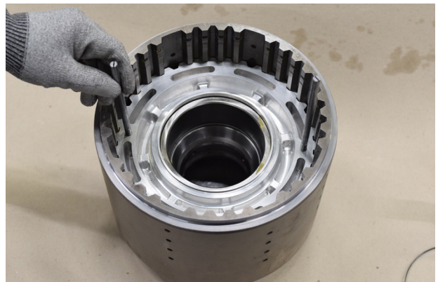
FIGURE 16: Install clutch piston assembly
