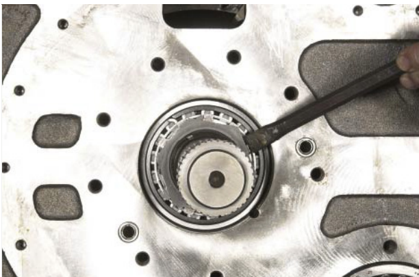
FIGURE 86: Secure nut loc by bending 2 lips.
