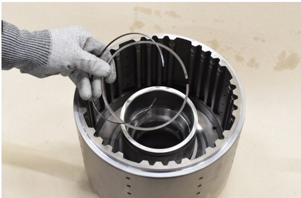
FIGURE 13: Remove clutch piston ring and expander.
