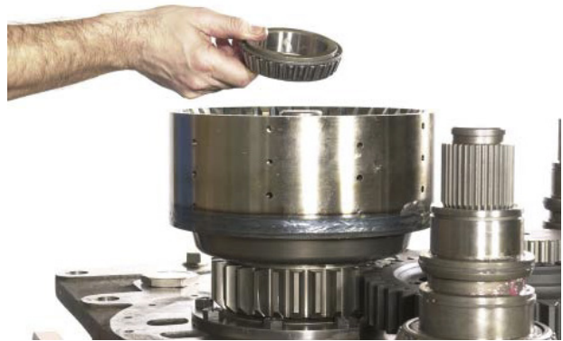
FIGURE 91: Install tapered roller bearing.
