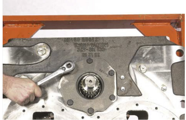
FIGURE 76: Install output shaft bearing cap bolts and lock-washers. See installation instruction for proper shim procedure.
