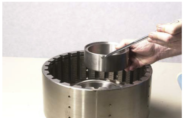
FIGURE 64: Install piston ring outer race and locking ball.
