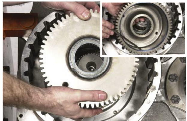
FIGURE 126: Install disc hub. Check that disc hub oil baffle ring is in place and intact. (See inset)
