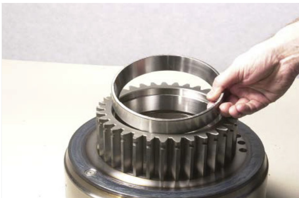
FIGURE 67: Install clutch outer bearing cup.
