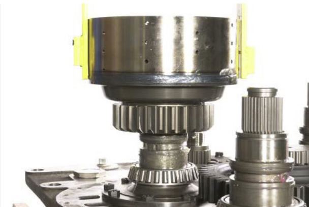
FIGURE 90: Install clutch drum on clutch drum support.
