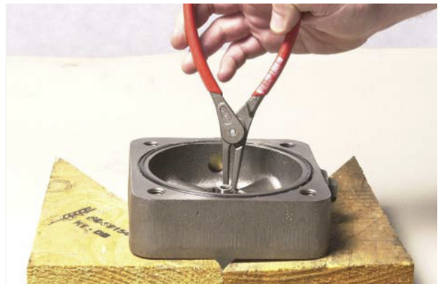
FIGURE 136: Remove speed bearing retaining snapring.
