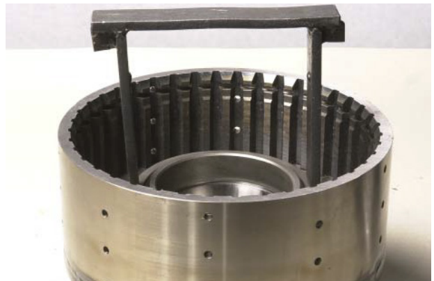
FIGURE 63: Install spring retaining snapping.
