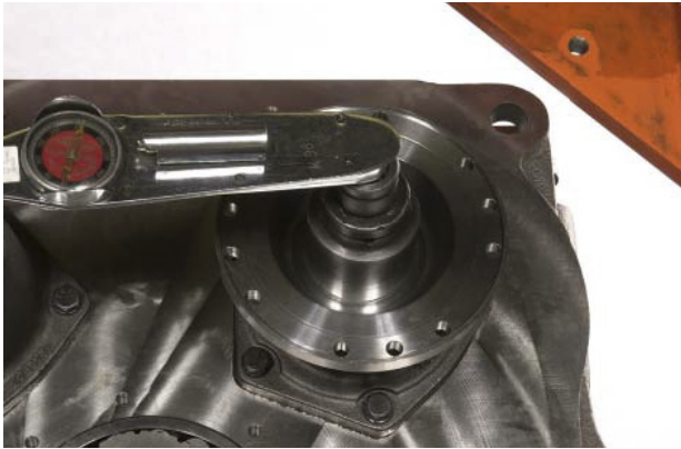
FIGURE 117: Install o-ring, washer and nut on input shaft and torque to specified torque.
