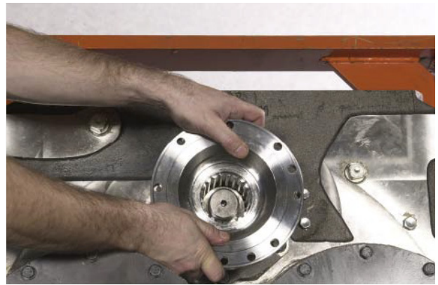
FIGURE 108: Install output flange on output shaft.
