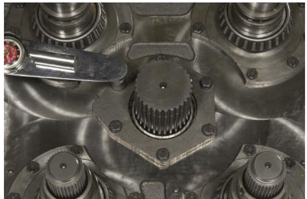
FIGURE 83: Install bearing cap and shims and torque bolts to specified torque. See installation instruction for shim procedure.
