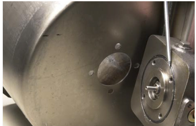
FIGURE 142: Install new seal and install speedo onto cover.
