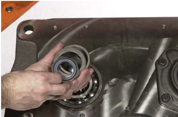
FIGURE 118: Install spacer, retainer and retaining nut on reverse shaft.
