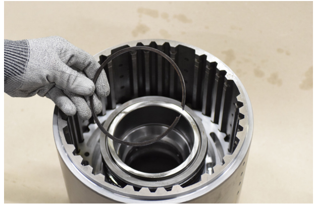
FIGURE 20: Install belleville springs washer snap ring
