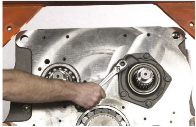
FIGURE 27: Remove input shaft bearing cap bolts, lockwashers and bearing cap. Remove bearing cap and oil seal.
