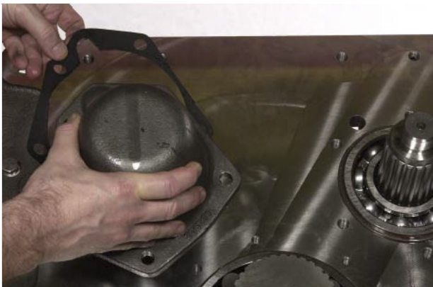
FIGURE 112: Install reverse shaft bearing cap gasket and bearing cap.
