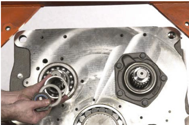
FIGURE 26: Remove reverse shaft nut washer and spacer.
