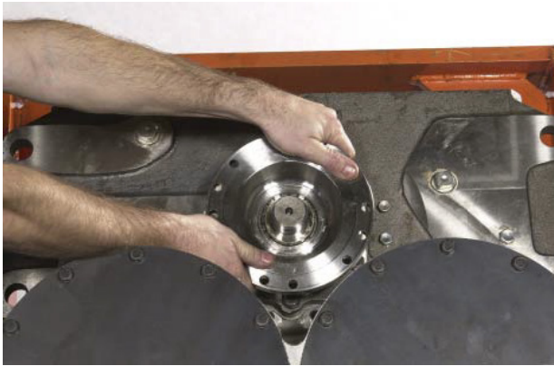
FIGURE 30: Remove output flange.
