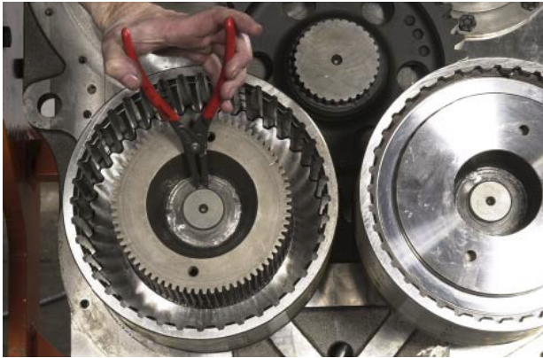
FIGURE 36: Remove clutch disc hub retaining snap ring.
