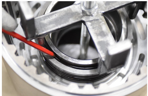
FIGURE 21: Install tool, compress belleville springs washers and install belleville springs washer snap ring into groove
