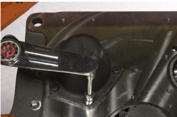
FIGURE 113: Place lockwashers and bolts and torque to specified torque.
