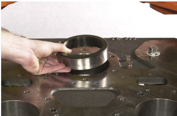
FIGURE 53: From other side remove bearing cup
