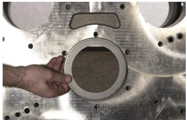
FIGURE 51: Remove oil shield.
