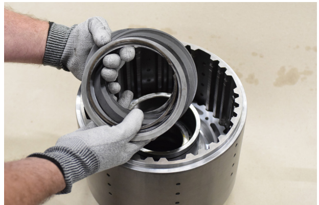
FIGURE 10: Remove belleville springs washer snap ring, spacer (2) and belleville springs washers (9)
