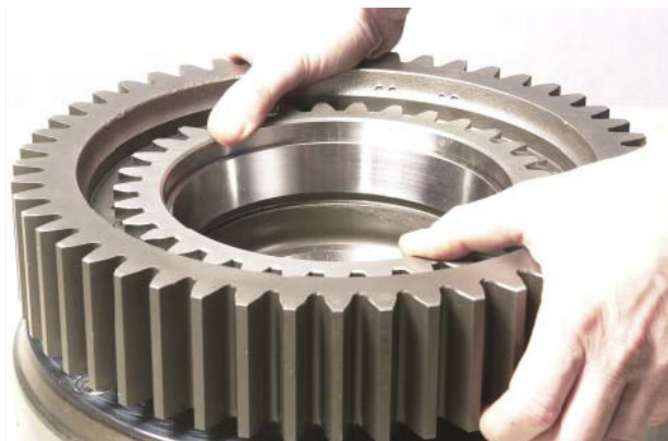
FIGURE 55: Remove clutch hub gear.
