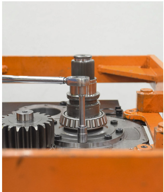
FIGURE 98: Tighten 8x cap screws to 80-88 ft-lbs (cap screws should be precoated, size \frac{3}{4} ).
