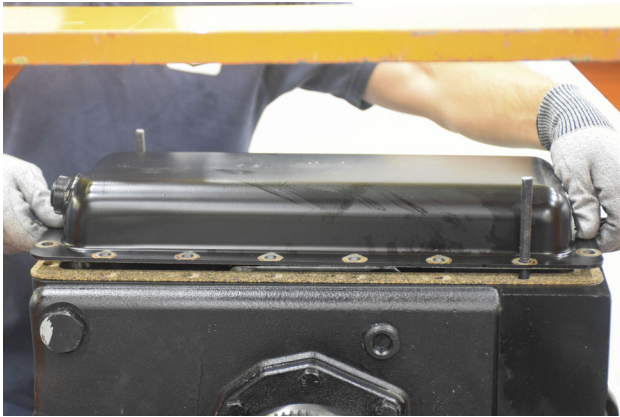
FIGURE 163: Install sump + sump magnets, use 2x guide pins.
