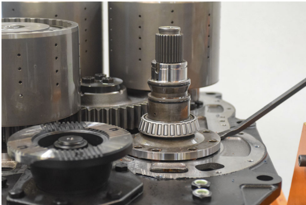
FIGURE 25: Remove clutch support-assembly.
