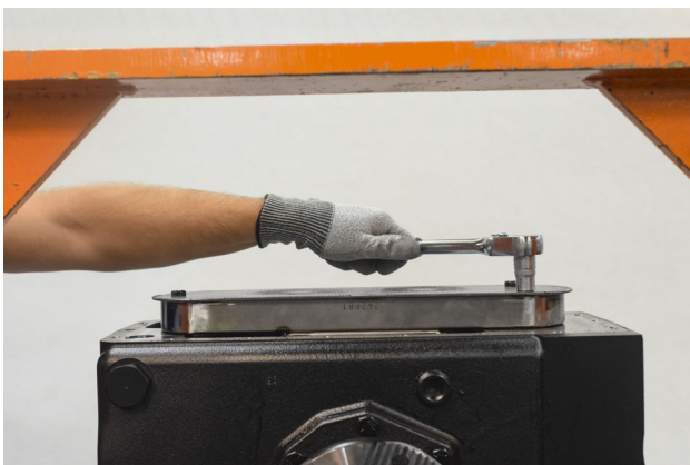
FIGURE 30: Remove 3x cap-screw (size 9/16).
