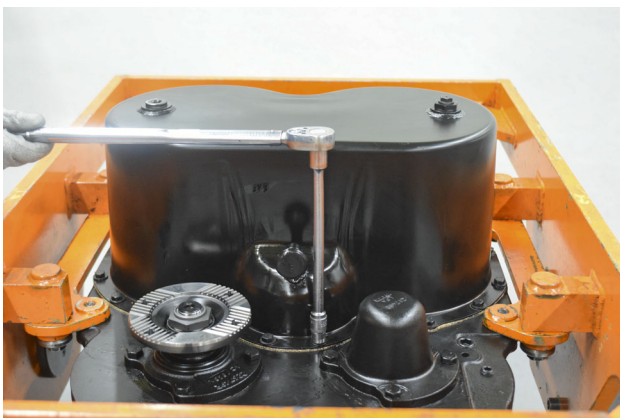
FIGURE 159: Install 20x cap screws + washers, torque to 23-25 ft·lbs (cap screws should be precoated, size 9/16).
