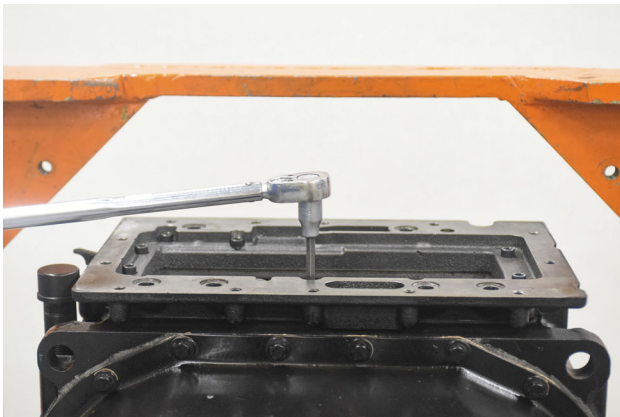
FIGURE 170: Install 12x cap screws, apply Loctite 243, torque to 41-46 ft-lbs (size 8).
