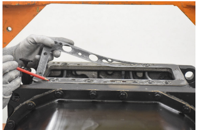
FIGURE 168: Install 6x O-rings + gasket.
