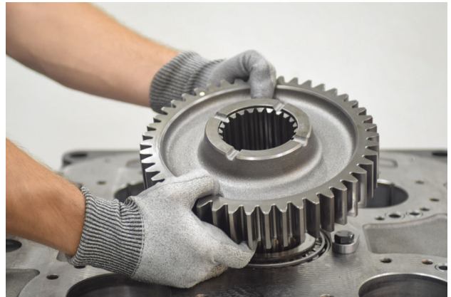
FIGURE 85: Install gear (groove on top).
