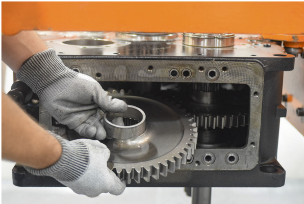
FIGURE 47: Remove gear and spacer.
