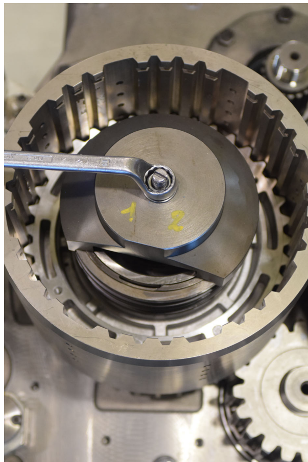
FIGURE 147: Using special tool AS0010012900 (see drawing AS0010012900 p. 153), push Belleville washers down and install snapping in position.
