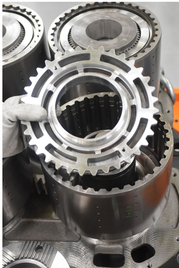
FIGURE 22: Remove piston, use two guide pins.
