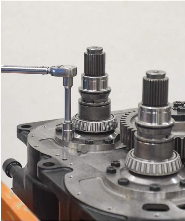
FIGURE 119: Tighten 8x cap screws to 80-88 ft-lbs (cap screws should be precoated, size 3/4).
