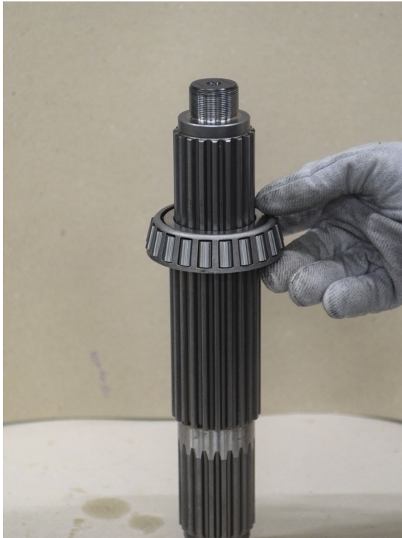
FIGURE 122: Install bearing (heat to 120°C).
