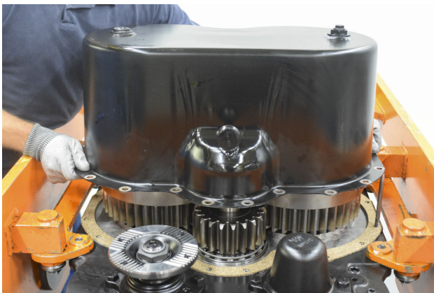
FIGURE 158: Install cover, use 2x guide pins.
