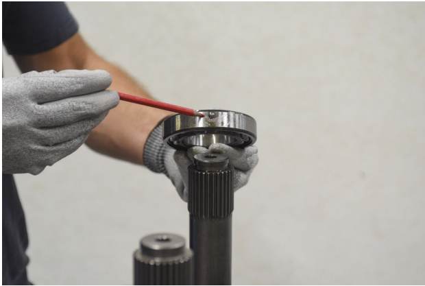
FIGURE 115: Install bearing + lock ball, align bearing lock ball with notch in bearing bore.
