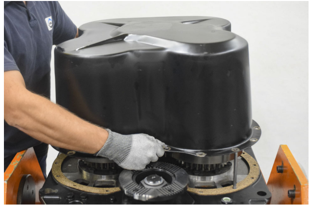
FIGURE 166: Install cover, use 2x guide pins.
