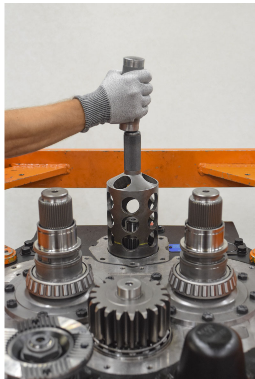
FIGURE 124: Install bearing cup using speial tool AS0010009800 (see drawing AS0010009800 p. 142).
