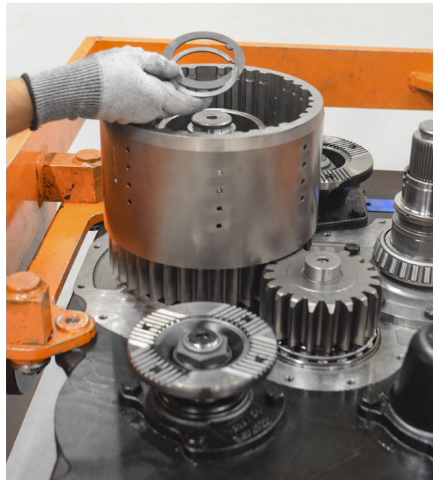
FIGURE 150: Install washer and snap-ring, when using new bearings follow shimming procedure below.
