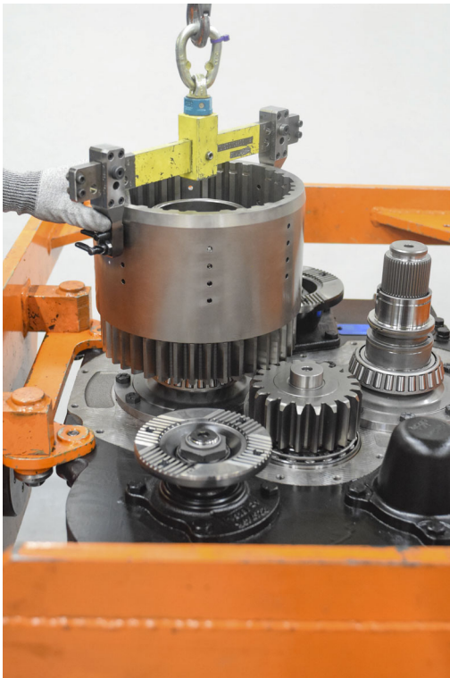
FIGURE 148: Grease and size clutch support piston rings and install clutch assembly using special tool TG1500106500 (see drawing TG1500106500 p. 144).
