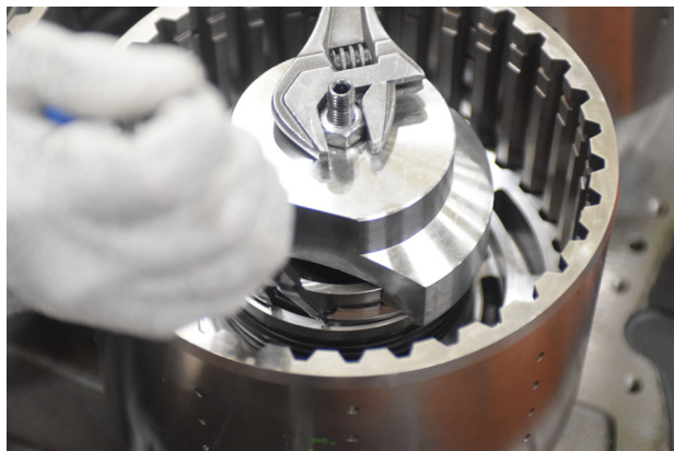
FIGURE 20: Using special tool AS0010012800 (see drawing AS0010012800 p. 153), push belleville washers down and remove snapping.
