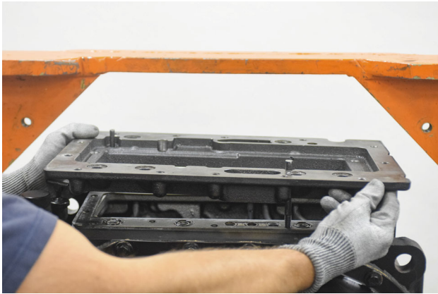
FIGURE 169: Install adaptor plate, use 2x guide pins.
