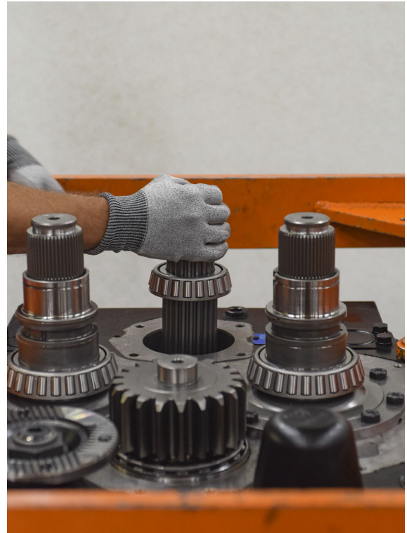
FIGURE 123: Lower shaft into bore hole through output gears.
