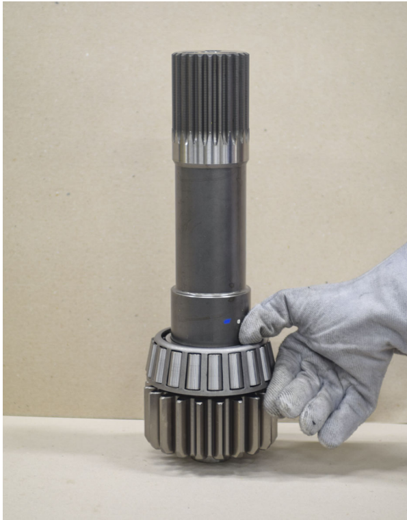
FIGURE 80: Install bearing (heat to 120°C).
