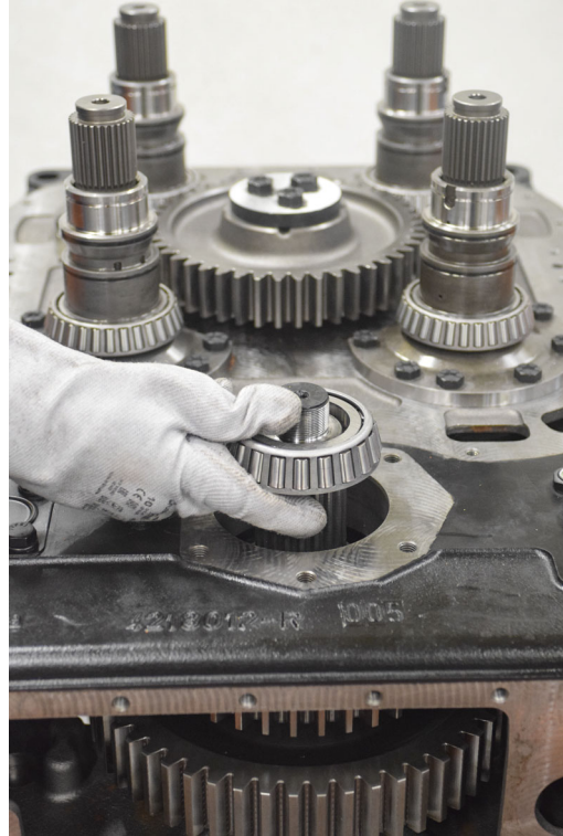
FIGURE 130: Install bearing cone (heat to 120°C).
