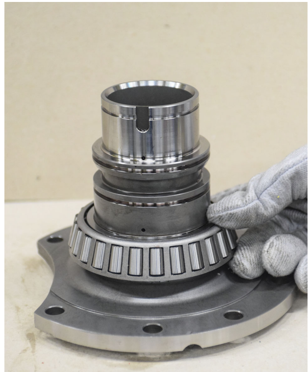
FIGURE 95: Install bearing (heat to 120°C).
