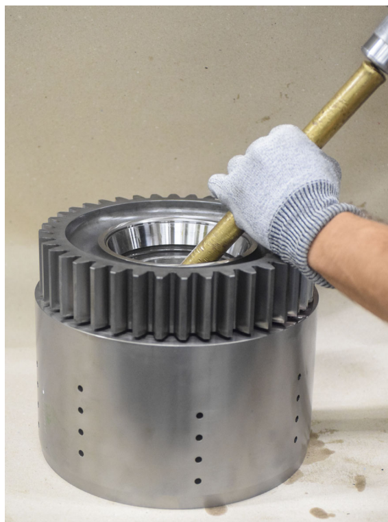
FIGURE 140: Remove bearing cup.
