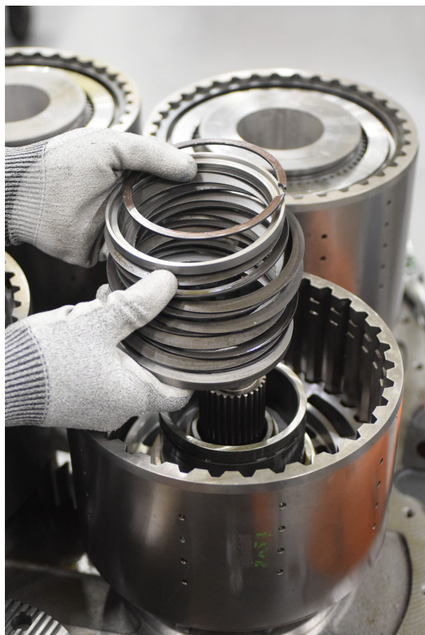
FIGURE 21: Remove snapping, spacer, Belleville washers and spacer.
