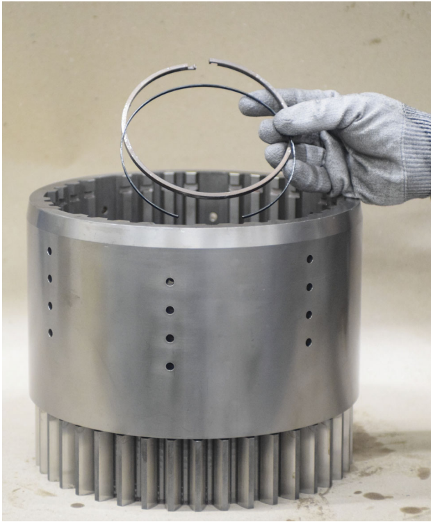
FIGURE 143: Install inner piston ring and expander.
