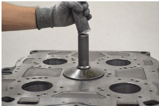
FIGURE 77: Install bearing cup.
