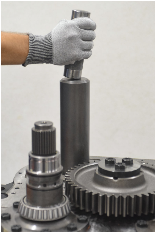
FIGURE 116: Tap bearing in position using special tool AS0010004200 (see drawing AS0010004200-000-001 p. 154).
