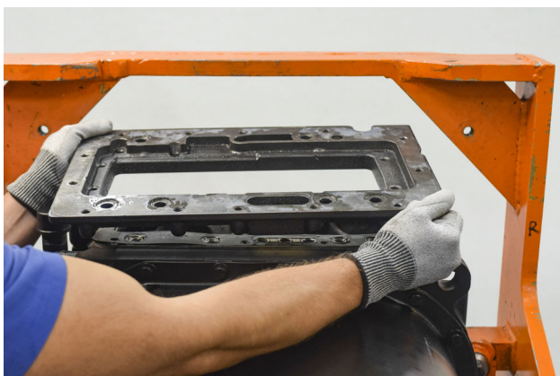
FIGURE 7: Remove adaptor plate.
