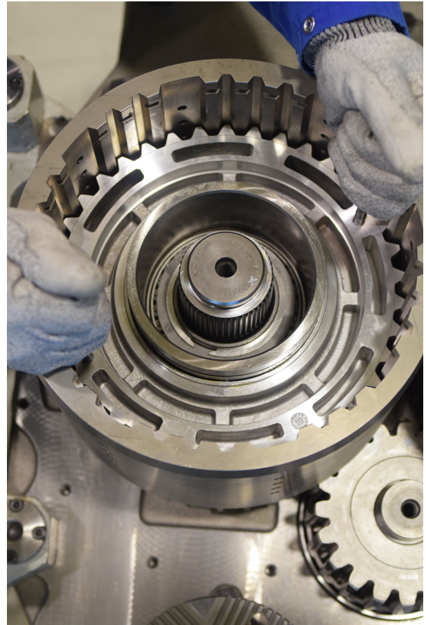
FIGURE 145: Install piston, use two guide pins.
