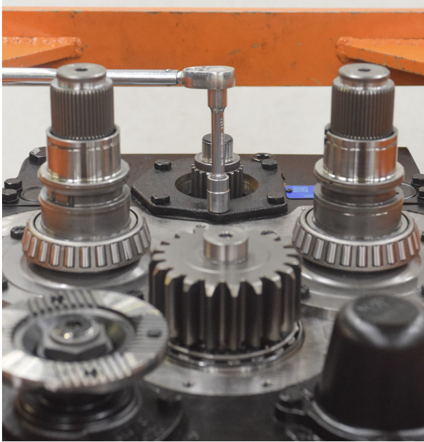
FIGURE 129: Install bearing cap +6x cap screws torque to 57-63 ft-lbs using special tools AS0010006400 (see drawing AS0010006400-000-001 p. 157) and AS0010005900 (see drawing AS0010005900-000-001 p. 155).
