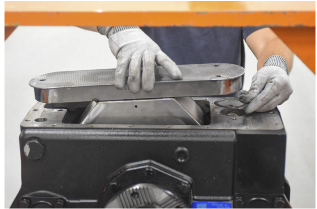
FIGURE 160: Install baffle + gasket.
