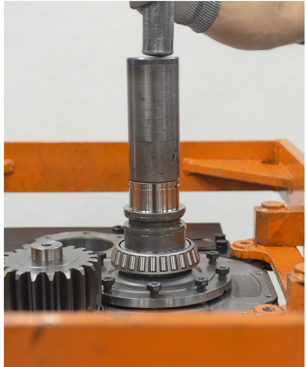
FIGURE 97: Install clutch support, align with 8x cap screws and tap clutch support down before driving the cap screws.
