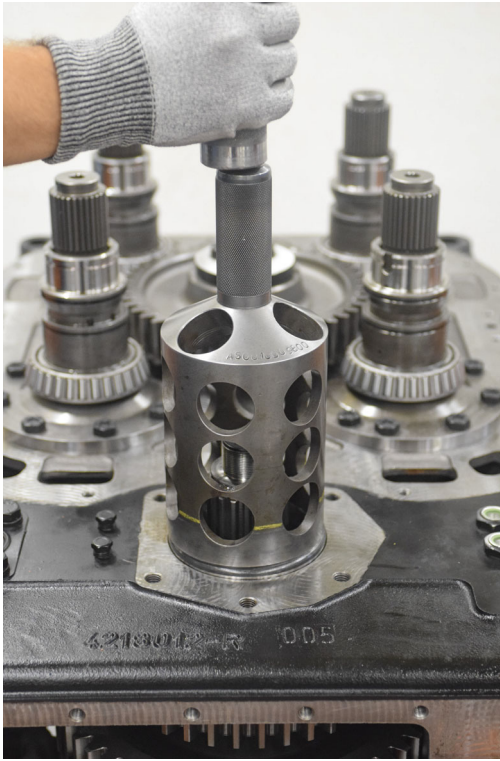
FIGURE 131: Install bearing cup using special tool AS0010009800 (see drawing AS0010009800 p. 142).
