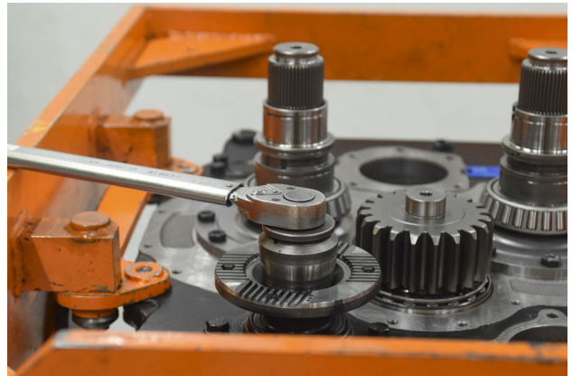
FIGURE 113: Block input shaft and torque nylon nut to 150-175 ft-lbs
