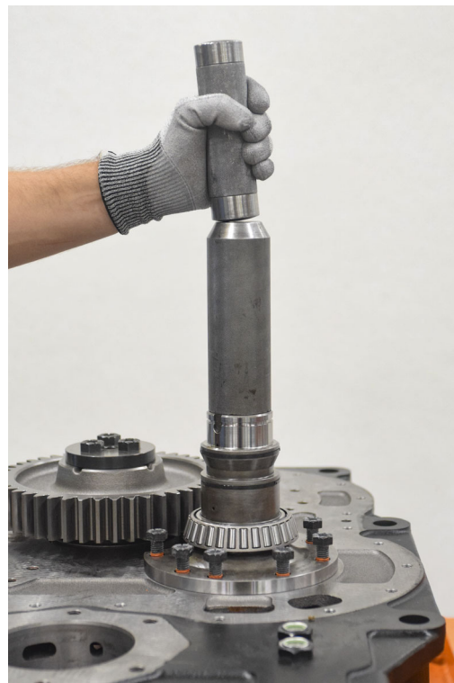
FIGURE 102: Install clutch support assembly, align with 8x cap screws and tap clutch support down before driving the cap screws.
