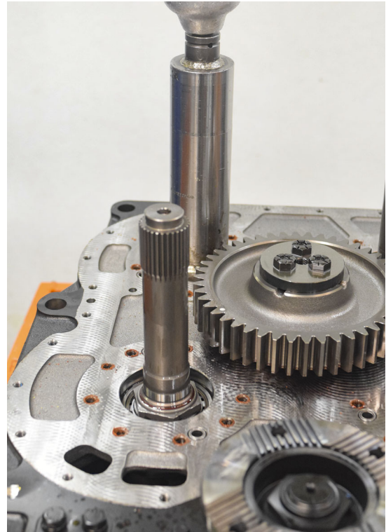
FIGURE 26: Remove 4x nylon nut using special tool AS0010005000 (see drawing AS0010005000 p. 140).
