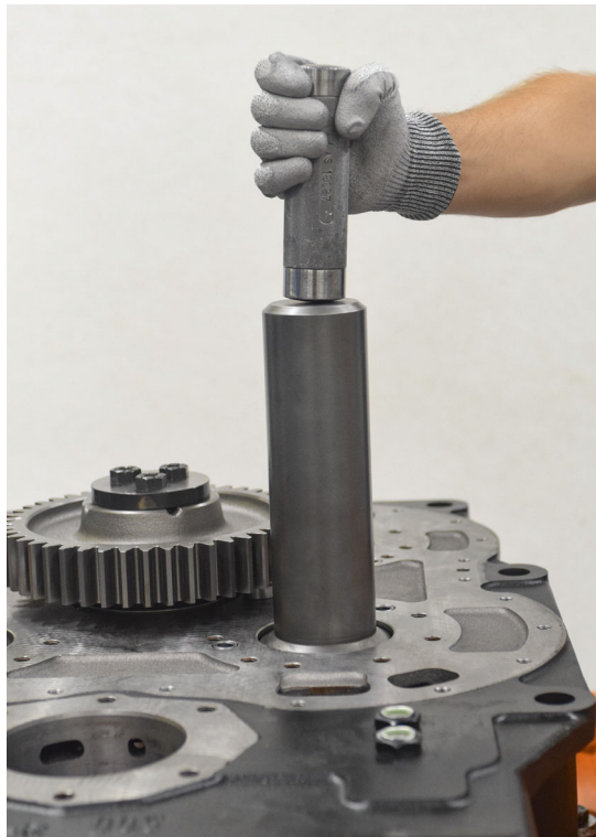
FIGURE 100: Tap bearing in position using special tool AS0010004200 (see drawing AS0010004200-000-001 p. 154).
