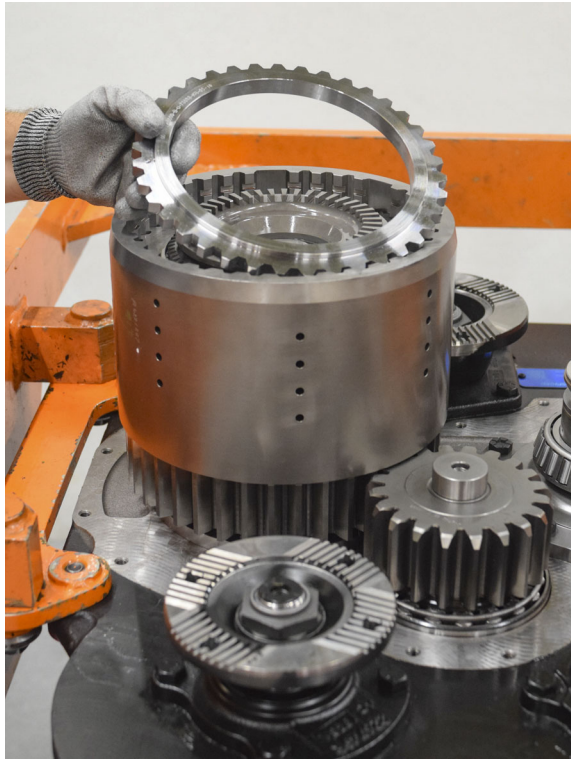
FIGURE 155: Install endplate.
