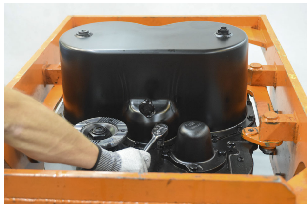
FIGURE 33: Remove 20x cap-screws + washers (size 9/16).
