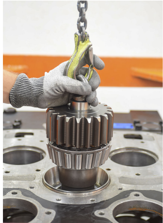
FIGURE 81: Lower idler shaft into transmission case (eyebolt M12).
