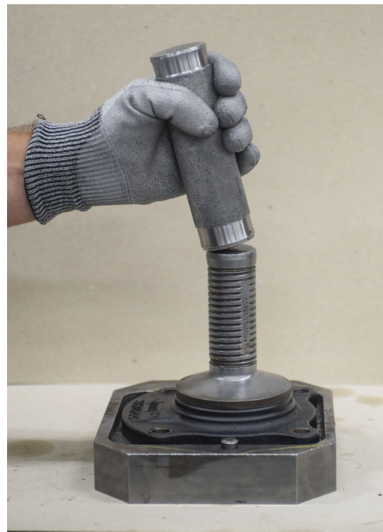
FIGURE 108: Install new seal, apply Loctite 641 using special tools AS0010006200 (see drawing AS0010006200-000-001 p. 156) and AS0010005900 (see drawing AS0010005900-000-001 p. 155).
