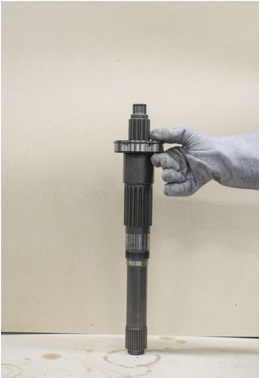
FIGURE 105: Install bearing (heat to 120°C).
