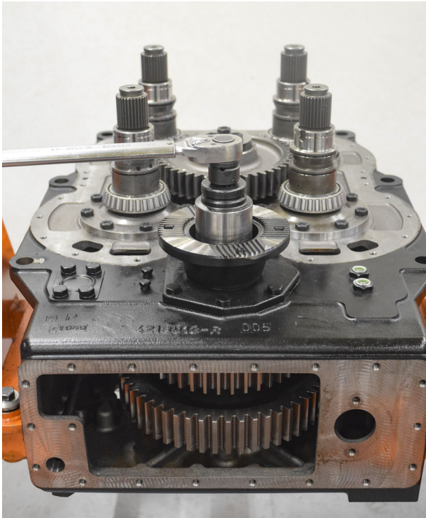
FIGURE 135: Torque nylon nut to 250-300 ft-lbs
