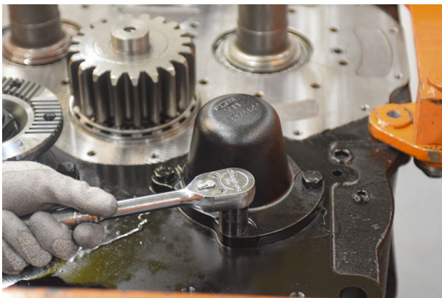
FIGURE 36: Remove 4x cap-screws (size 3/4).
