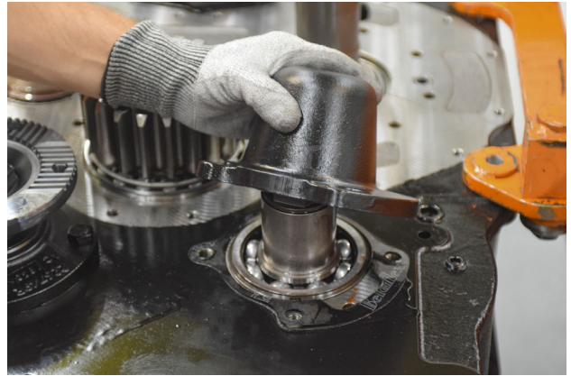
FIGURE 37: Remove Reverse cap.
