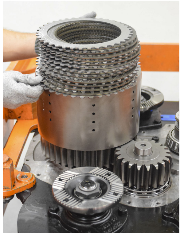
FIGURE 154: Installing clutch discs: Complete discs packs are supplied with an adjusted total thickness (pre-shimmed). Keep discs as ordered in the pack (from bottom to top). Start installing the bottom steel disc next to the piston, alternate friction and steel discs. In case clutch discs are mixed up, follow the assembly instructions at Clutch packs assembly instructions p. 64 to check the pack thickness, the pack shimming and position of the shims into the clutch pack.
