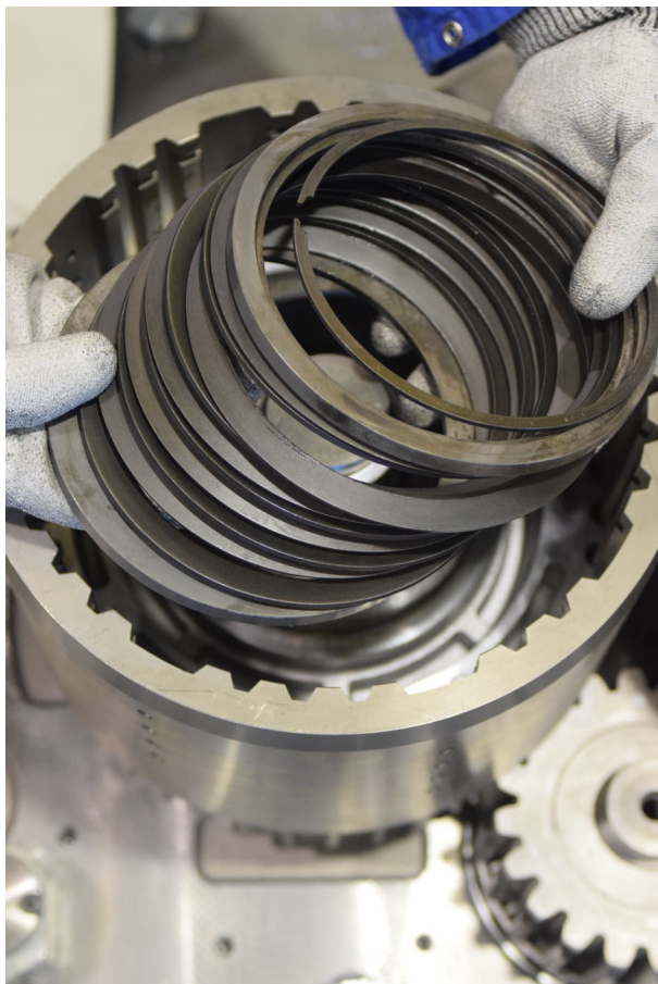
FIGURE 146: Install spacer, Belleville washers, spacer and snapping.
