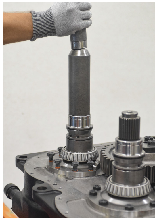
FIGURE 118: Install clutch support assembly, align with 8x cap screws and tap clutch support down before driving the cap screws.
