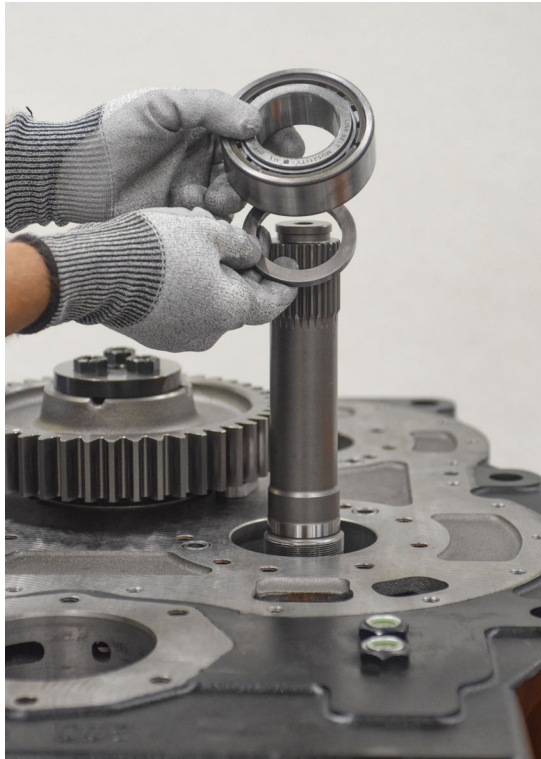
FIGURE 99: On the rear side install spacer and bearing (sharp inner radius of bearing is assembled to the top).
