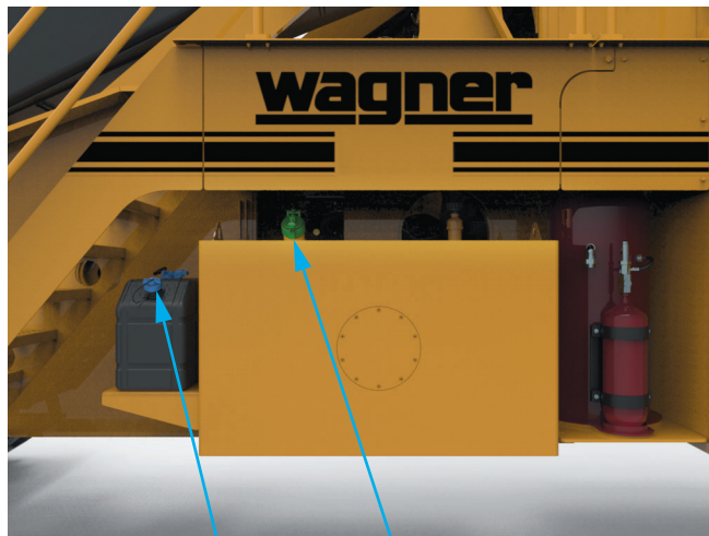
DEF Fill Diesel Fuel Fill Figure 5 Diesel Fuel Fill Cap
