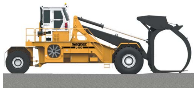
Figure 7 Normal Park Position (Carriage Tines Resting on the Ground, Kickoff Arms Retracted, Holddown Arms Touching the Ground)
