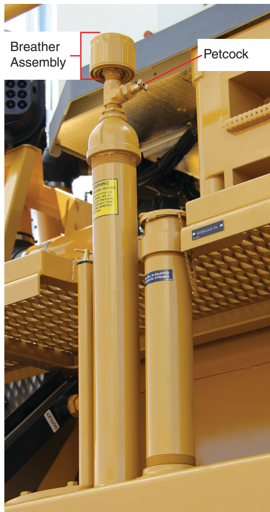
Figure 1 Typical Hydraulic Tank Breather Installation
