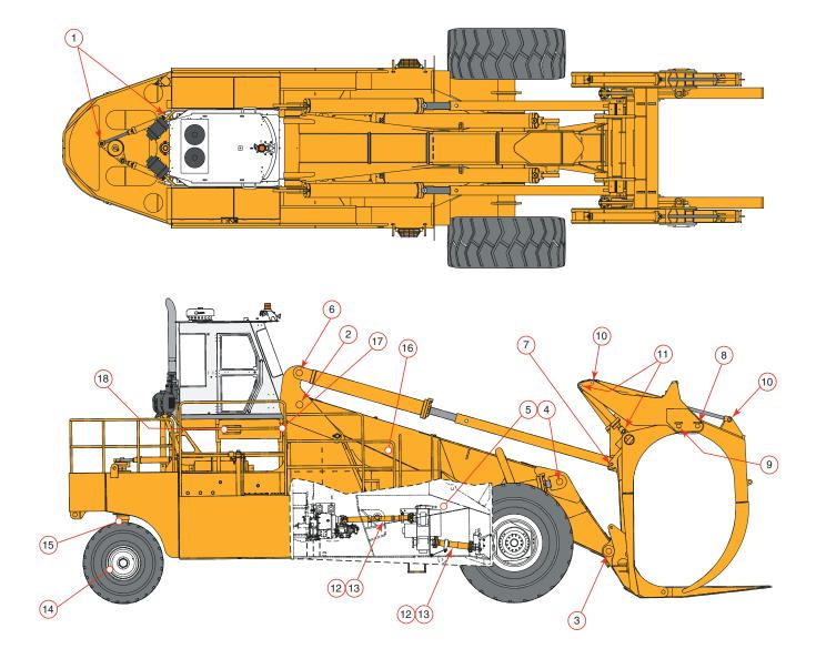
Figure 5-3-1 Lubrication Points
