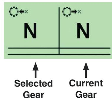
If the main screen does not display Selected Gear parameter on left side or Current Gear parameter on right side, press the button under the
