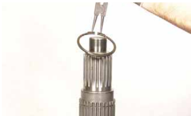
FIGURE 339: Install snap ring on output shaft.
