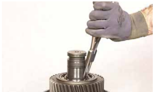
FIGURE 153: Remove snap ring.
