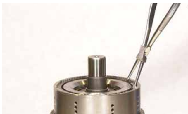
FIGURE 115: Remove 2nd clutch end plate snap ring.
