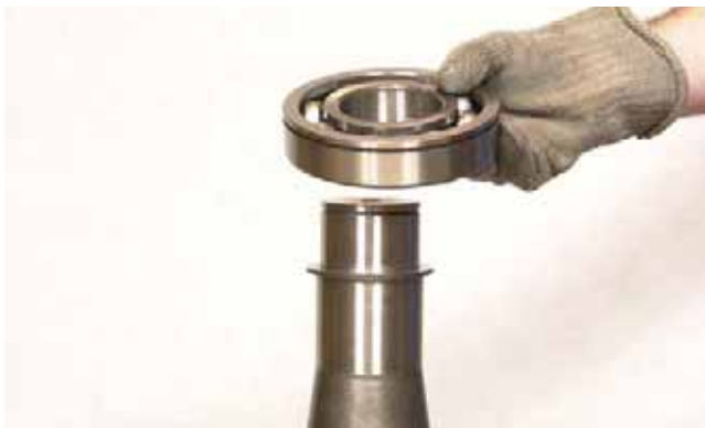
FIGURE 277: Warm bearing to 248°F [120°C] and install on shaft.
