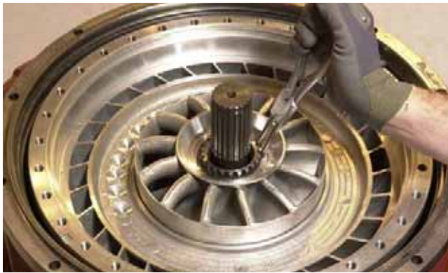
FIGURE 12: Remove reaction member snap ring.
