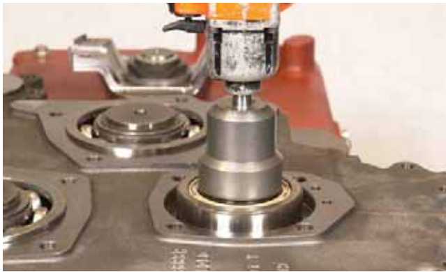
FIGURE 54: Use special tool to remove nut from 1st shaft. (See “Shaft Nut Socket”, on page 180.)
