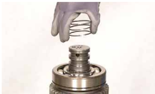
FIGURE 101: Remove piston rings (3).
