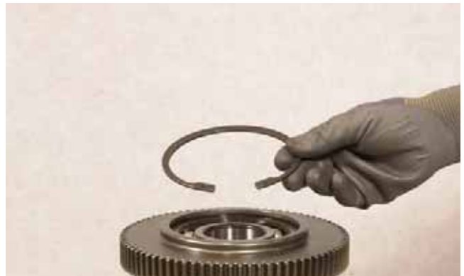
FIGURE 319: Install bearing snap ring.
