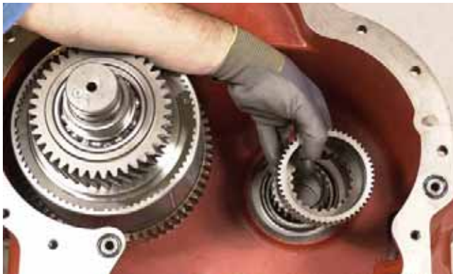
FIGURE 42: Remove 2nd clutch hub.
