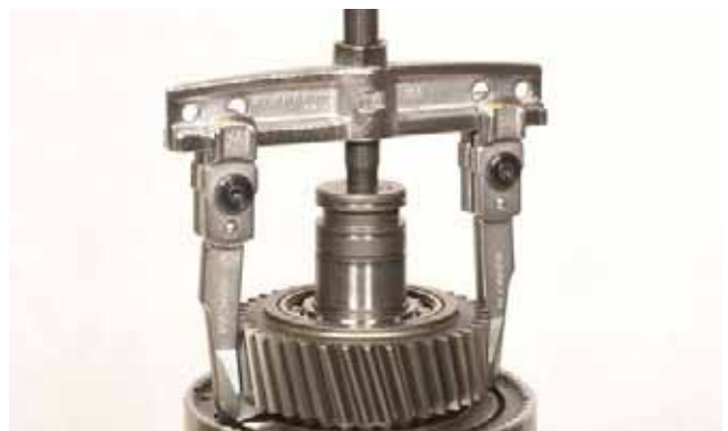
FIGURE 154: Using a puller, remove clutch gear and outer bearing.
