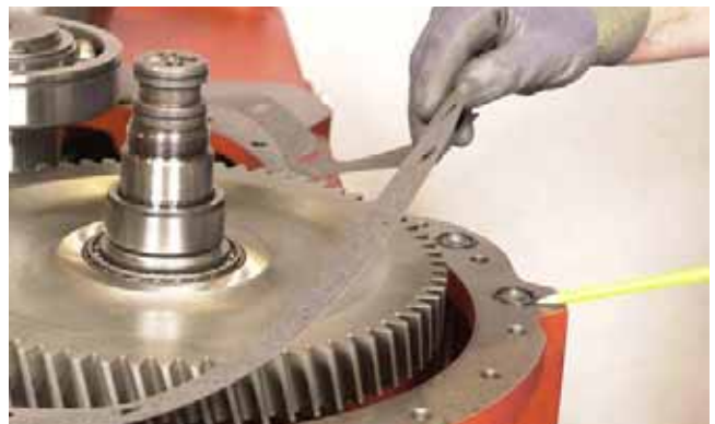
FIGURE 374: Install transmission-case-to-rear-cover new gasket and o-rings.
