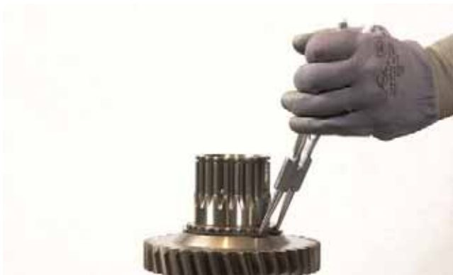
FIGURE 247: Remove snap ring.
