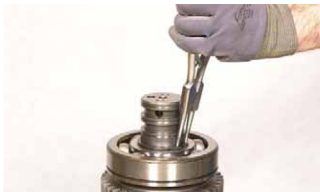
FIGURE 102: Remove bearing snap ring.
