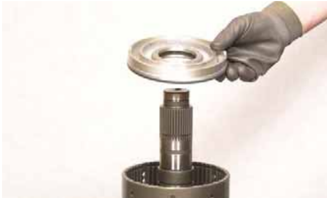
FIGURE 191: Remove clutch piston.
