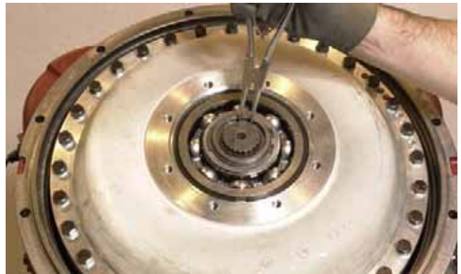
FIGURE 8: Remove turbine shaft outer snap ring.
