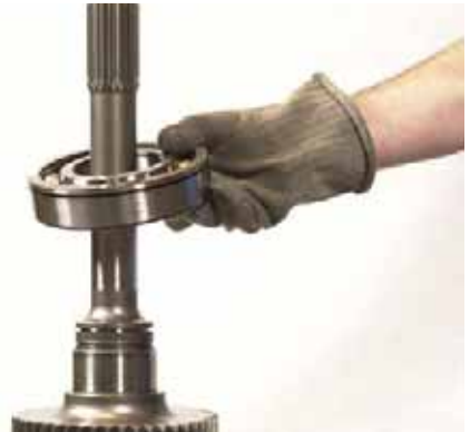
FIGURE 284: Warm bearing to 248°F [120°C] and install on shaft, ensuring that snap ring groove is up as shown.
