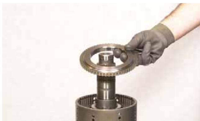
FIGURE 186: Remove end plate.
