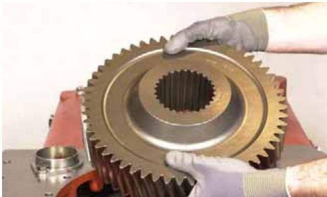
FIGURE 84: Remove output gear.
