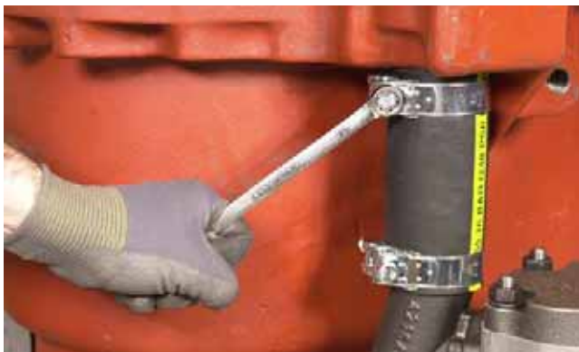
FIGURE 402: Tighten clamps on suction hose.
