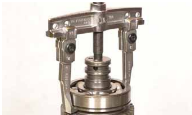
FIGURE 106: Remove clutch gear and outer bearing as an assembly.
