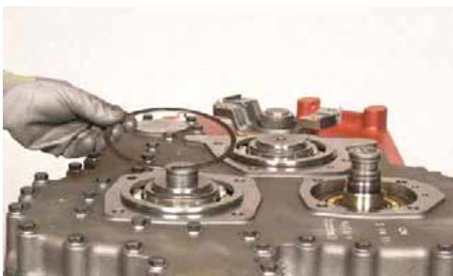
FIGURE 378: Raise 3rd shaft slightly and install snap ring.
