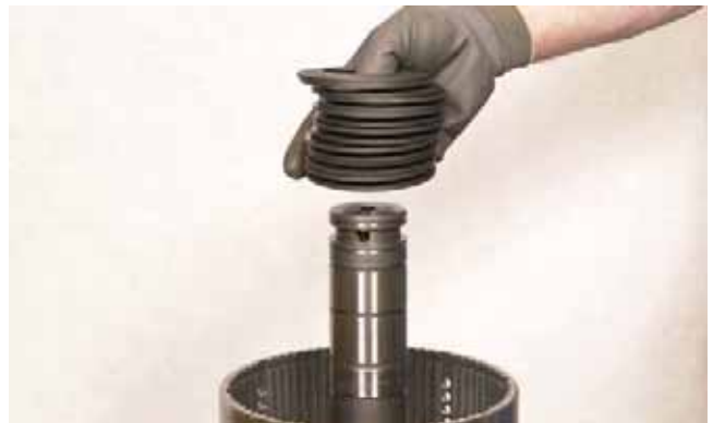
FIGURE 166: Install clutch piston Belleville washers. Position first washer with large diameter of bevel toward spacer (wear sleeve). Alternate fifteen (15) washers. Refer to Figure 167.
