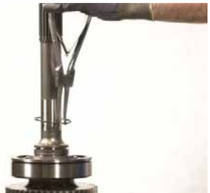
FIGURE 285: Install front bearing spacer.
