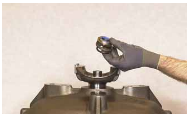
FIGURE 419: Install input flange o-ring, washer, and nut.
