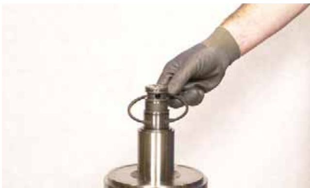
FIGURE 211: Remove snap ring.
