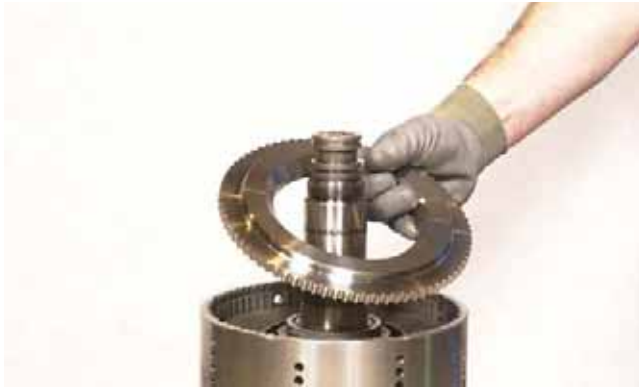
FIGURE 257: Install end plate.
