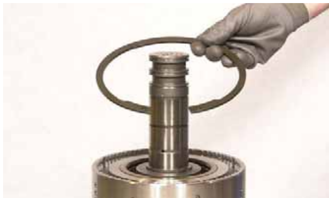
FIGURE 139: Install end plate in drum and fit end plate snap ring.
