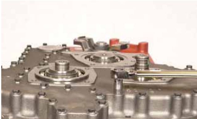
FIGURE 376: Install rear-cover-to-transmission-case bolts and tighten to specified torque. Refer to “TORQUE SPECIFICATIONS” on page 175.
