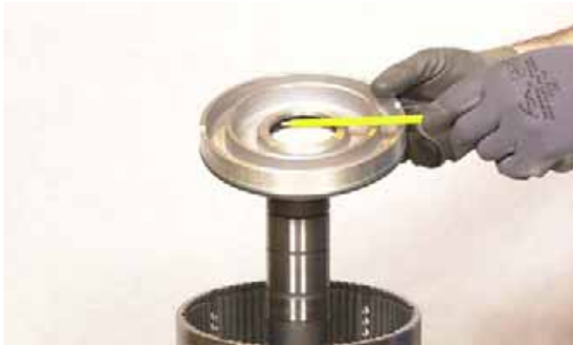
FIGURE 163: Install clutch piston inner seal.
