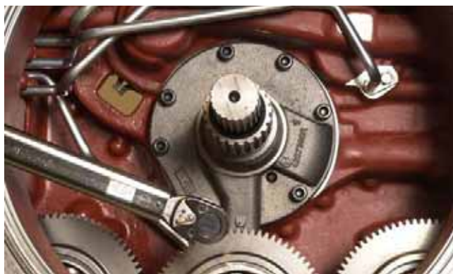
FIGURE 326: Install stator support assembly bolts and lockwashers and tighten to specified torque. Refer to "TORQUE SPECIFICATIONS" on page 175.
