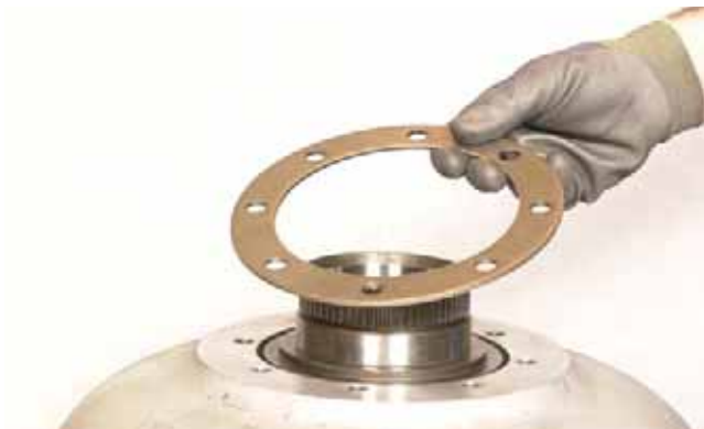
FIGURE 300: Position impeller hub backing ring.
