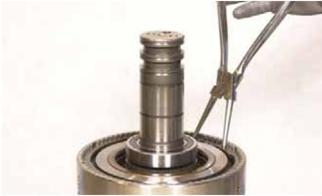
FIGURE 107: Remove end plate snap ring.
