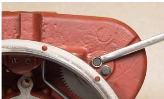
FIGURE 31: Remove pump drive gear bolts.
