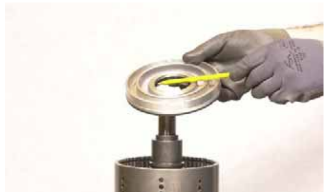
FIGURE 219: Install clutch piston inner seal.
