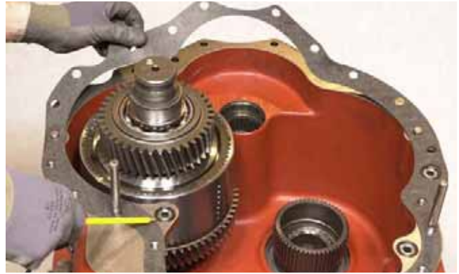
FIGURE 391: Install new converter-housing-to-transmission-case gasket and new o-rings (3).
