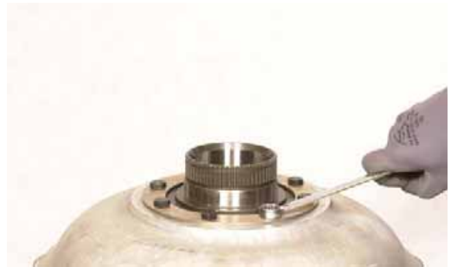
FIGURE 290: Remove impeller hub bolts.
