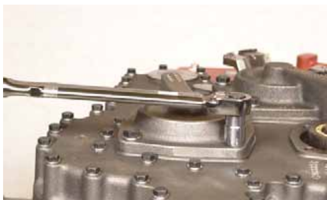
FIGURE 385: Install nuts and lockwashers to bearing cap and tighten to specified torque. Refer to "TORQUE SPECIFICATIONS" on page 175.
