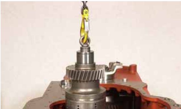
FIGURE 61: Remove 3rd shaft drum assembly.
