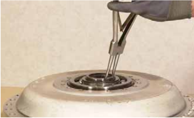
FIGURE 304: Remove turbine hub front bearing snap ring.
