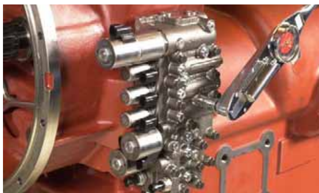
FIGURE 394: Install control valve and tighten capscrews to specified torque (refer to "TORQUE SPECIFICATIONS" on page 175), following the sequence outlined in the "Transmission Assembly Instructions" on page 97 of the manual.
