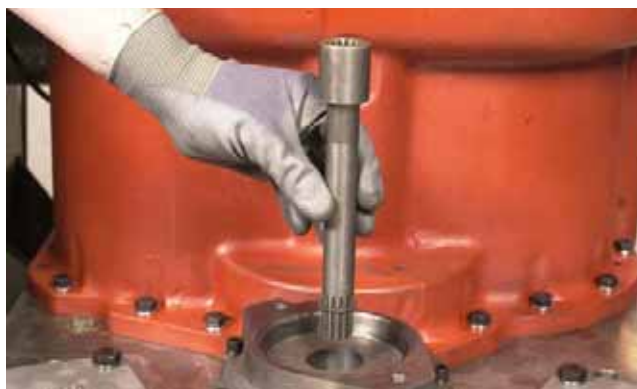
FIGURE 20: Remove gear-to-pump shaft.
