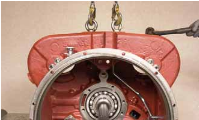
FIGURE 37: Support converter housing with chain hoist and strap. Use a soft hammer to separate converter housing from transmission case.
