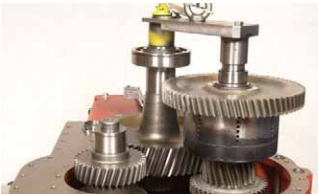
FIGURE 60: Shown are the 1st shaft drum assembly and idler shaft as an assembly, removed. (See “Idler & Low Shaft Lifting Hook”, on page 178.)
