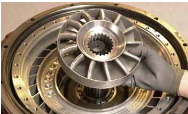
FIGURE 13: Remove reaction member.
