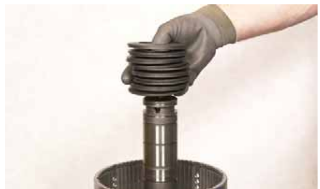
FIGURE 160: Remove Belleville washers.
