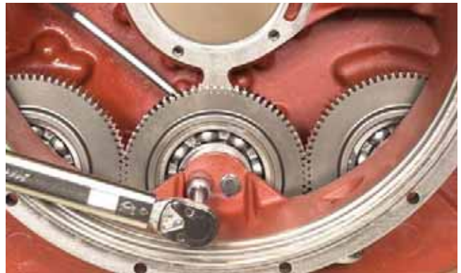
FIGURE 321: Install center charging pump drive gear assembly. Tighten bolts to specified torque. Refer to "TORQUE SPECIFICATIONS" on page 175.
