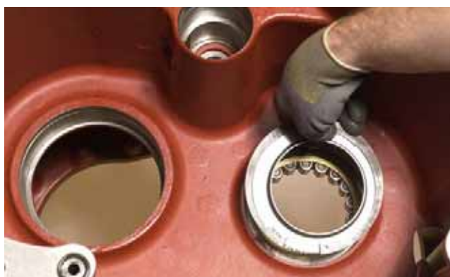
FIGURE 362: Install 1st clutch shaft oil retainer and snap ring. Refer to Figure 363.
