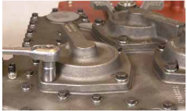
FIGURE 44: Remove bolts from 3rd clutch shaft rear bearing.
