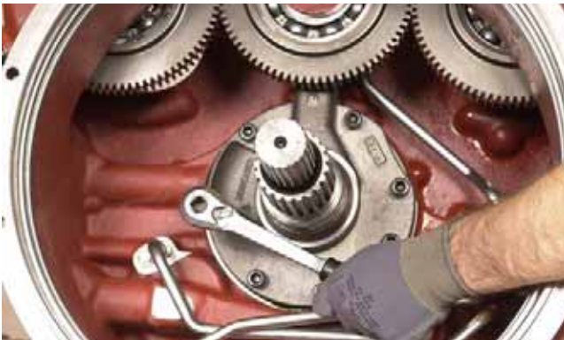
FIGURE 25: Remove stator support assembly bolts and lockwashers.
