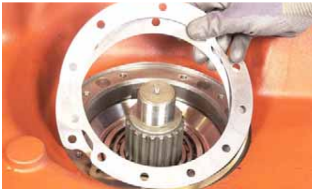
FIGURE 348: Position shims on transmission case.
