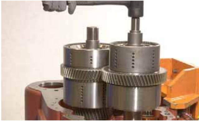
FIGURE 328: Install 4th shaft and drum assembly converter housing.
