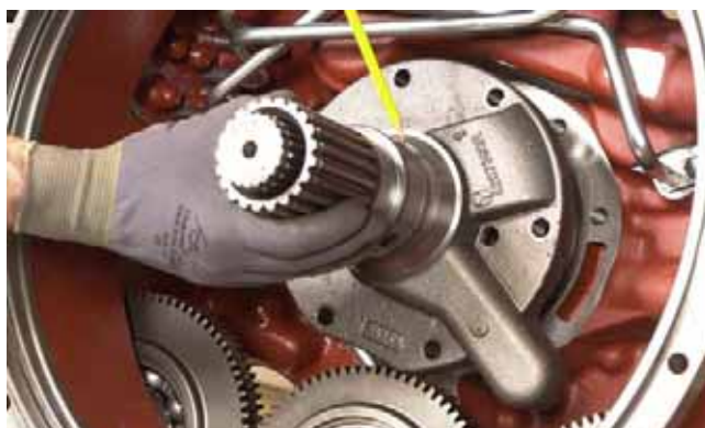
FIGURE 325: Install new o-ring and piston ring on stator support. Position stator support assembly on turbine shaft. Turn stator support assembly to clear pump drive gear. Align support assembly holes with converter housing.
