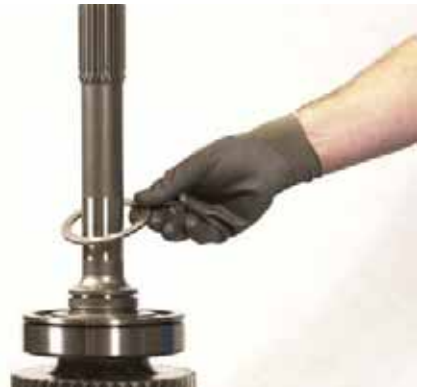
FIGURE 285: Install front bearing spacer.
