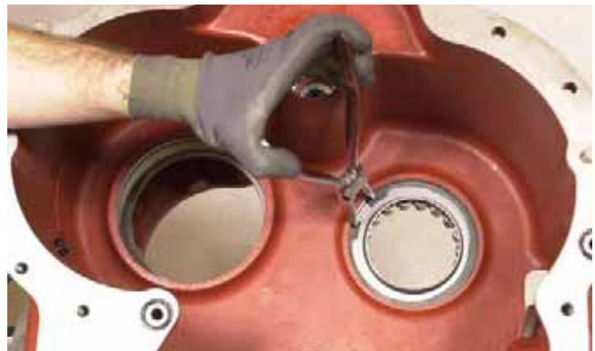
FIGURE 64: Remove 1st shaft drum assembly front bearing snap ring.
