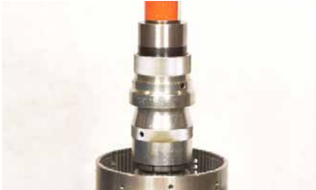
FIGURE 239: Using a bearing puller, remove lower hub taper roller bearing from shaft.
