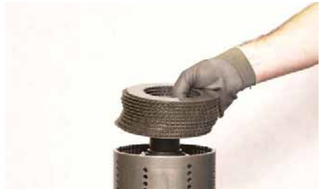
FIGURE 225: Install one (1) friction disc. Alternate steel and friction discs until proper number of discs are installed.
