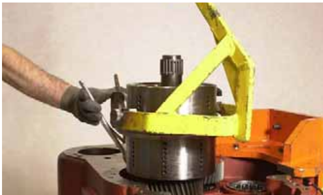
FIGURE 97: Using external snap ring pliers, open Rev/2nd drum shaft assembly bearing snap ring and remove shaft assembly
