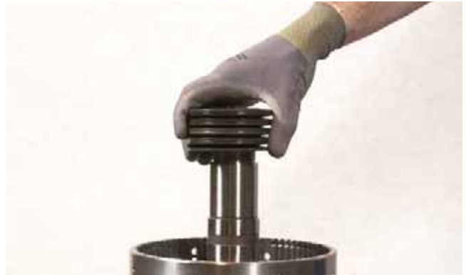
FIGURE 242: Remove Belleville washers.
