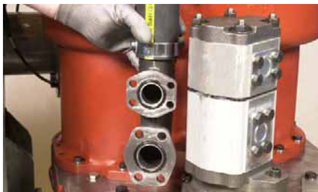
FIGURE 17: Remove suction adapter assembly and o-rings.
