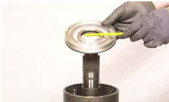
FIGURE 192: Install clutch piston inner seal.
