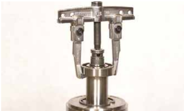
FIGURE 210: Using a puller as shown, remove front bearing shaft.
