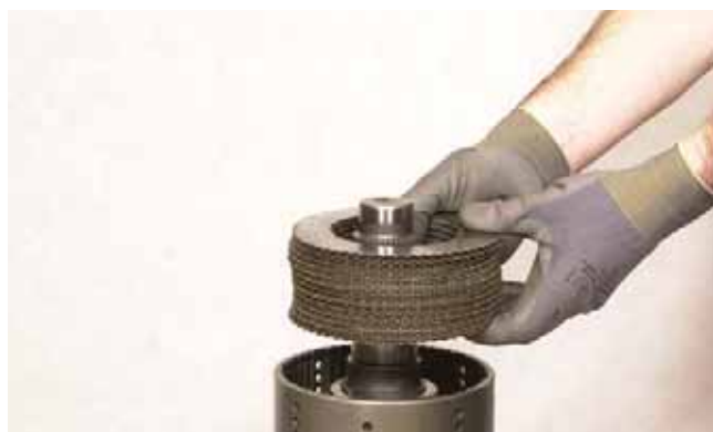
FIGURE 187: Remove clutch inner and outer discs.
