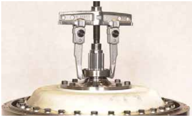
FIGURE 6: Remove input shaft support bearing.
