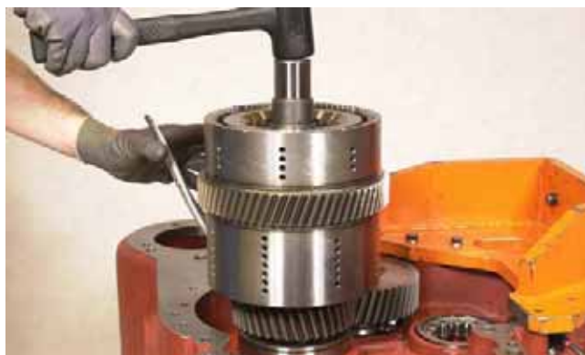
FIGURE 327: Spread ears on snap ring and install 2nd/Rev clutch drum assembly into converter housing.
