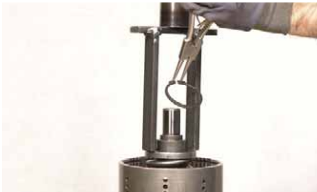
FIGURE 223: Compress spring and install snap ring.
