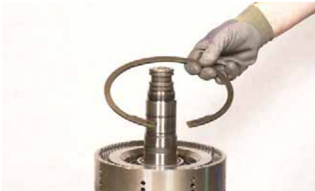
FIGURE 258: Install end plate snap ring.
