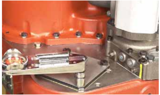
FIGURE 403: Install hydraulic pump drive shipping covers (if fitted) and install bolts and lockwashers. Tighten to specified torque. Refer to "TORQUE SPECIFICATIONS" on page 175.
