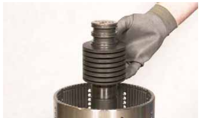
FIGURE 112: Remove Belleville washers.
