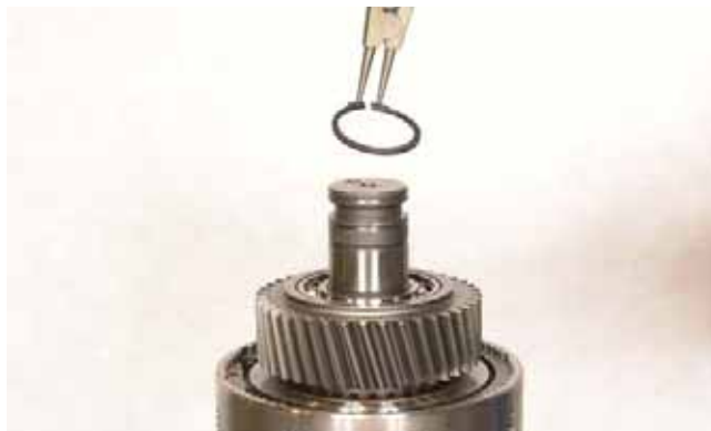
FIGURE 173: Install bearing snap ring.
