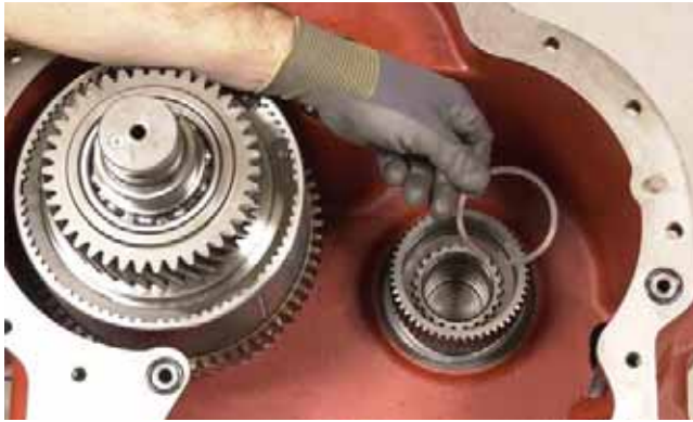
FIGURE 41: Remove inner snap ring from 2nd clutch hub.
