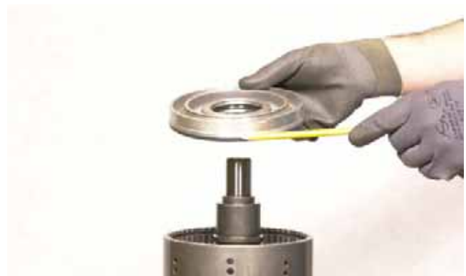
FIGURE 220: Install clutch piston outer seal and install piston into drum.
