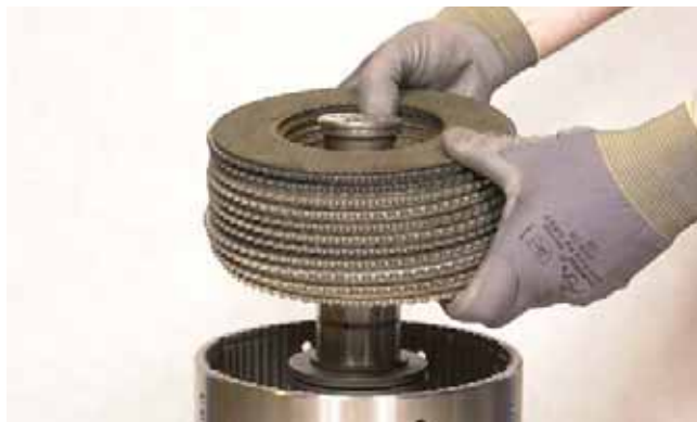
FIGURE 137: Install one (1) clutch inner/outer steel disc into drum. Alternate friction and steel discs until proper number of discs are installed. First and last discs are steel.
