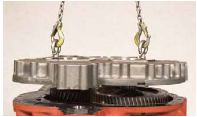
FIGURE 56: Using a hoist, remove rear cover from transmission case. Tap 3rd/1st shaft with a soft hammer to assist removal and avoid bending shaft.
