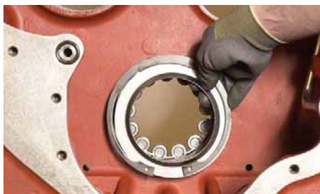
FIGURE 359: Install idler shaft, oil retainer, and snapring. Refer to Figure 360.
