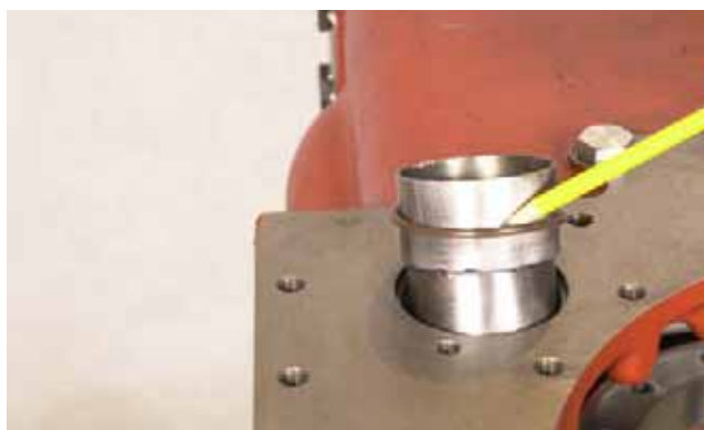
FIGURE 94: Remove suction tube assembly and o-ring.
