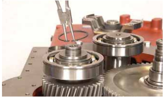
FIGURE 373: Install snap ring.
