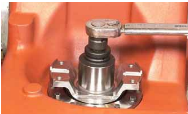
FIGURE 354: Tighten front output flange nut to 250 - 300 lbs. ft. (339 - 407 N•m).
