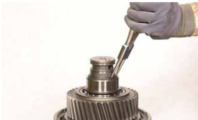
FIGURE 151: Remove bearing snap ring.
