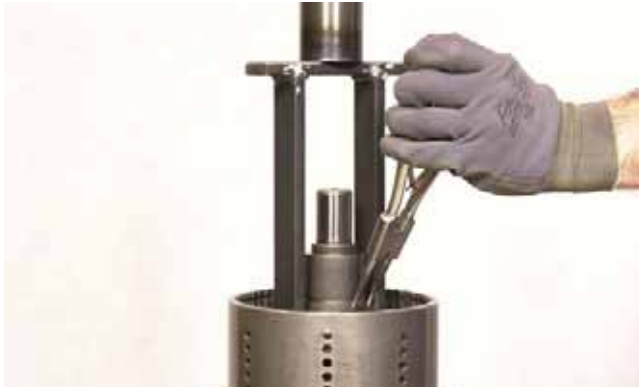
FIGURE 215: Compress spring and remove snap ring.
