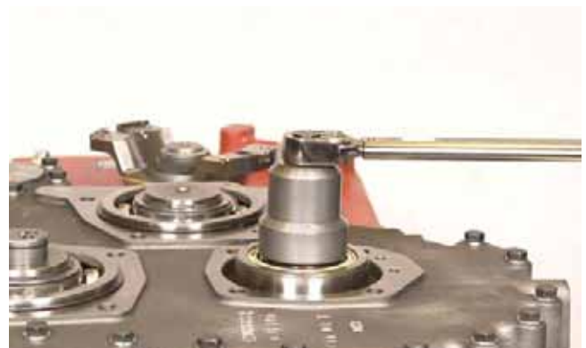
FIGURE 381: Using special tool “Shaft Nut Socket” (see page 180), torque lock nut to 107–118 lbs ft. [145–160 N•m].
