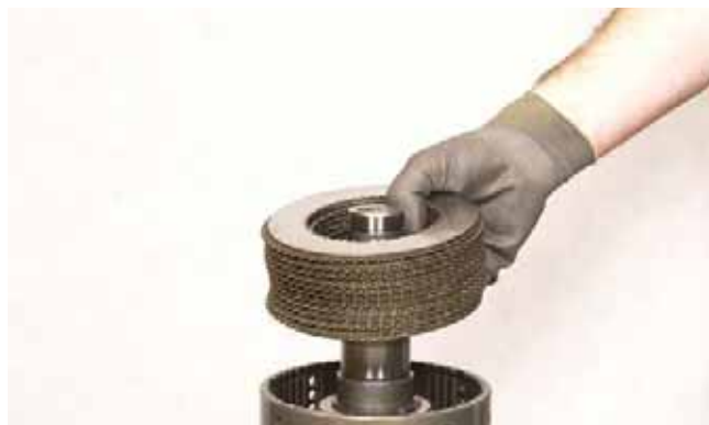
FIGURE 199: Install steel discs. Alternate friction and steel discs until proper number of discs are installed. First and last discs are steel.
