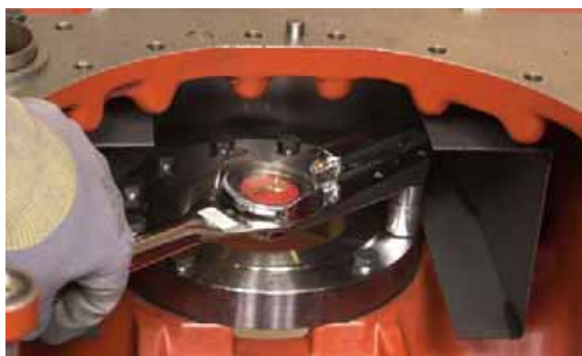
FIGURE 337: Install inside front cap bolts and tighten to specific torque. Refer to “TORQUE SPECIFICATIONS” on page 175.
