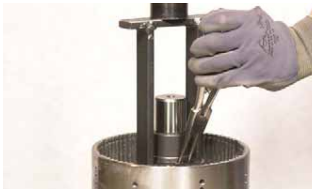
FIGURE 118: Compress return springs and remove snap ring.
