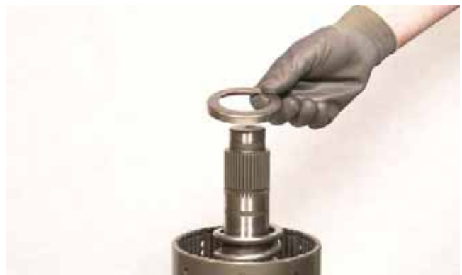
FIGURE 196: Install spring retainer.
