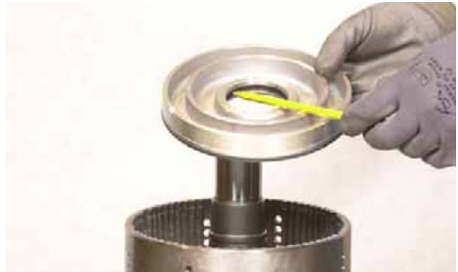
FIGURE 122: Install clutch piston inner seal. Rotate piston until seal is flush with outer diameter of piston.
