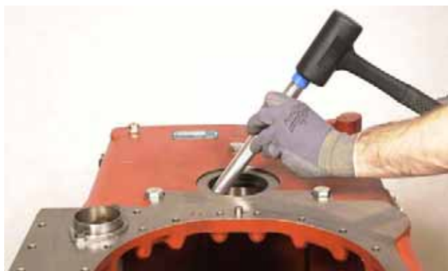
FIGURE 89: Tap rear bearing cup from case.
