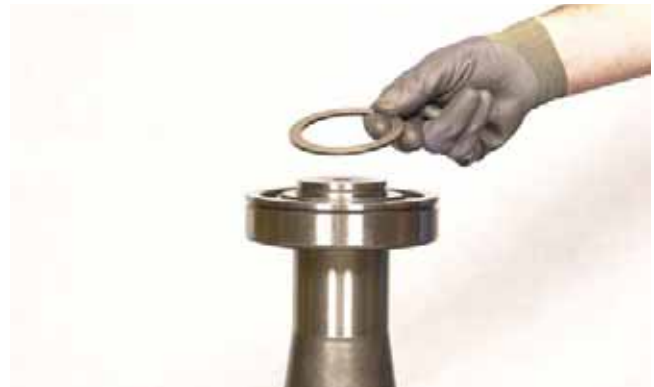
FIGURE 278: Install idler shaft rear bearing spacer.
