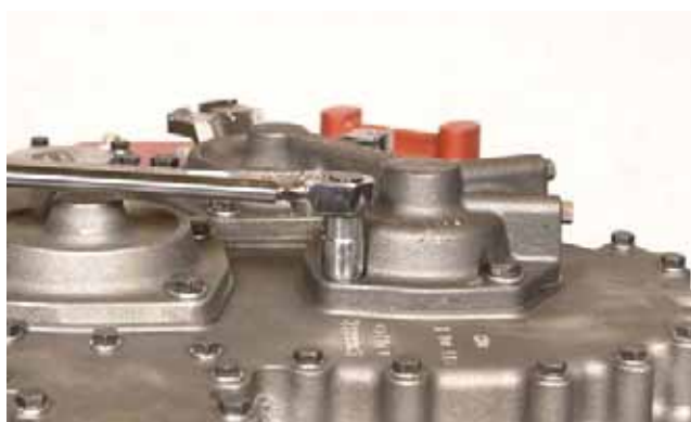
FIGURE 387: Install bolts and lockwashers to bearing cap and tighten to specified torque. Refer to "TORQUE SPECIFICATIONS" on page 175.
