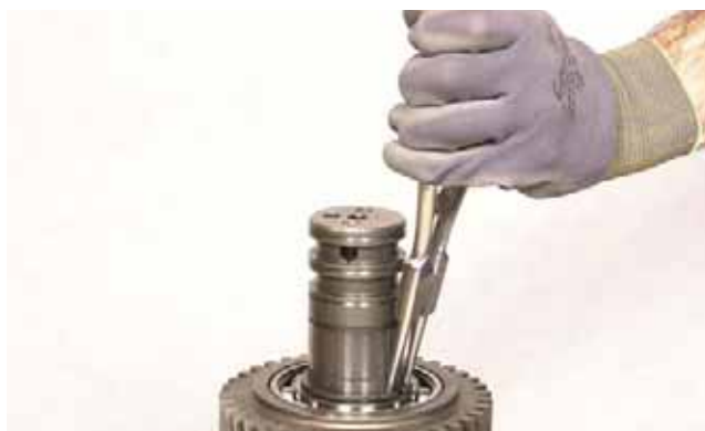
FIGURE 105: Remove clutch gear snap ring.
