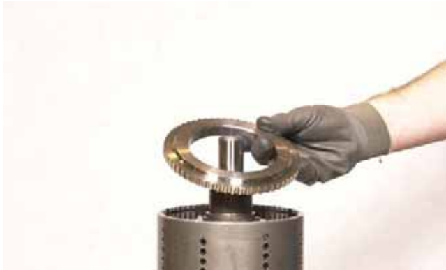
FIGURE 227: Install end plate.
