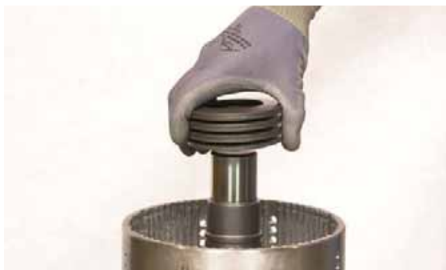
FIGURE 125: Install piston Belleville washers. Position first washer with large diameter of bevel toward spacer (wear sleeve). Refer to Figure 126. Alternate seven washers.
