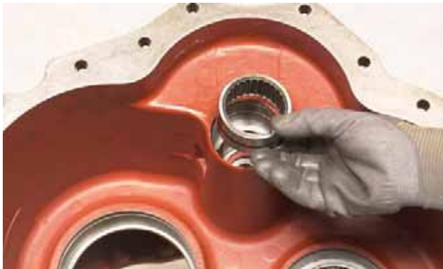
FIGURE 364: Install turbine shaft needle roller bearing.
