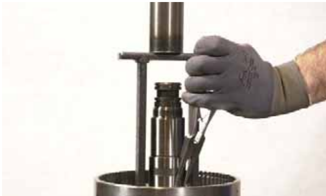
FIGURE 240: Compress Belleville washers and remove piston return spring snap ring.
