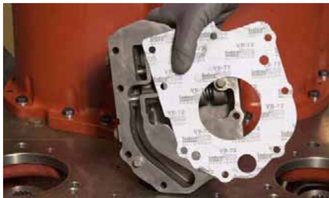
FIGURE 395: Install regulator valve and new valve-to-converter-housing gasket to converter housing.
