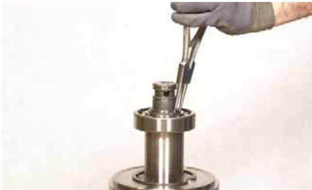
FIGURE 209: Remove bearing snap ring.
