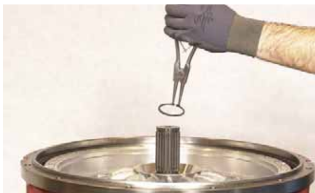
FIGURE 409: Install turbine hub rear snap ring on shaft.
