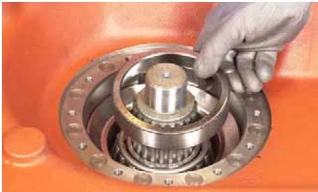
FIGURE 347: Install front bearing cup.
