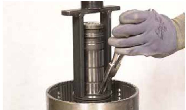
FIGURE 111: Compress piston return springs and remove spring snap ring.
