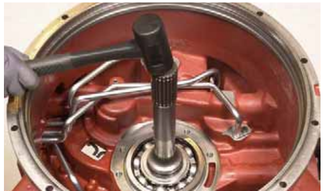
FIGURE 99: Using a soft hammer, tap turbine shaft and bearing assembly from converter housing.
