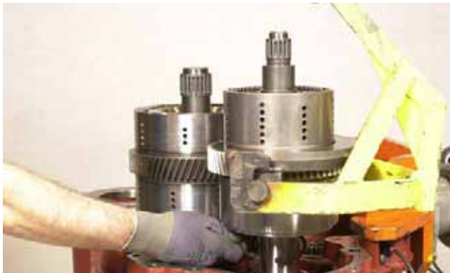
FIGURE 96: Remove 4th drum shaft assembly using special tool. (See “4th Drum Lifting Hook”, on page 181.)
