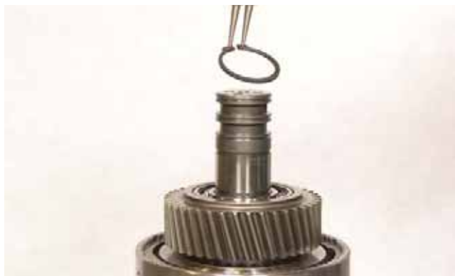
FIGURE 141: Install bearing snap ring.
