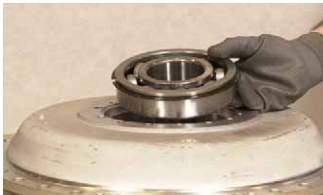
FIGURE 310: Center impeller cover over turbine hub. Install bearing in impeller cover and over turbine hub. Tap bearing into place.
