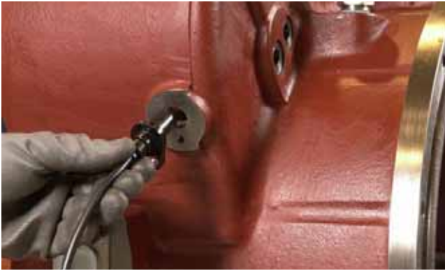
FIGURE 35: Remove all sensors from converter housing (3).
