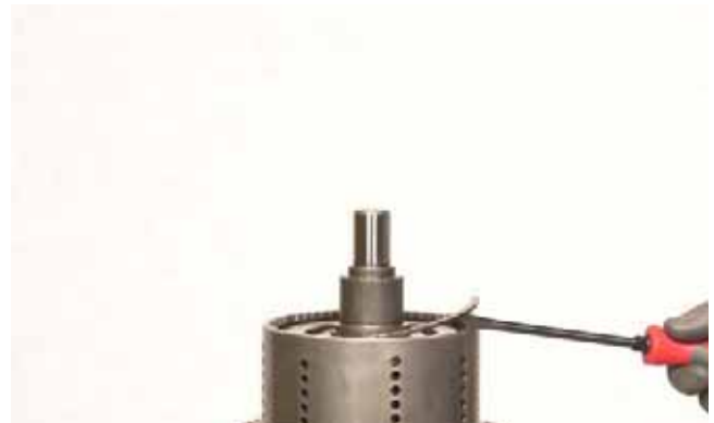
FIGURE 212: Remove end plate snap ring.
