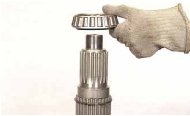
FIGURE 340: Warm rear bearing cone to 248°F [120°C] and install on output shaft.
