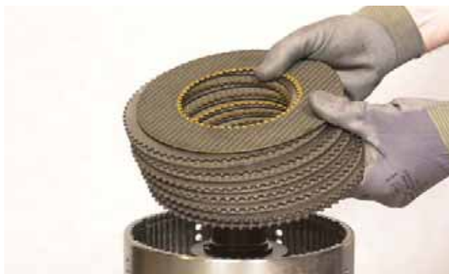
FIGURE 128: Install clutch inner and outer discs into drum. Start with one steel disc against piston. Alternate friction and steel discs until proper number of discs are installed. Last disc is friction disc.
