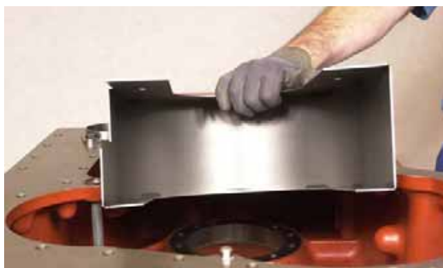
FIGURE 334: Install oil baffle with LOCTITE® 262™ on threads of capscrews. Torque to specified torque. Refer to “TORQUE SPECIFICATIONS” on page 175.
