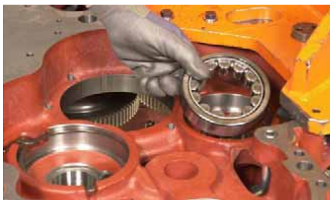
FIGURE 322: Install forward speed outer roller bearing in converter housing.
