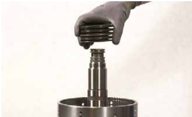
FIGURE 252: Install Belleville washers. Position first washer with large diameter of bevel toward spacer (wear sleeve). Alternate nine (9) washers. Refer to Figure 253.
