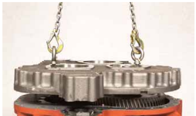
FIGURE 375: Install two aligning studs and install transmission rear cover.
