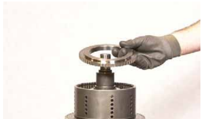
FIGURE 213: Remove end plate.
