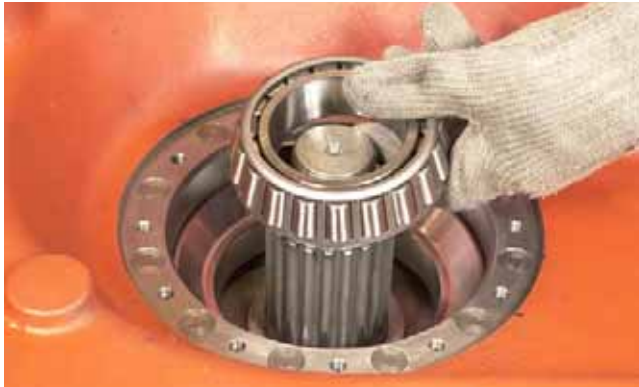
FIGURE 346: Install front bearing cone and warm to to 248°F [120°C].
