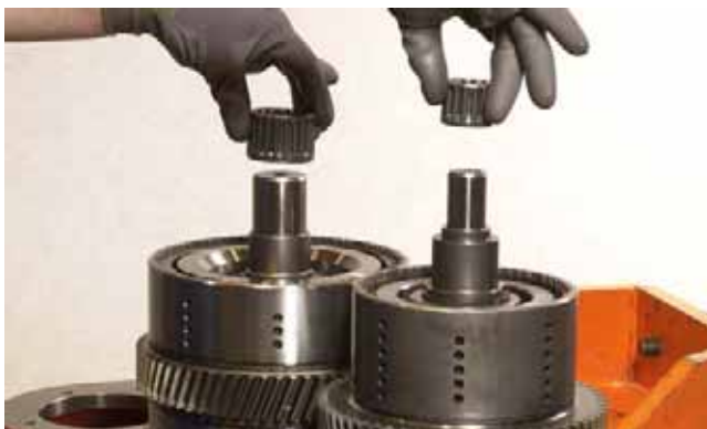
FIGURE 330: Install needle roller bearings on 2nd/Rev and 4th shafts.
