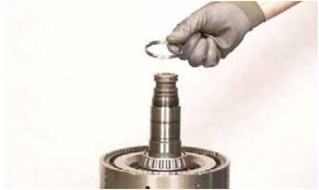
FIGURE 260: Install bearing spacer.
