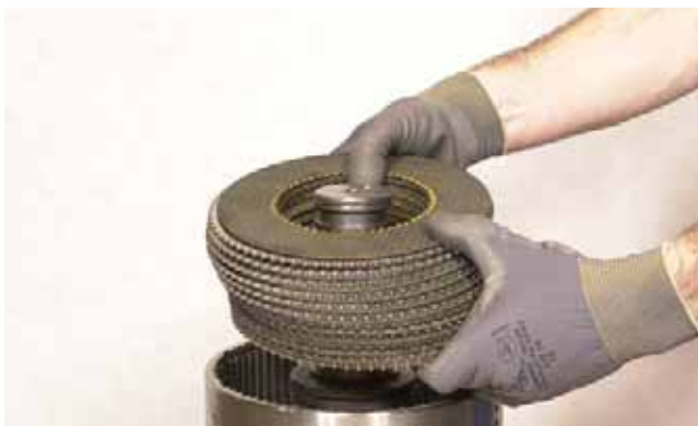
FIGURE 169: Install steel discs. Alternate friction and steel discs until proper number of discs are installed. First and last discs are steel.
