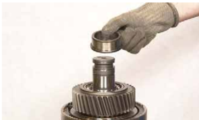
FIGURE 174: Install bearing inner race.
