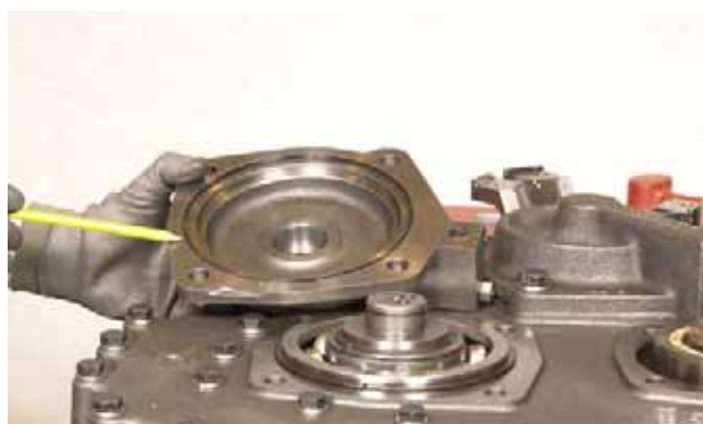
FIGURE 384: Fit o-ring (2) to 3rd shaft bearing cap and install bearing cap.
