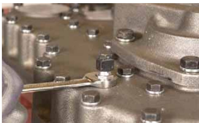
FIGURE 422: Install temperature sensor.
