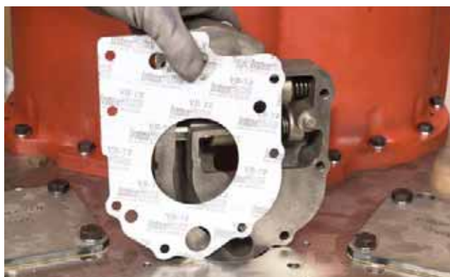
FIGURE 22: Remove regulator valve assembly and gasket.
