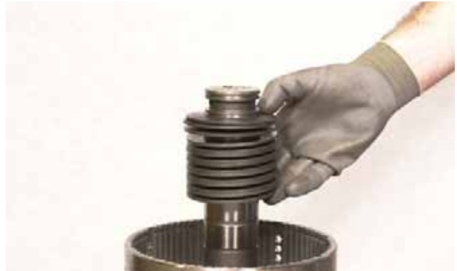
FIGURE 134: Install clutch piston Belleville washers. Position first washer with large diameter of bevel toward spacer (wear sleeve). Alternate fifteen (15) washers. Refer to Figure 135.
