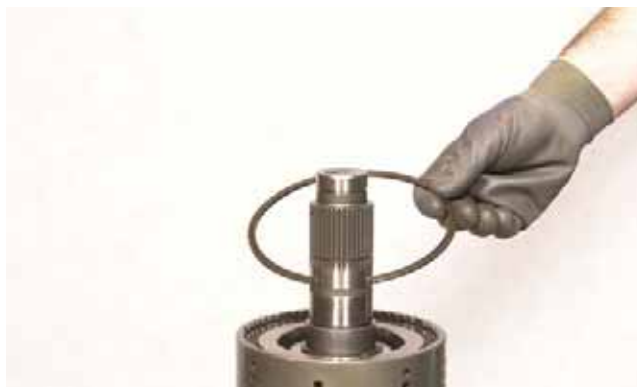
FIGURE 202: Install snap ring.
