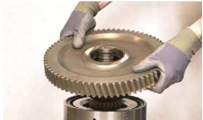
FIGURE 261: Install clutch driven gear and hub assembly. Align splines on clutch gear hub with internal splines of friction discs.
