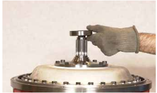
FIGURE 415: Warm input shaft support bearing to 248°F [120°C] and install on input shaft.
