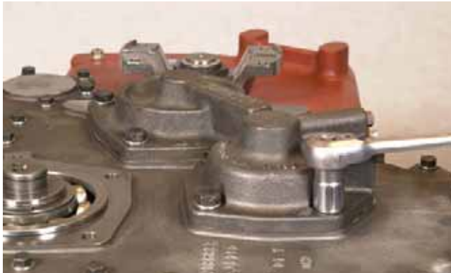
FIGURE 47: Remove 1st clutch shaft rear bearing cap bolts.
