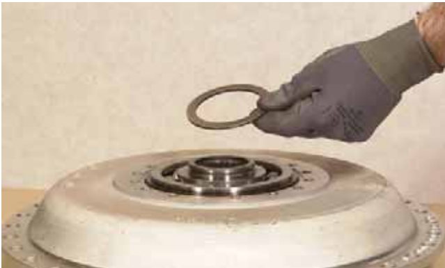
FIGURE 305: Remove turbine hub front bearing washer.
