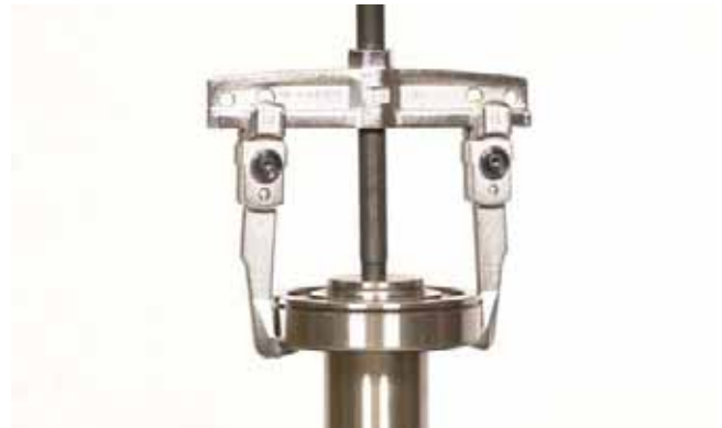
FIGURE 272: Using a puller, remove idler shaft rear bearing.
