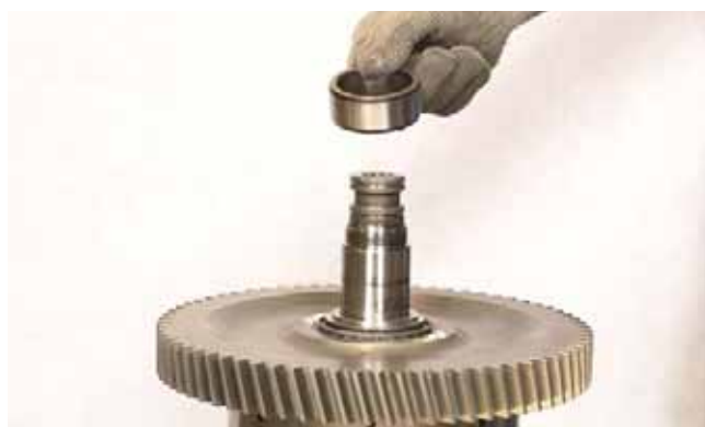
FIGURE 264: Warm bearing to 248°F [120°C] and install on shaft.
