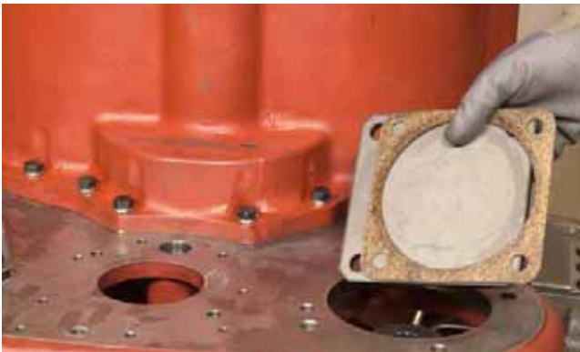
FIGURE 24: Remove pump drive blanking cover plate and gasket (if fitted).
