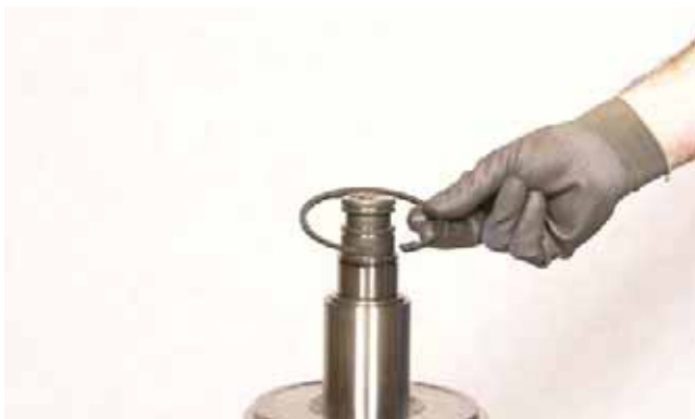
FIGURE 229: Install snap ring over shaft (to be used when installing drum/shaft in casing).
