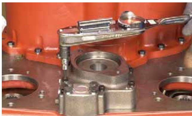
FIGURE 396: Install capscrews and tighten to specified torque. Refer to "TORQUE SPECIFICATIONS" on page 175.
