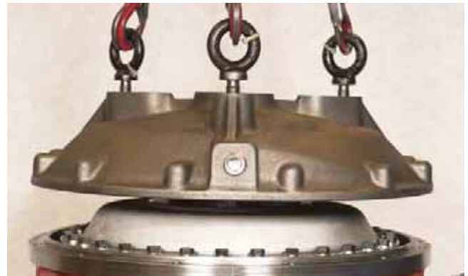
FIGURE 416: Install converter housing front cover with Loctite 515.
