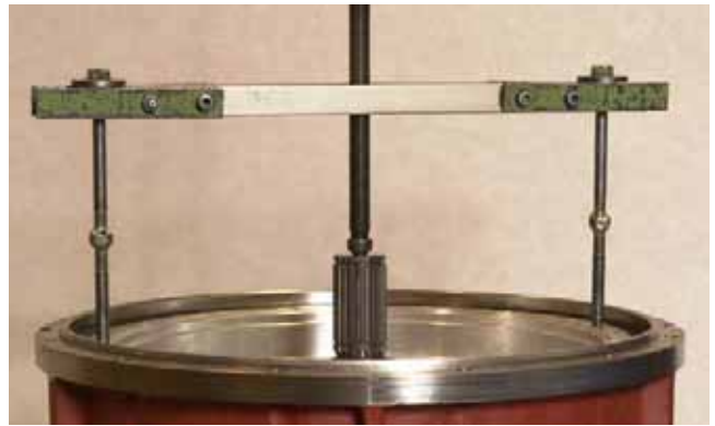
FIGURE 15: Use a standard bar-style puller to remove the impeller and oil baffle.
