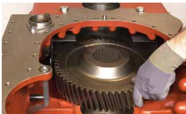
FIGURE 338: Position output gear in transmission case with long hub of gear to the rear side.
