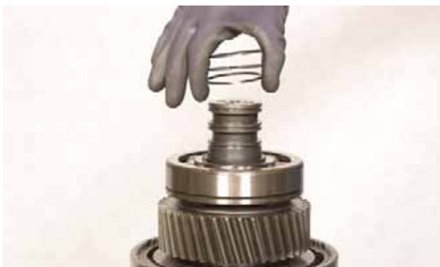
FIGURE 145: Install three (3) piston rings.
