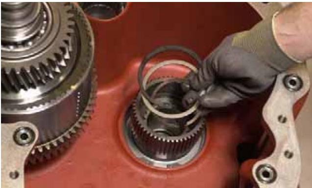
FIGURE 390: Install 2nd clutch hub snap ring, spacer, and snap ring.
