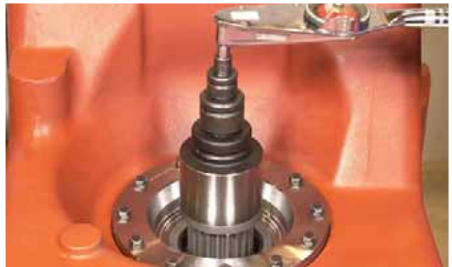
FIGURE 351: Tap and rotate output shaft to seat taper bearings. Loosen front bearing cap bolts. Using an torque wrench, determine the rolling torque of the output shaft and record. Tighten front bearing cap bolts to specified torque. Refer to "TORQUE SPECIFICATIONS" on page 175. Check rolling torque with bolts tight. Torque must be 4 - 10 lbs. in. (0.46 - 1.1 N•m) more than when bearing cap bolts were loose. Add or omit shims on the front bearing cap to achieve the proper preload.
