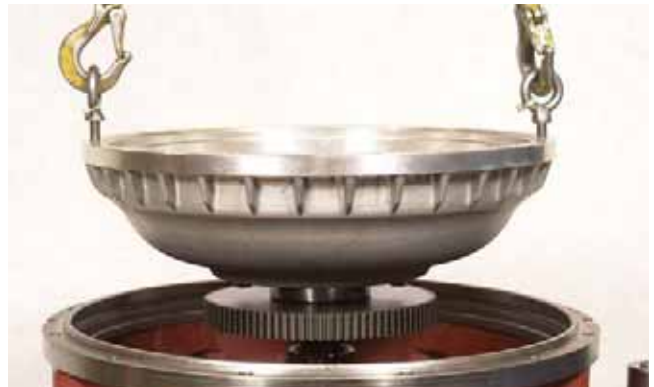
FIGURE 404: Install impeller assembly.
