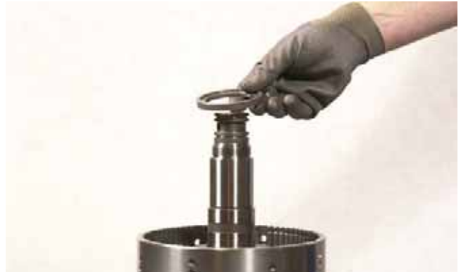
FIGURE 254: Install spring retainer, making sure it is fitted with stepped groove upward.
