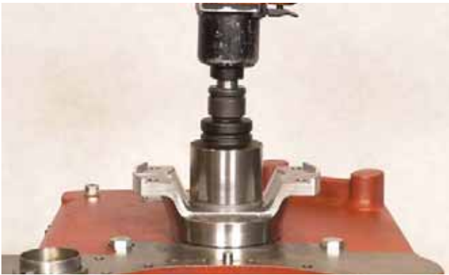
FIGURE 78: Using an impact wrench, loosen rear output flange nut.
