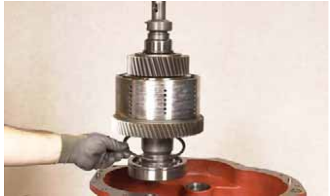
FIGURE 62: Forward drum assembly removed, showing snap ring and front bearing. Snap ring sits under gear and must be removed before forward drum assembly can be hoisted.
