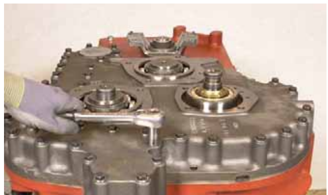
FIGURE 52: Remove transmission rear cover bolts.
