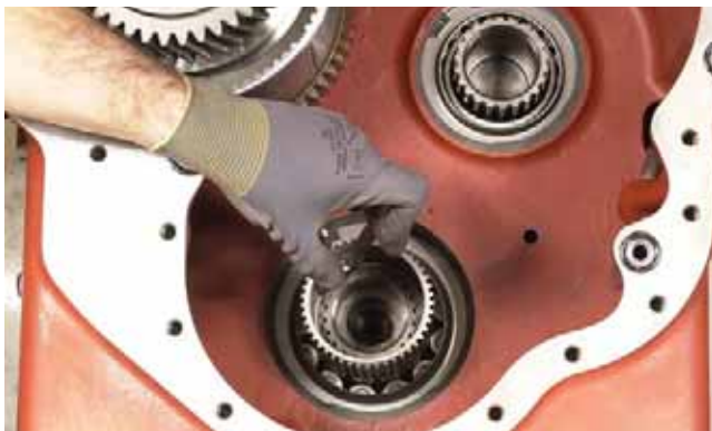
FIGURE 43: Remove snap ring from 4th clutch hub and remove hub.
