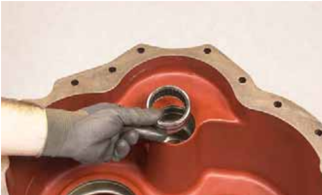
FIGURE 71: Remove turbine shaft bearings (2).
