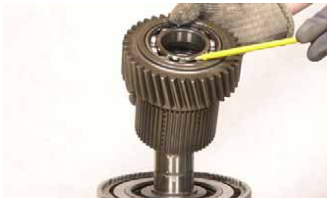
FIGURE 140: Install two (2) bearings in clutch gear and warm assembly to 248°F [120°C]. Install clutch gear and hub into clutch drum. Align splines on clutch hub with internal teeth of friction discs. Tap gear into position.
