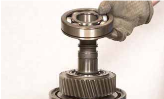
FIGURE 143: Warm outer bearing to 248°F [120°C] and install on shaft with groove down as shown.
