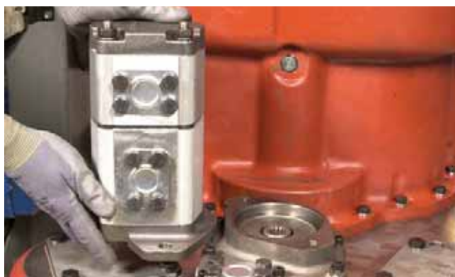
FIGURE 19: Remove pump manifold and o-ring.
