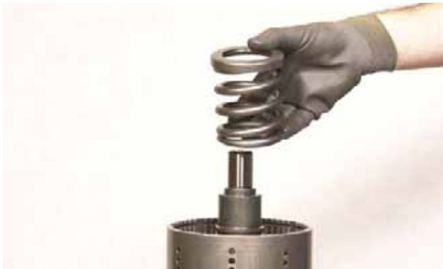
FIGURE 222: Install spring and spring retainer.
