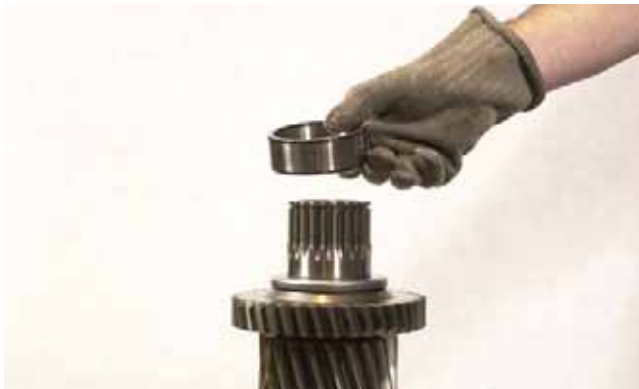
FIGURE 269: Warm bearing to 248°F [120°C] and install on shaft.
