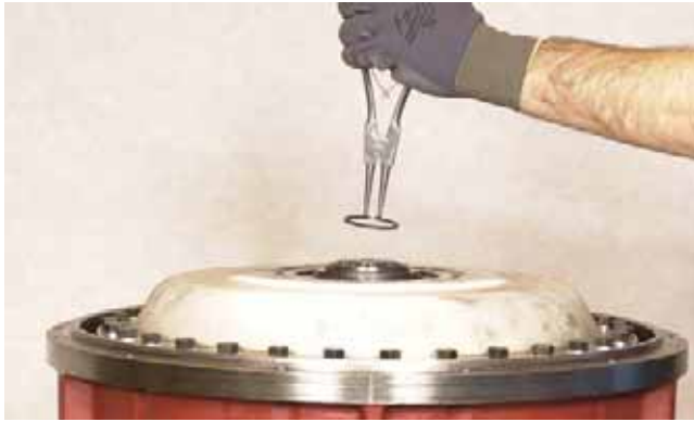
FIGURE 412: Install turbine snap ring.
