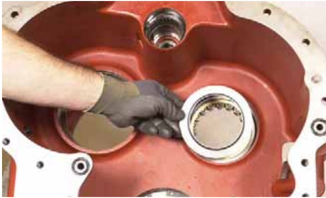
FIGURE 65: Remove 1st shaft drum assembly front bearing oil retainer.
