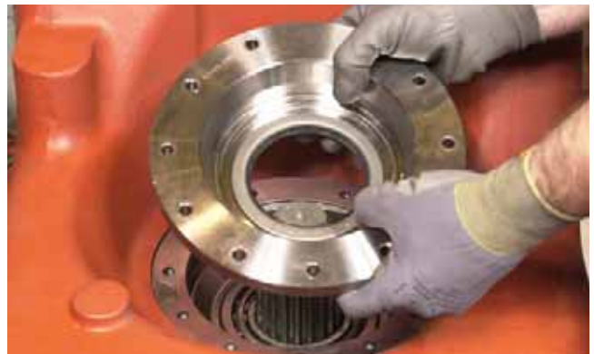
FIGURE 76: Remove front output cap and o-ring.
