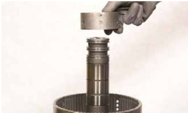
FIGURE 133: Install clutch piston spacer (wear sleeve).
