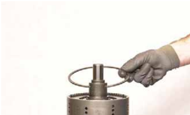
FIGURE 228: Install end plate snap ring.
