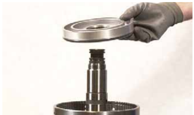
FIGURE 244: Remove clutch piston.
