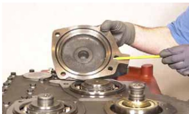
FIGURE 382: Fit o-ring (2) to idler shaft bearing cap and install bearing cap.
