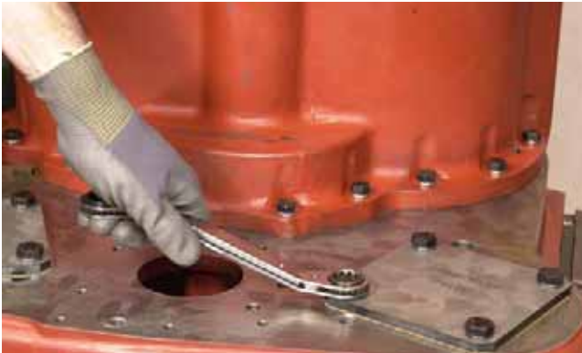
FIGURE 23: Remove pump drive blanking cover plate bolts (if fitted).
