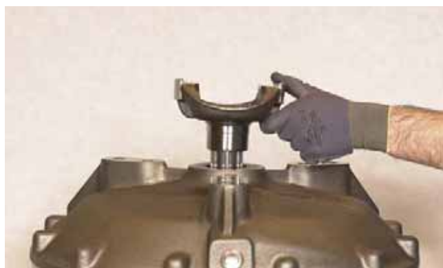
FIGURE 418: Install input flange.
