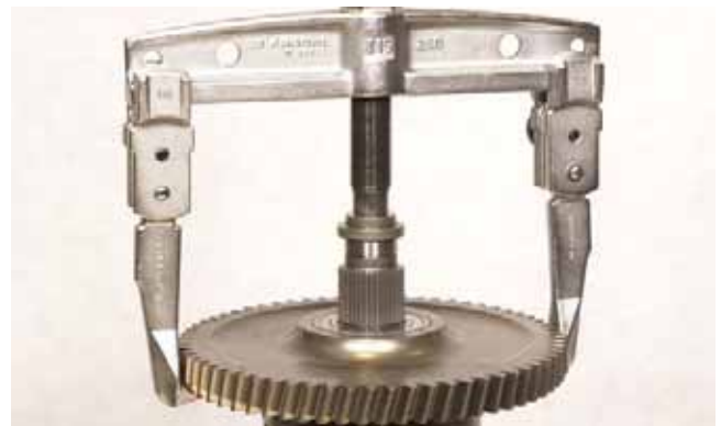
FIGURE 183: Remove 3rd clutch driven gear and bearing.
