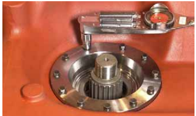
FIGURE 350: Tighten bearing cap bolts to specified torque. Refer to "TORQUE SPECIFICATIONS" on page 175.
