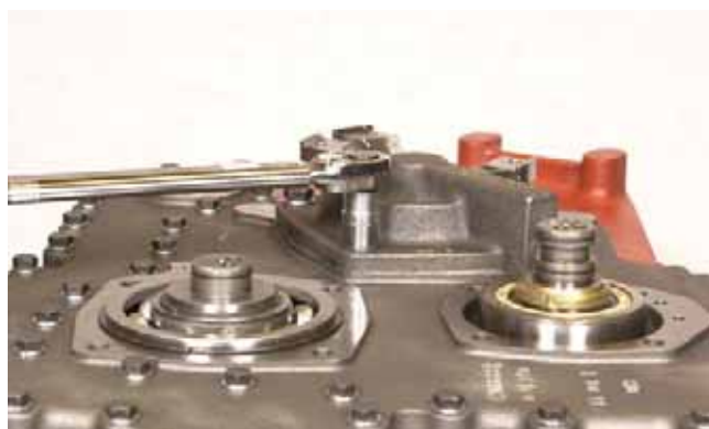
FIGURE 383: Install nuts and lockwashers to bearing cap and tighten to specified torque. Refer to "TORQUE SPECIFICATIONS" on page 175.
