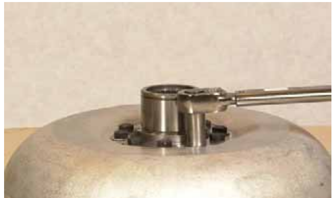
FIGURE 308: Align holes in turbine and turbine hub. Position locktabs and install screws. Tighten screws to specified torque. Refer to "TORQUE SPECIFICATIONS" on page 175. Bend a corner of the locktab over a flat of the screw heads. Refer to Figure 309.
