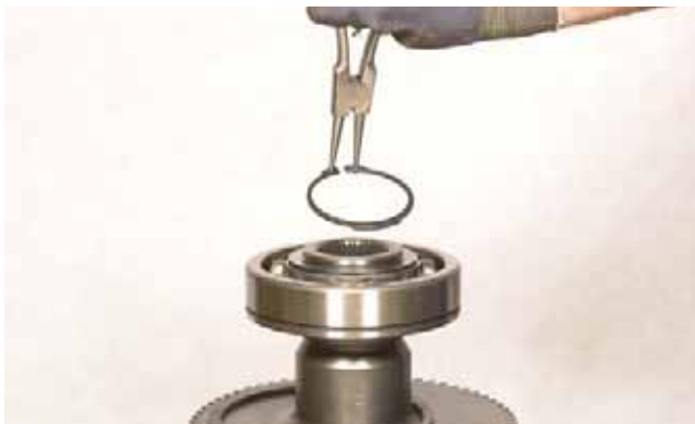
FIGURE 180: Install snap ring.
