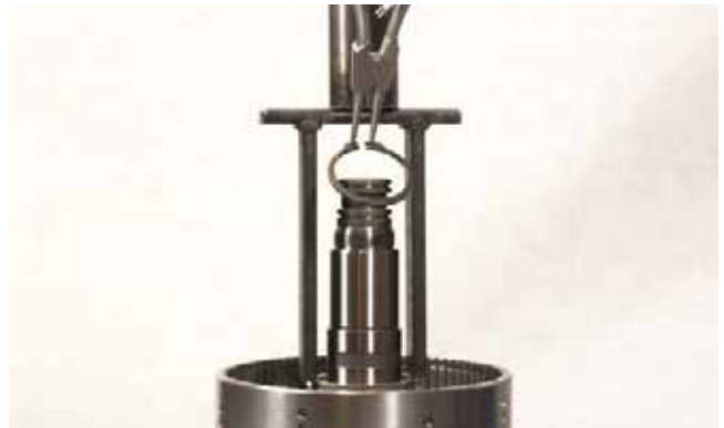
FIGURE 255: Compress return spring and install snap ring. Make sure retainer ring is in full position in groove.
