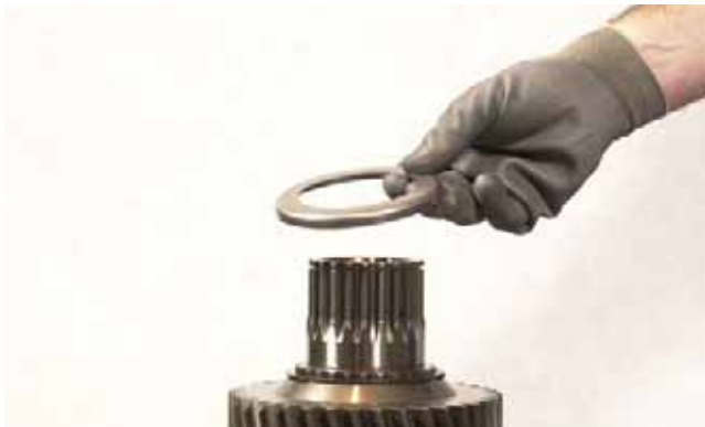
FIGURE 246: Remove bearing spacer.
