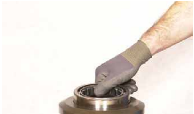
FIGURE 296: Install bearing to impeller hub.
