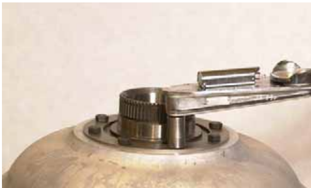
FIGURE 301: Make sure that hub mounting surface and tapped holes are cleaned with solvent. Install self-locking screws and tighten to 58–65 lbs ft. [79–87 N•m].
