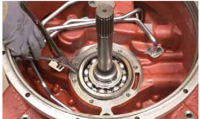
FIGURE 98: Remove turbine shaft bearing snap ring.
