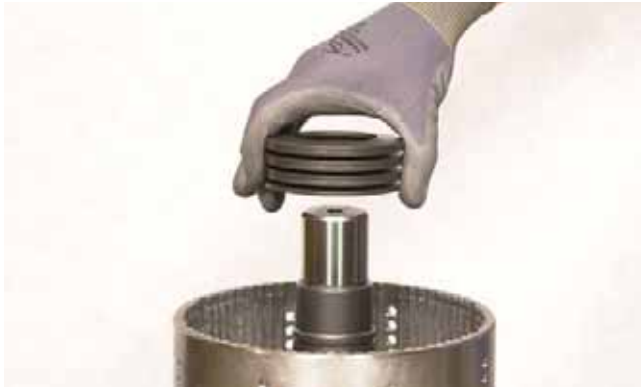
FIGURE 119: Remove Belleville washers.
