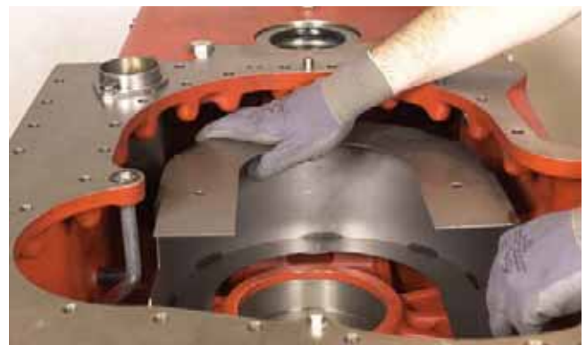
FIGURE 88: Remove oil baffle.
