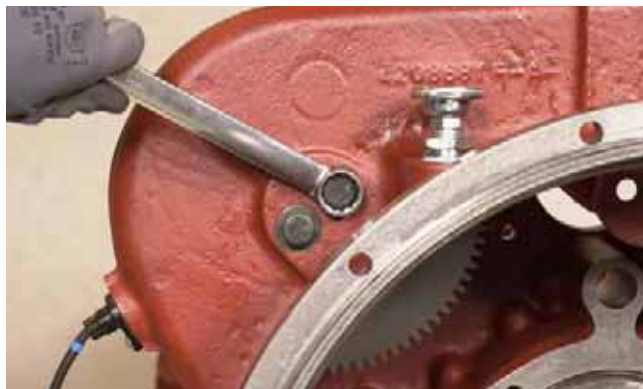
FIGURE 29: Remove pump drive gear bolts.
