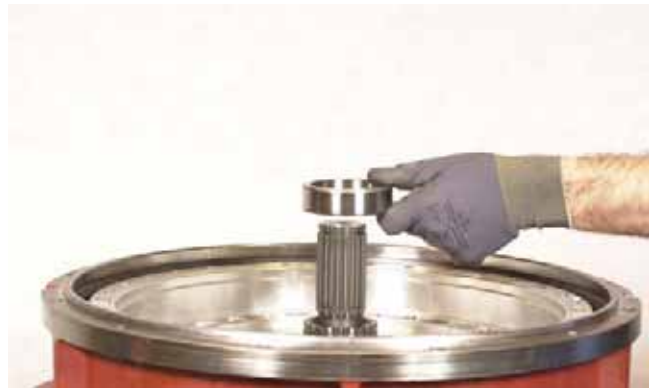
FIGURE 405: Install impeller hub bearing inner race.
