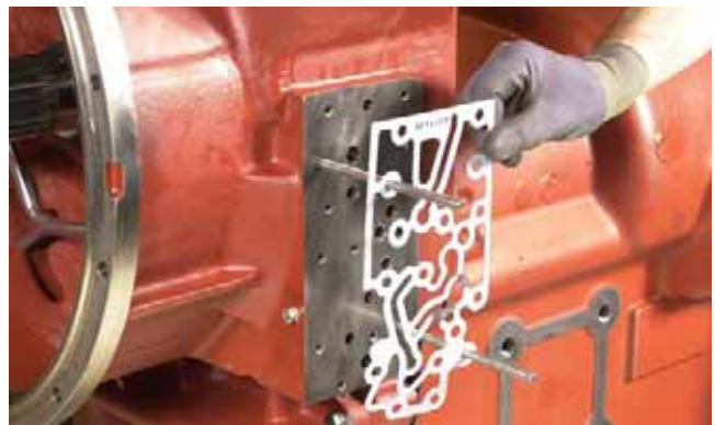
FIGURE 393: Install aligning studs and install new valve gasket.
