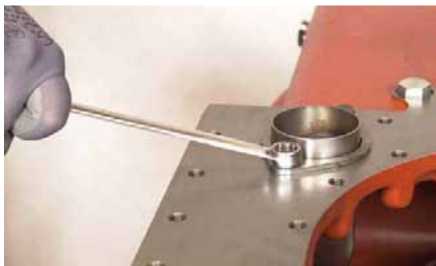
FIGURE 92: Remove suction tube bolts (2).
