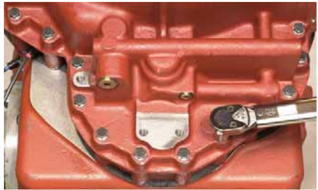
FIGURE 392: Install alignment studs and position converter housing assembly onto studs. Install converter-housing-to-transmission-housing bolts and lockwashers and tighten to specified torque. Refer to "TORQUE SPECIFICATIONS" on page 175.
