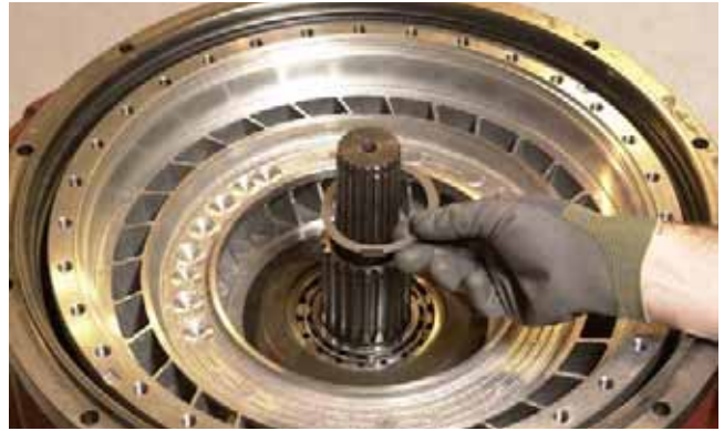
FIGURE 14: Remove reaction member spacer.
