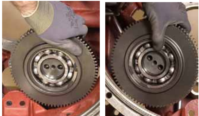
FIGURE 320: Install left and right outer auxiliary pump drive gear assemblies. Put new o-rings (4) on bolts, install bolts, and tighten to specified torque. Refer to "TORQUE SPECIFICATIONS" on page 175.
