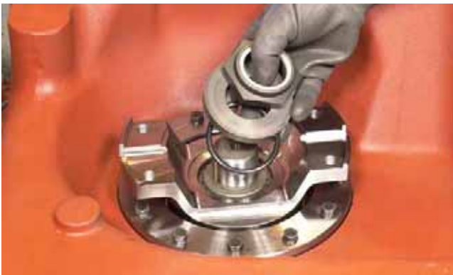
FIGURE 73: Remove front output flange nut, washer, and o-ring.
