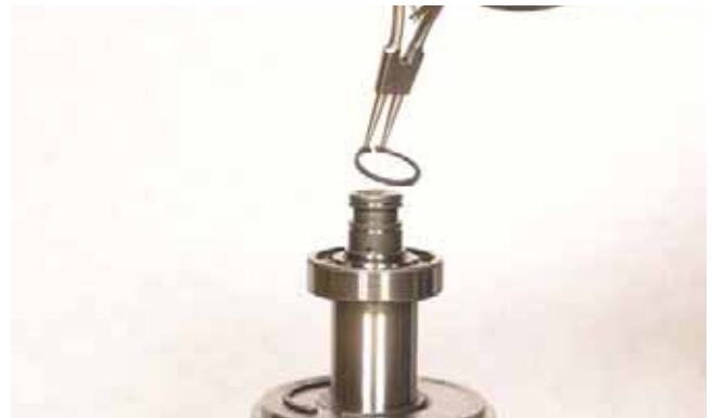
FIGURE 231: Install bearing snap ring.
