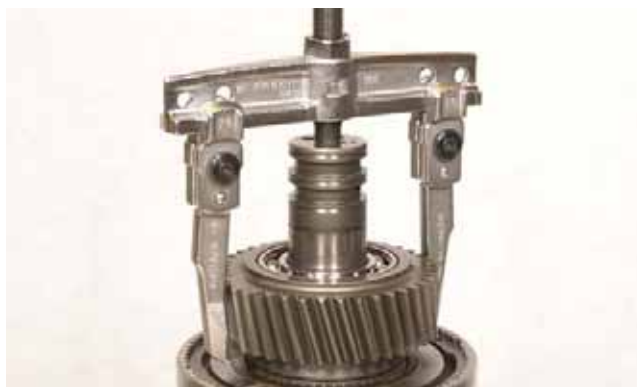
FIGURE 106: Remove clutch gear and outer bearing as an assembly.
