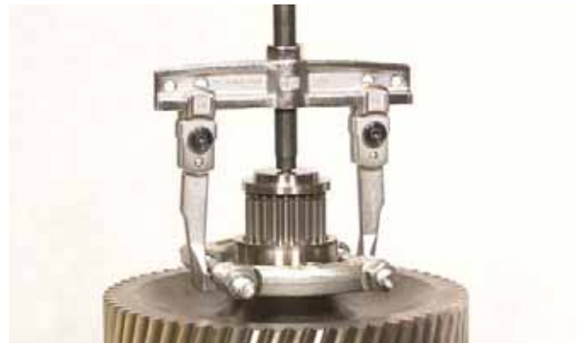
FIGURE 274: Turn shaft and, using a puller, remove bearing inner race from shaft.
