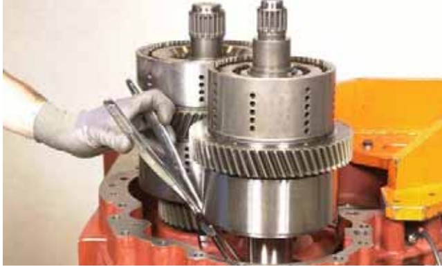
FIGURE 95: Remove 4th drum shaft assembly snap ring.
