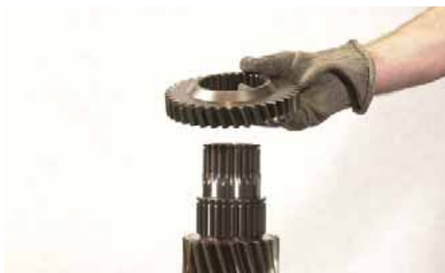
FIGURE 266: Turn shaft and install gear.
