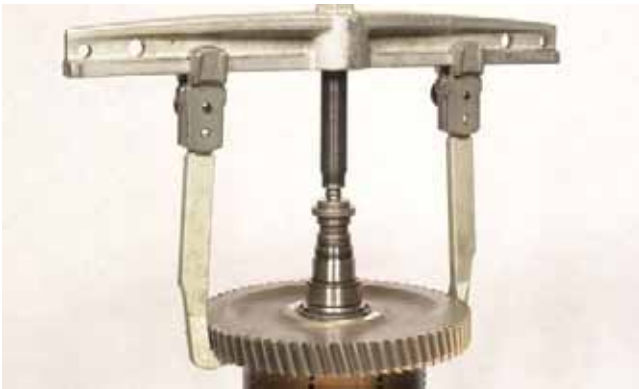
FIGURE 234: Using a puller, remove gear, bearing outer race, and spacer as an assembly.
