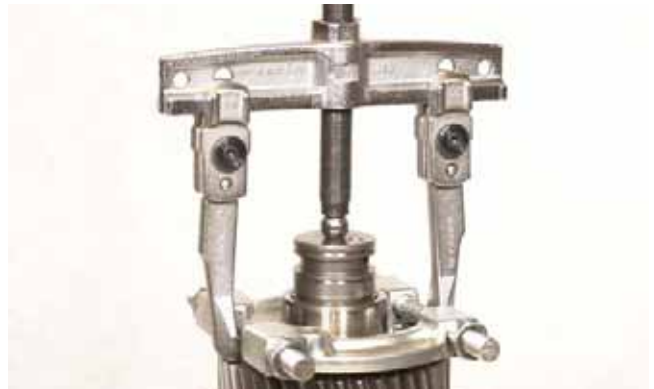
FIGURE 152: Remove bearing inner race.
