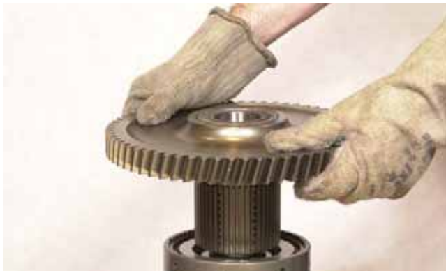
FIGURE 204: Install gear and bearing into clutch drum by warming the assembly to 248°F [120°C]. Align splines on clutch hub with internal teeth of friction discs. Tap gear into position.
