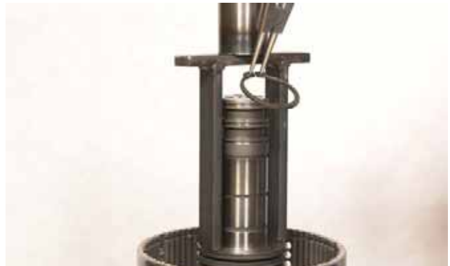
FIGURE 136: Compress spring and install snap ring, making sure ring is in full position in groove.
