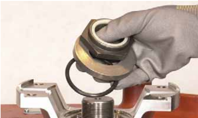
FIGURE 79: Remove rear output flange nut, washer, and o-ring.
