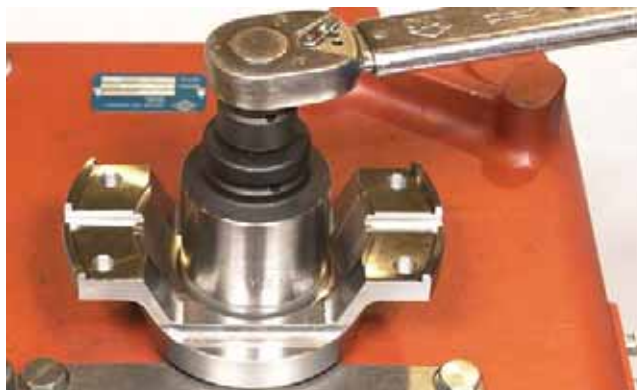
FIGURE 357: Tighten rear output flange nut to 250 - 300 lbs. ft. (339 - 407 N•m).
