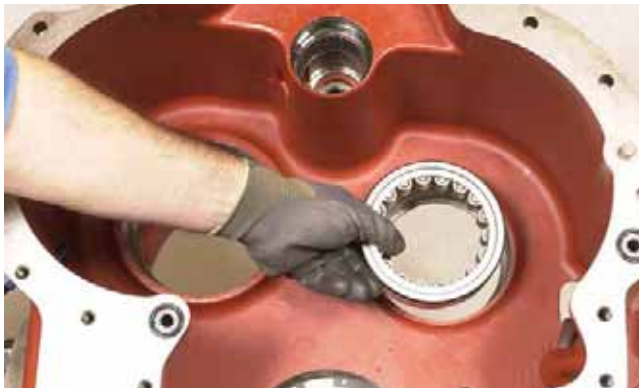
FIGURE 66: Remove 1st shaft drum assembly front bearing.
