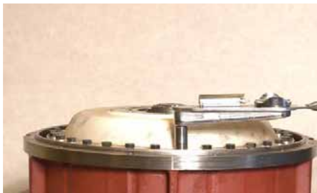
FIGURE 411: Install impeller cover screws and lockwashers and tighten to specified torque. Refer to "TORQUE SPECIFICATIONS" on page 175.
