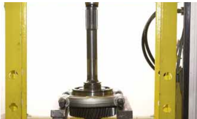
FIGURE 283: Using a hydraulic press, remove bearing.
