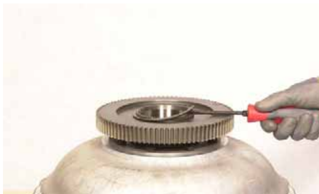
FIGURE 288: Remove impeller hub gear snap ring.
