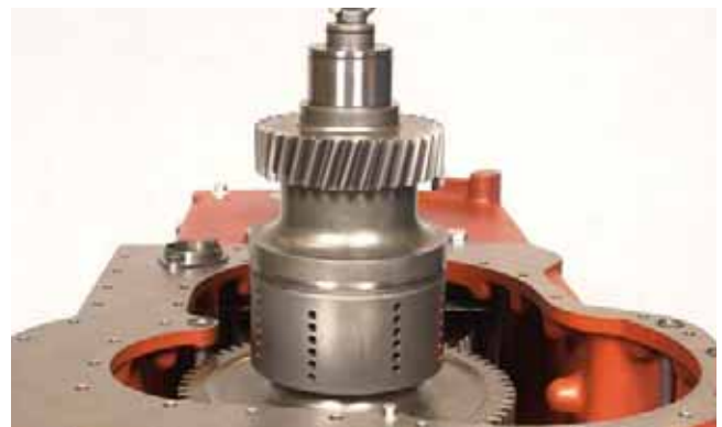
FIGURE 369: Install 3rd clutch assembly.
