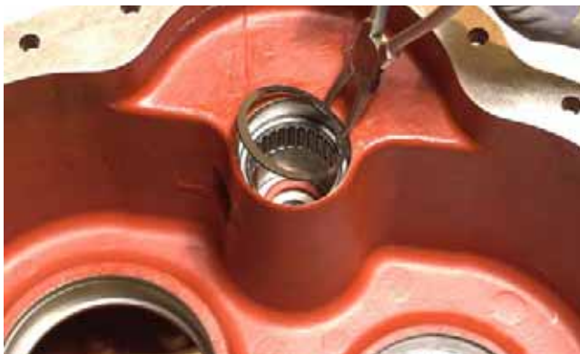
FIGURE 365: Install turbine shaft needle roller bearing snapring.
