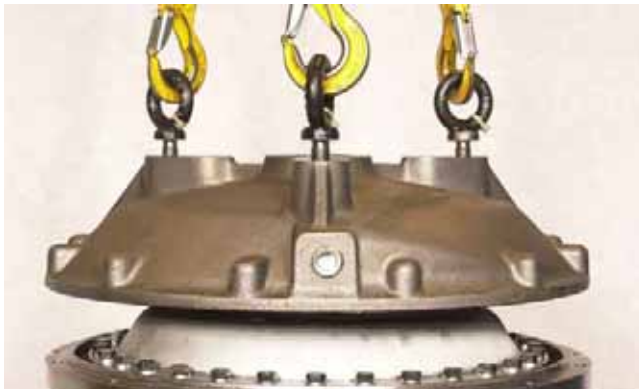
FIGURE 5: Remove converter housing front cover with three (3) standard eye bolts 3/4 UNC attached to a chain.
