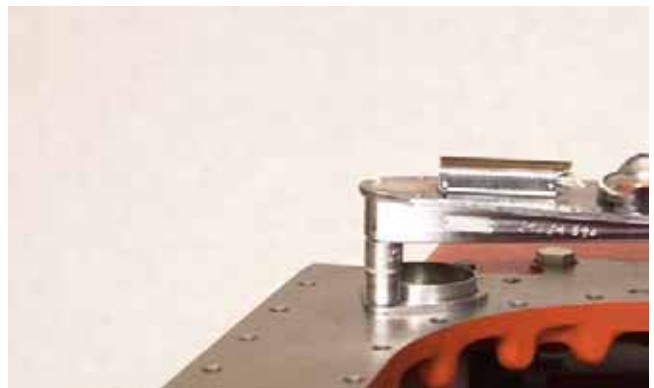
FIGURE 333: Install suction tube capscrews and lockwashers and tighten to specified torque. Refer to "TORQUE SPECIFICATIONS" on page 175.
