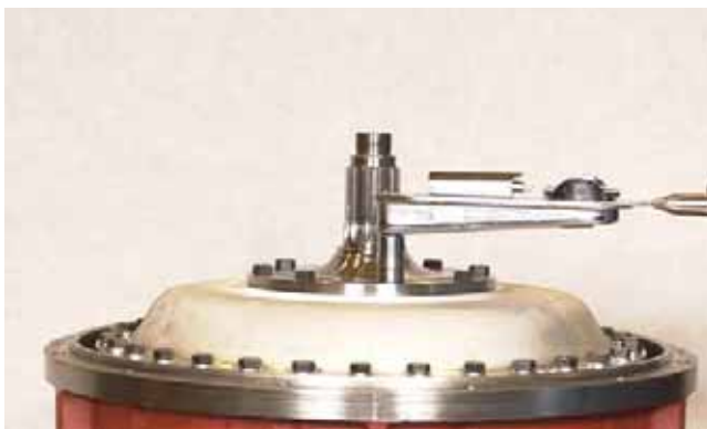
FIGURE 414: Install bolts and tighten to specified torque. Refer to "TORQUE SPECIFICATIONS" on page 175.
