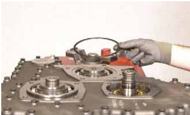
FIGURE 377: Raise idler shaft slightly and install snap ring.
