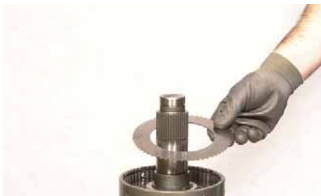
FIGURE 200: Install clutch outer half disc (friction material on one side) with steel side up.
