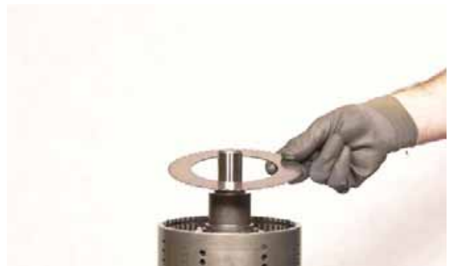
FIGURE 226: Install one (1) clutch outer half disc (friction material on one side) steel side up.
