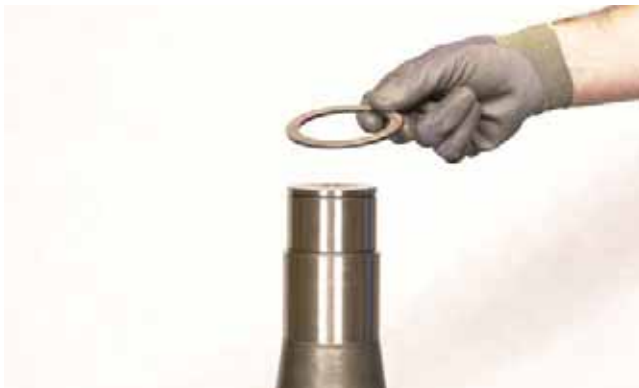
FIGURE 276: Turn shaft and install idler shaft rear bearing spacer.
