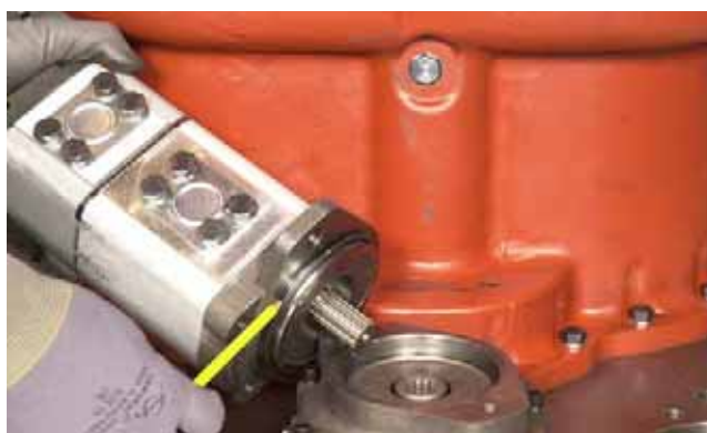
FIGURE 398: With new o-ring in place, install hydraulic pump assembly.
