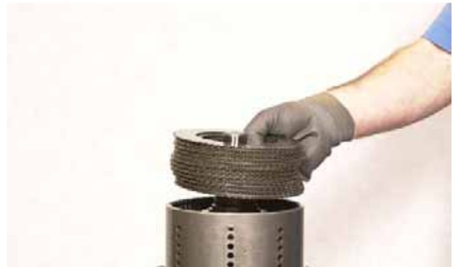
FIGURE 214: Remove clutch inner and outer discs.
