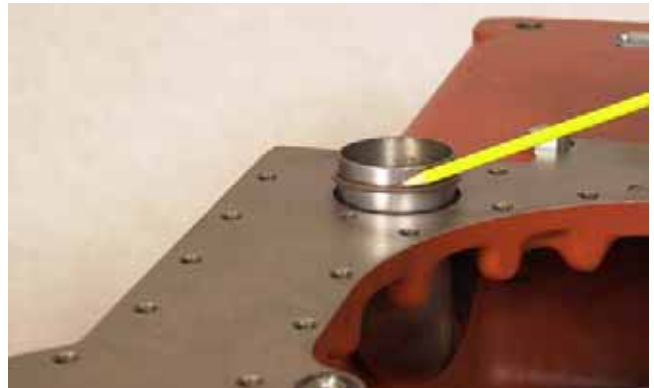
FIGURE 331: Install suction tube and o-ring into transmission case.
