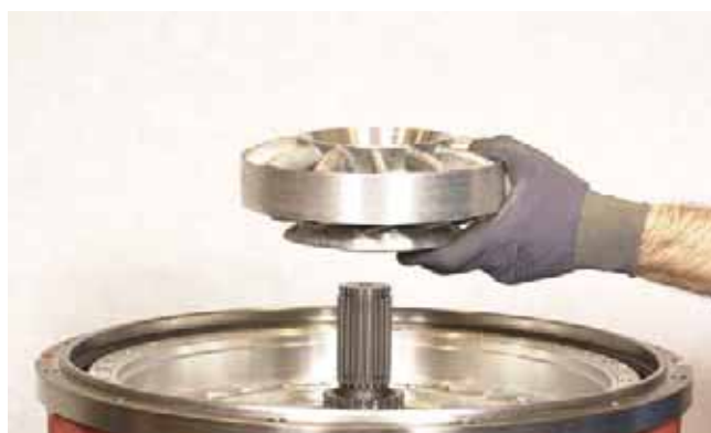
FIGURE 407: Install reaction member with thin side of blades inward to impeller.
