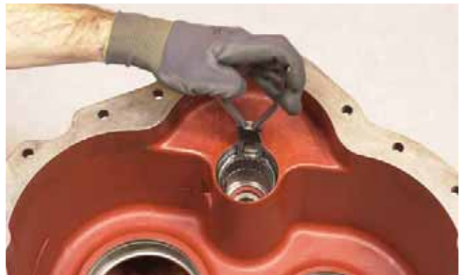
FIGURE 70: Remove turbine shaft bearing snap ring.
