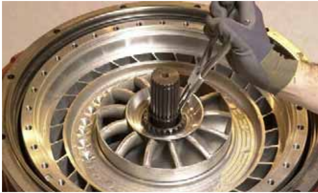
FIGURE 11: Remove locating ring from turbine shaft.
