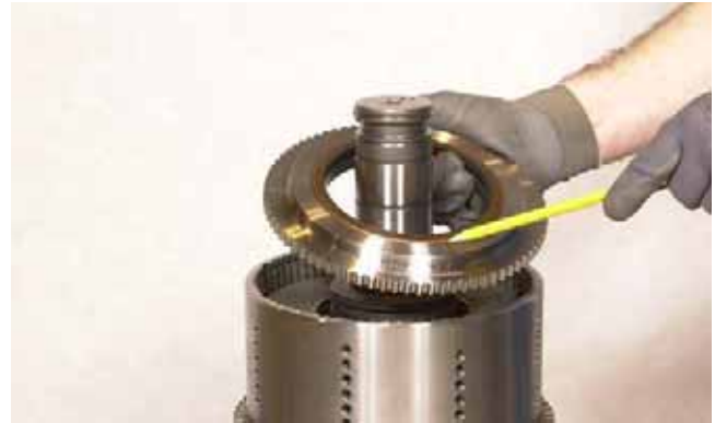
FIGURE 170: Install new seal in end plate and install plate.
