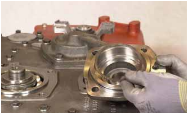
FIGURE 48: Remove 1st clutch shaft rear bearing cap o-rings and spring disc.
