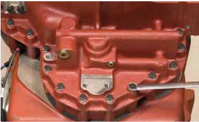
FIGURE 36: Remove converter-housing-to-transmission-case bolts and washers.
