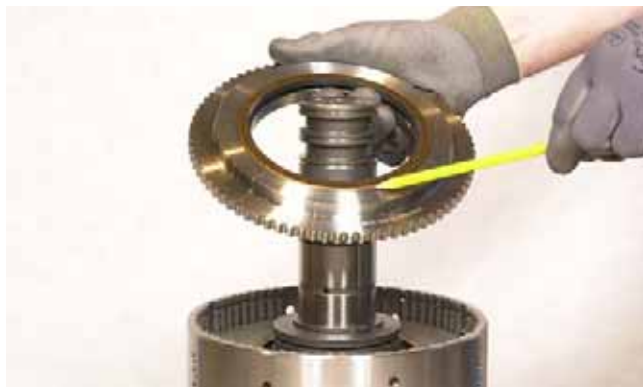
FIGURE 138: Install new seal in end plate.
