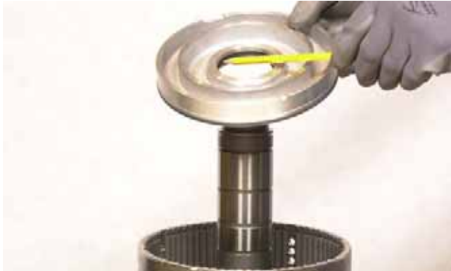
FIGURE 131: Install clutch piston inner seal. Size as described in Figure 106.
