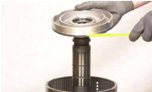
FIGURE 132: Install clutch piston outer seal.
