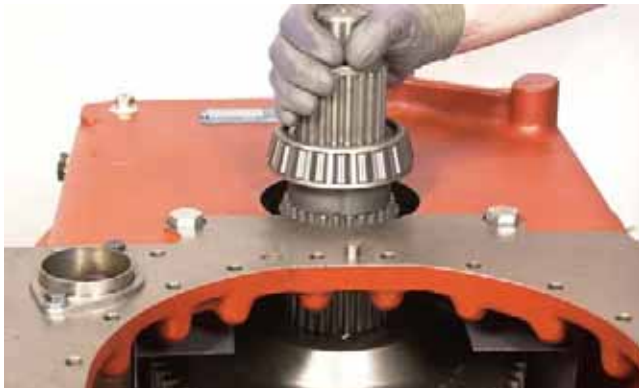
FIGURE 341: Insert output shaft and taper bearing from rear of case and through output gear.
