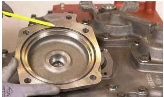
FIGURE 45: Remove 3rd clutch shaft rear bearing cap and o-ring.
