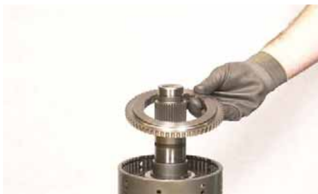
FIGURE 201: Install end plate.
