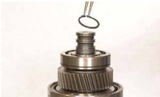
FIGURE 144: Install bearing snap ring.
