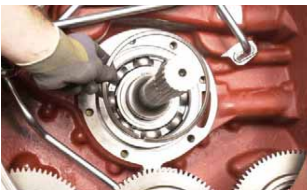
FIGURE 324: From the front of the housing, install turbine shaft bearing snap ring. Tap shaft until snap ring is in full position in groove.
