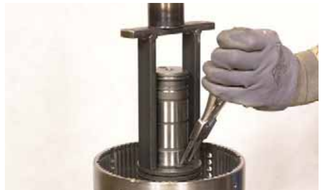
FIGURE 159: Compress return spring and remove snap ring.
