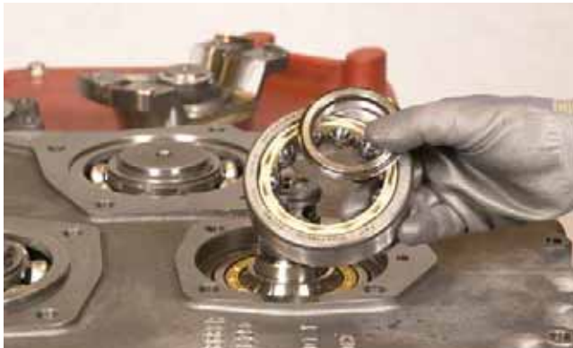
FIGURE 55: Remove bearing inner and outer race.
