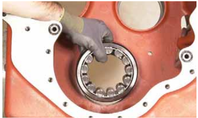
FIGURE 69: Remove idler shaft front bearing.
