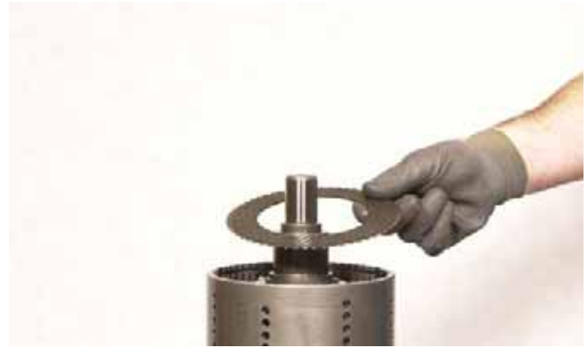
FIGURE 224: Install one (1) clutch outer half disc (friction material on one side) steel side down.
