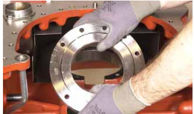
FIGURE 86: Remove inside front cap.
