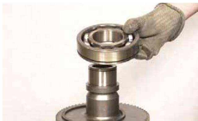
FIGURE 178: Warm bearing to 248°F [120°C] and install on shaft with groove down as shown.
