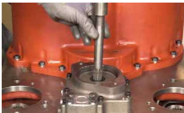
FIGURE 397: Install pump drive shaft.
