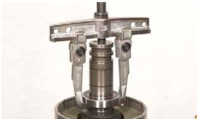
FIGURE 109: Remove clutch gear inner bearing.
