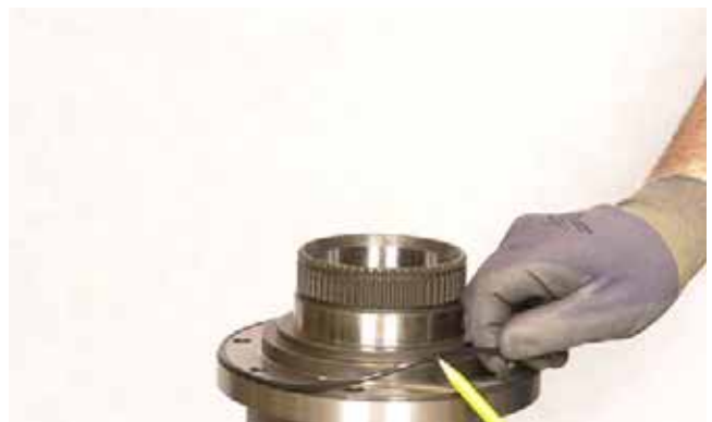
FIGURE 298: Position new impeller hub o-ring on hub.
