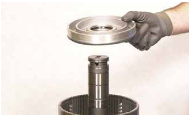
FIGURE 162: Remove clutch piston.
