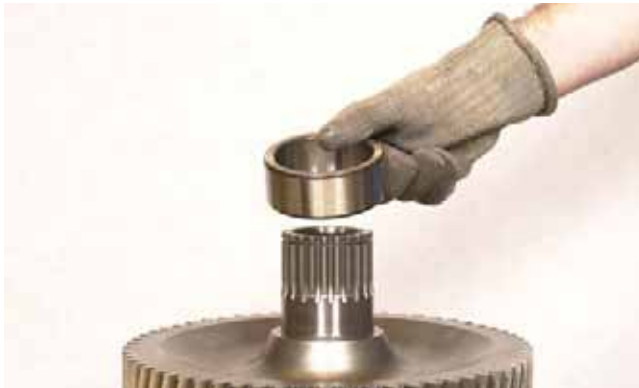
FIGURE 275: Warm bearing inner race to 248°F [120°C] and install on shaft.
