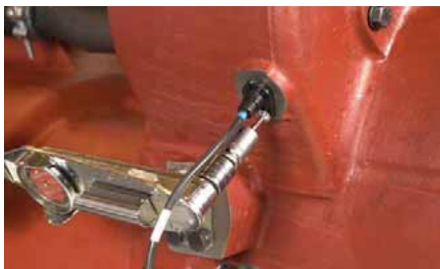
FIGURE 421: Install speed sensors (3).
