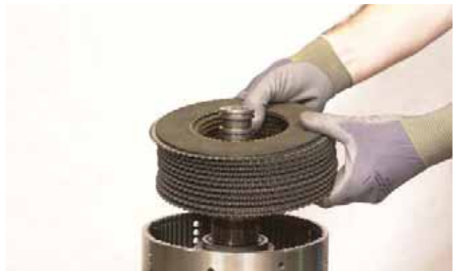
FIGURE 256: Install one (1) steel disc. Alternate steel and friction discs until proper number of discs are installed.
