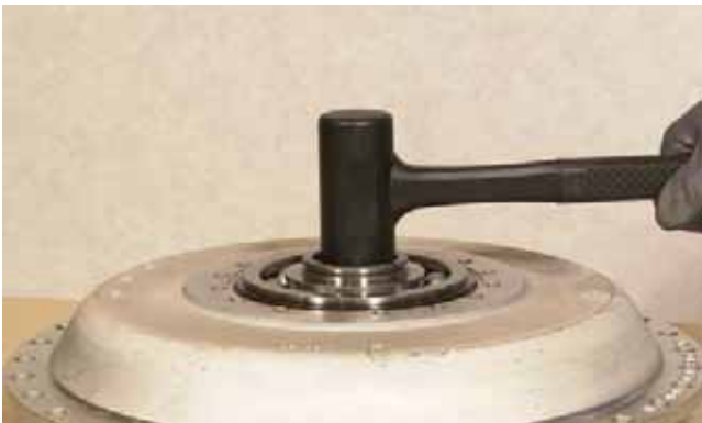
FIGURE 306: Tap turbine hub from impeller cover.
