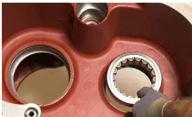
FIGURE 361: Install 1st clutch shaft bearing.
