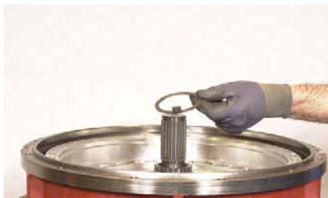
FIGURE 406: Install reaction member spacer.
