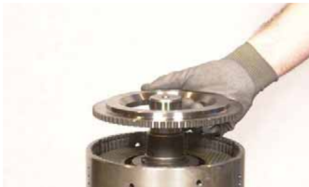
FIGURE 129: Install end plate.
