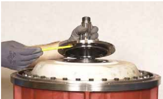
FIGURE 413: Install input shaft support with new o-ring.
