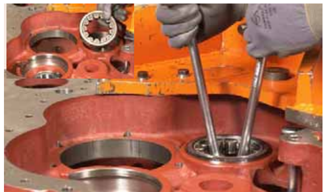
FIGURE 99: Using a soft hammer, tap turbine shaft and bearing assembly from converter housing.
