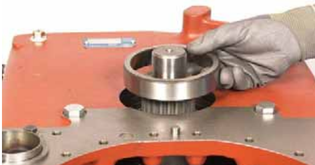
FIGURE 342: Install bearing cup.
