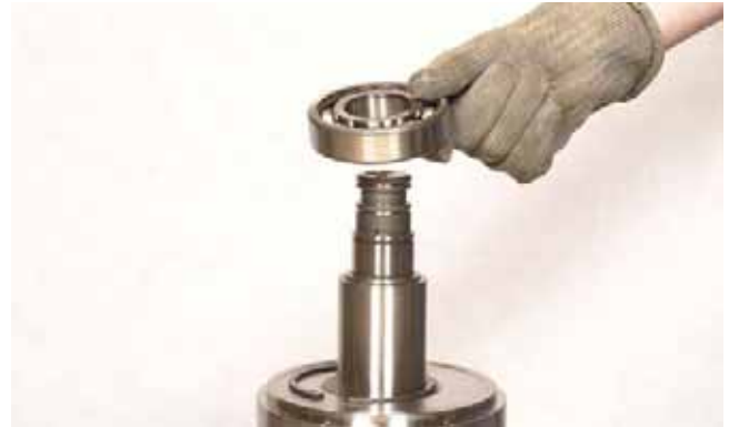
FIGURE 230: Warm bearing to 248°F [120°C] and install on shaft.
