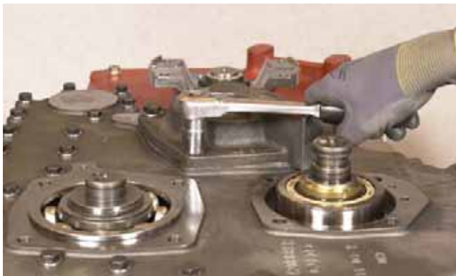
FIGURE 49: Remove nuts from idler bearing cover assembly.
