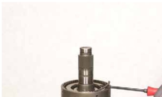
FIGURE 185: Remove end plate snap ring.
