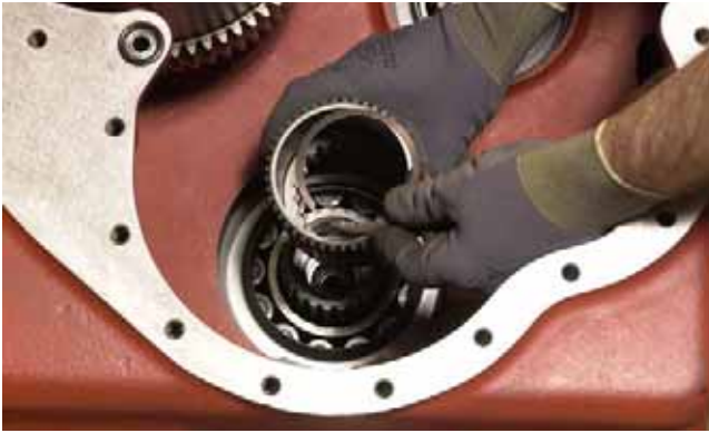
FIGURE 388: Install 4th clutch hub and snap ring.
