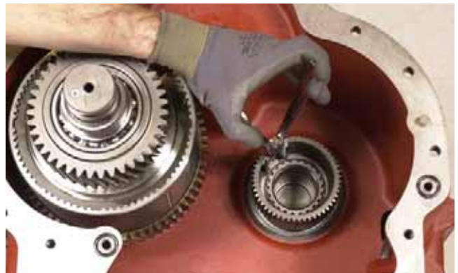
FIGURE 39: Remove snap ring from 2nd clutch hub (driven gear).
