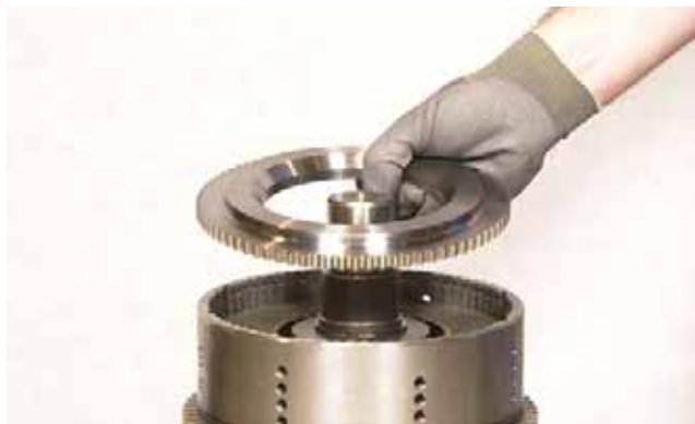
FIGURE 116: Remove 2nd clutch end plate.
