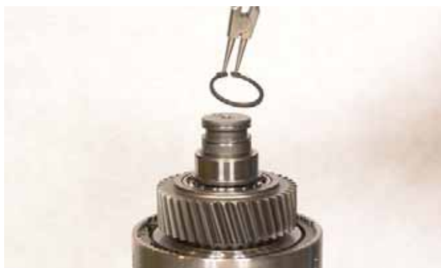
FIGURE 175: Install bearing snap ring.
