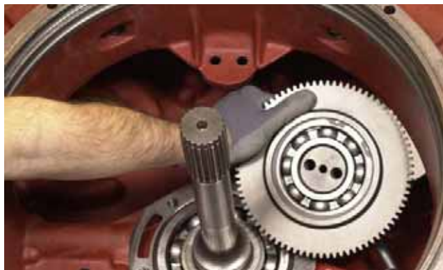
FIGURE 32: Remove pump drive.
