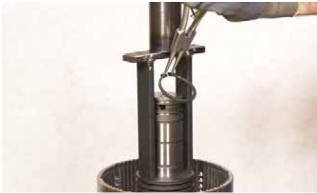
FIGURE 168: Compress spring and install snap ring.
