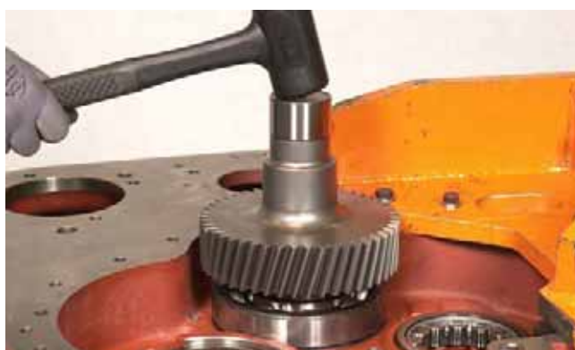
FIGURE 323: From the rear of the housing, tap turbine shaft and bearing in converter housing. Tap shaft until gear shoulders are against converter housing.
