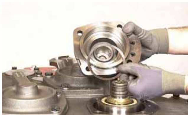
FIGURE 386: Install 1st shaft bearing cap with new o-rings (3) and spring disc.
