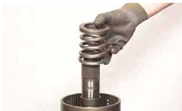
FIGURE 189: Remove spring and spring retainer.
