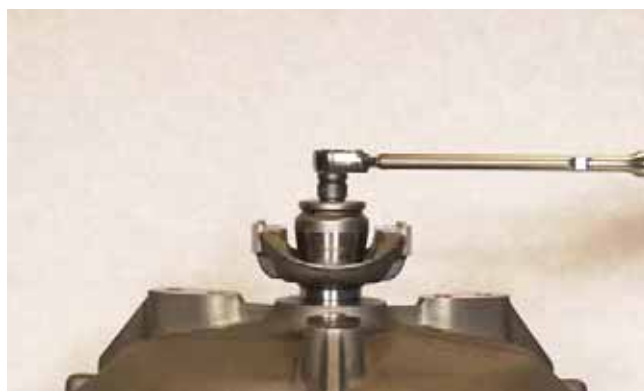
FIGURE 420: Tighten nut to specified torque. Refer to "TORQUE SPECIFICATIONS" on page 175.
