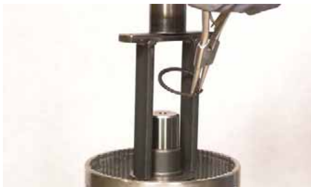
FIGURE 127: Compress spring and install snap ring, making sure ring is in full position in groove.
