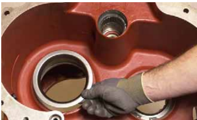
FIGURE 366: Install forward shaft bearing oil retainer. Refer to Figure 367.
