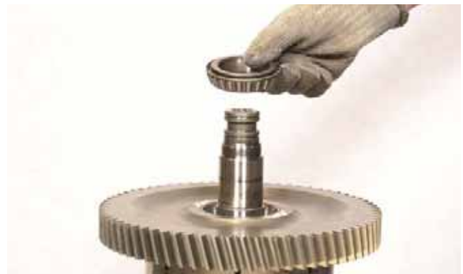
FIGURE 262: Warm taper bearing to 248°F [120°C].
