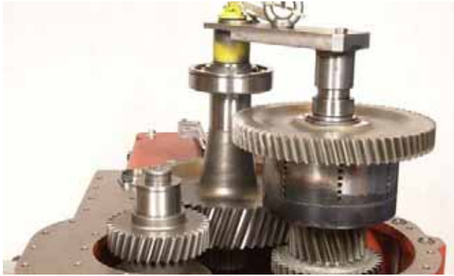
FIGURE 370: Using special tool “Idler & Low Shaft Lifting Hook” (see page 178), install idler shaft and 1st clutch assembly.
