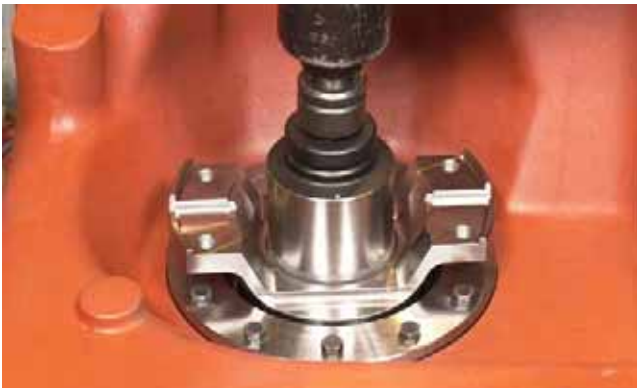
FIGURE 72: Using an impact wrench, remove front output flange nut.
