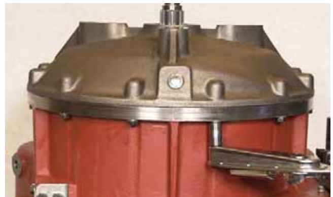
FIGURE 417: Install bolts and washers and tighten to specified torque. Refer to "TORQUE SPECIFICATIONS" on page 175.
