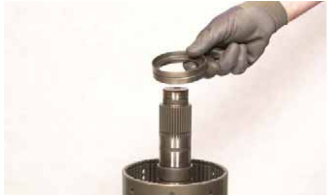
FIGURE 194: Install clutch piston spacer.
