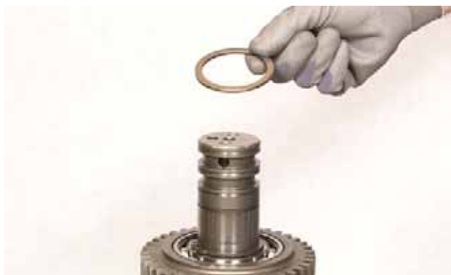
FIGURE 104: Remove bearing thrust washer.
