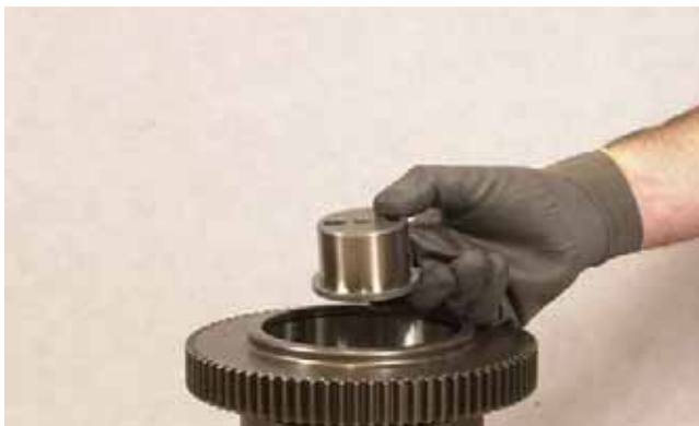
FIGURE 317: Remove bearing support.
