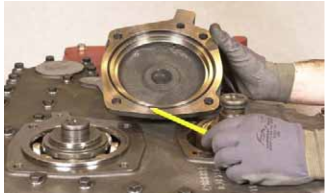
FIGURE 50: Remove idler bearing cover assembly and o-ring.
