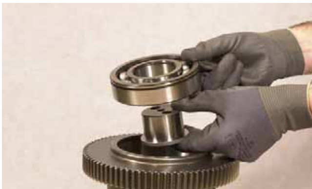
FIGURE 318: Press bearing support into bearing and install assembly into gear.
