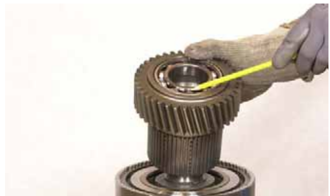
FIGURE 172: Install two (2) bearings in clutch gear and warm assembly to 248°F [120°C]. Install clutch gear and hub into clutch drum. Align splines on clutch hub with internal teeth of friction discs. Tap gear into position.
