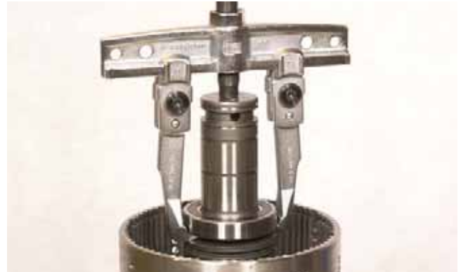
FIGURE 158: Remove inner bearing.
