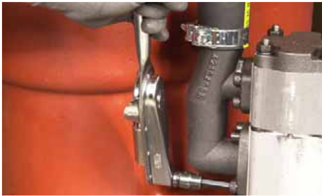
FIGURE 401: Install capscrews and lockwashers and tighten to specified torque. Refer to "TORQUE SPECIFICATIONS" on page 175.
