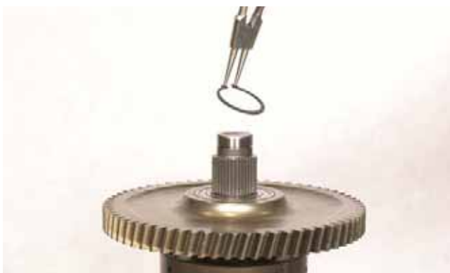
FIGURE 205: Install snap ring.
