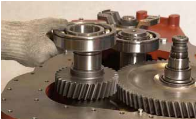
FIGURE 371: Warm 3rd shaft bearing to 248°F [120°C] and install on shaft with snap ring groove up as shown.
