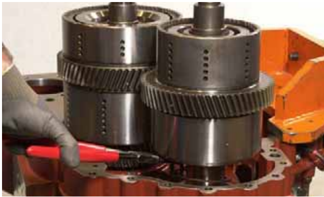
FIGURE 329: Install 4th shaft and drum assembly snap ring.
