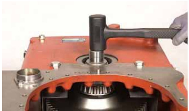
FIGURE 82: Push output shaft through bearing and gear from the rear side.
