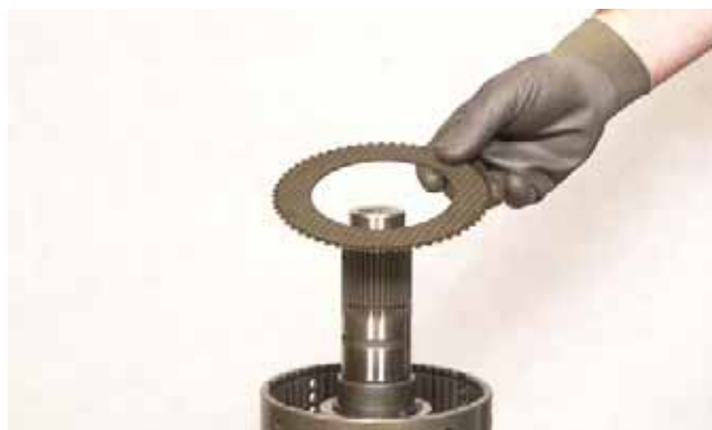
FIGURE 198: Install clutch outer half disc (friction material on one side) with steel side down.
