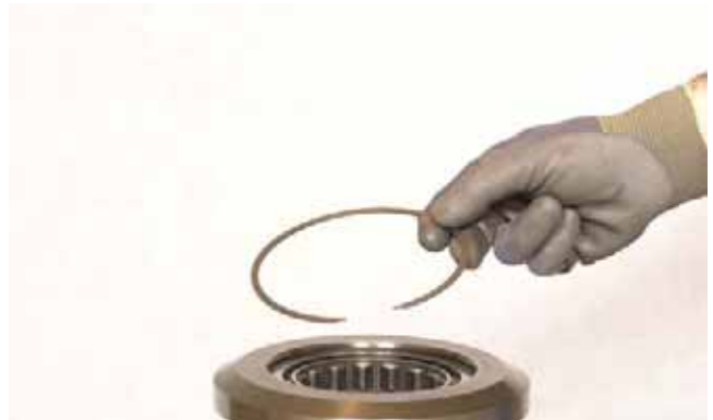
FIGURE 297: Install impeller hub bearing snap ring.
