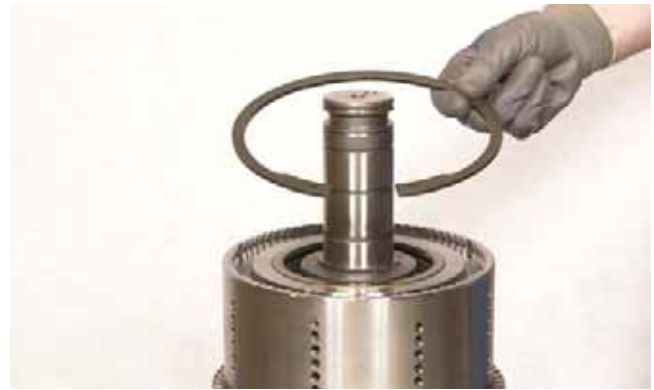
FIGURE 171: Install end plate snap ring.
