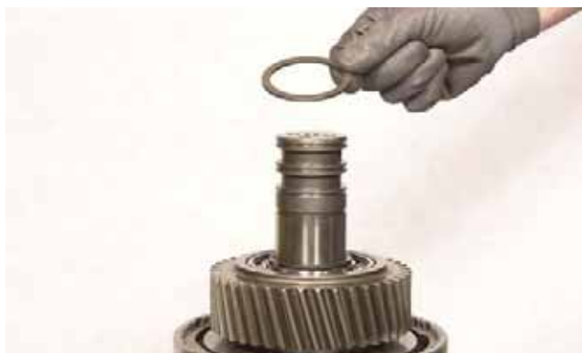
FIGURE 142: Install outer bearing thrust washer.
