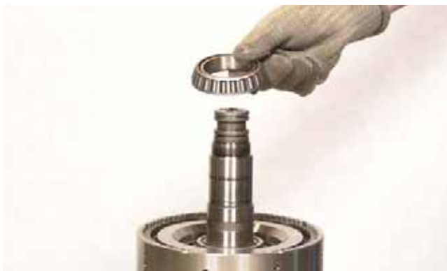
FIGURE 259: Warm taper bearing to 248°F [120°C] and install on shaft.
