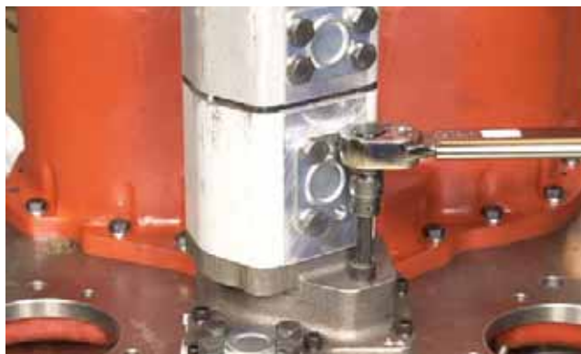
FIGURE 399: Install hydraulic pump capscrews and lockwashers and tighten to specified torque. Refer to "TORQUE SPECIFICATIONS" on page 175.
