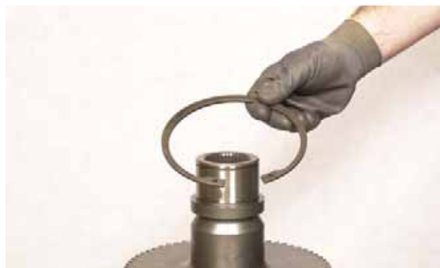
FIGURE 177: Install snap ring over shaft before fitting bearing.
