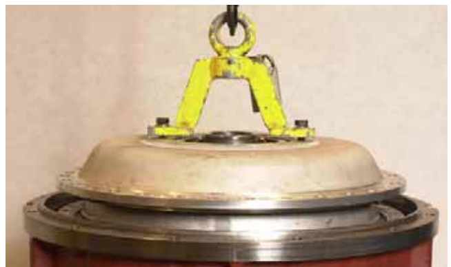
FIGURE 10: Use special tool to lift impeller cover assembly. (See “Impeller Cover Lifting Hook”, on page 179.)
