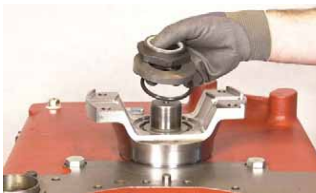
FIGURE 356: Install o-ring, spacer, and nut.
