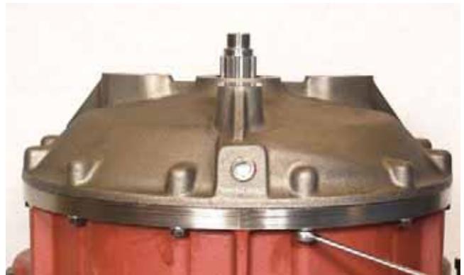
FIGURE 4: Remove bolts and washers securing front cover to converter housing.
