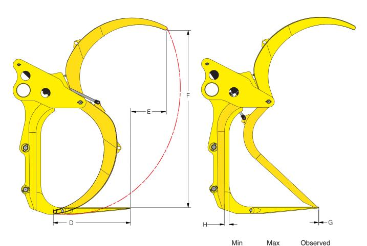
Min Max Tine Tip to HD Tip, Horizontal, HD Closed (D): 38" 48" 60 Tine Tip to HD Tip, Horizontal, HD Open (E): 74" 84" 61 Tine Tip to HD Tip, Vertical, HD Open (F): 185" 209" 62 0" KO Arm Tip to End of Tine (G): 6" 63 -1" KO Arm to Carriage Face (H): 0" 64
