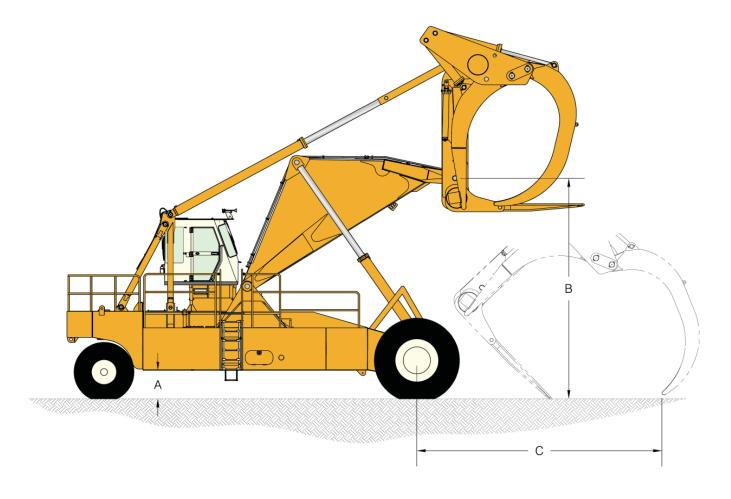
Ground Clearance, Chassis (measure from rear of chassis lower flange) (A) :
