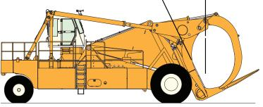
Carriage Angle from Vertical - Hoist Fully Extended, Tilt Fully Retracted (X) Carriage Angle from Vertical - Hoist Fully Extended, Tilt Fully Extended (Y) Carriage Angle from Vertical - Hoist Fully Retracted, Tilt Fully Retracted (Z)
