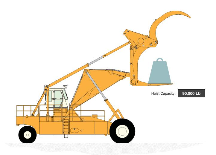
Verify that the machine can hoist the rated load.
