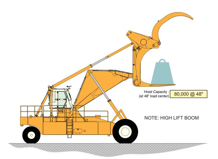
Verify that the machine can hoist the rated load.
