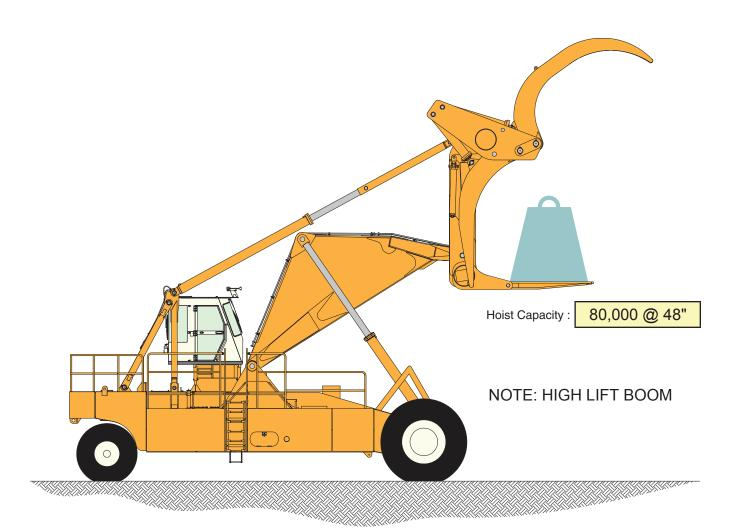
Verify that the machine can hoist the load.
