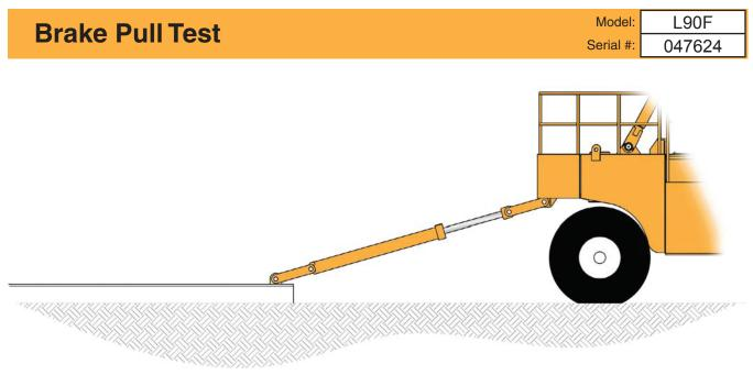
Install pressure gauge on stem port.
